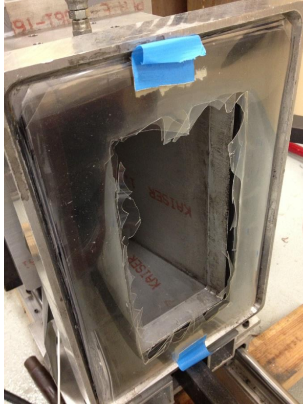
Figure 63. Acetate membrane rupture after blast.
