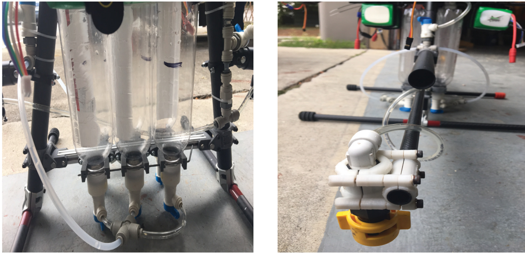
Figure 4.3: Sprayer assembly (a) Spray Tank (b) Spray Applicator
