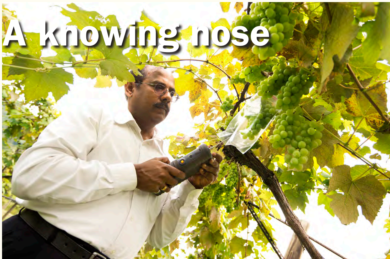
Kumar Mallikarjunan conducts research using the Cyranose 320 to detect chemical vapors in the air surrounding fruit by preprogramming pattern-sensing algorithms to recognize vapors of interest.
