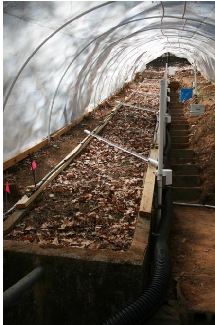
Report 3/Figure 2 (above). The physical soil model after installation of all the physical infrastructure (greenhouse shelter; plumbing, irrigation, and electrical lines) and instruments (soil moisture and temperature probes; input and output tipping buckets; lysimeters; and meteorological station). Photo courtesy of Ray Lee.
