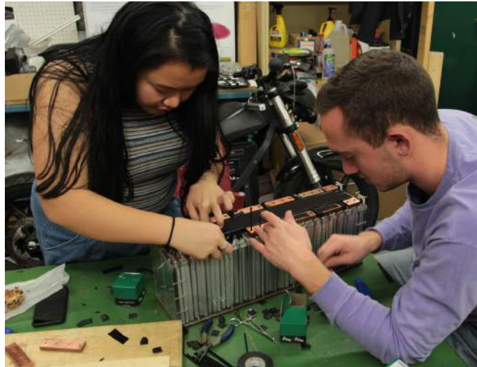
Cecilia Reyes (left) and Frank D'Amico (right) install the bus bars onto one of BOLT III's battery boxes. These bars conduct electricity and act as a switchboard for the electric vehicle
