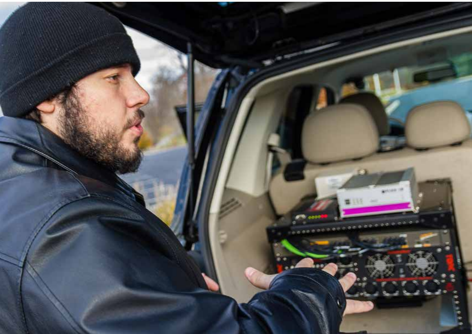
Adam Shoemaker, a member of the Autonomous Car Team, gestures toward the autonomous vehicle's main computers. They are the heart of any successful autonomous vehicle, and must allow the car to understand its environment by integrating data from all its sensors and plan the vehicle's path accordingly.
