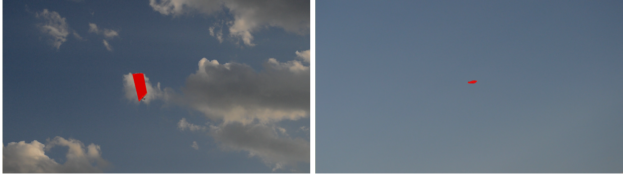
Figure 2.12: False detection by the edge of the clouds (left) feature points occlusion (right)
