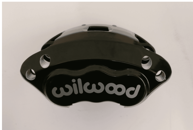
Figure 5.5: Procured brake caliper model 120-11873 by Wilwood Disc Brakes.
