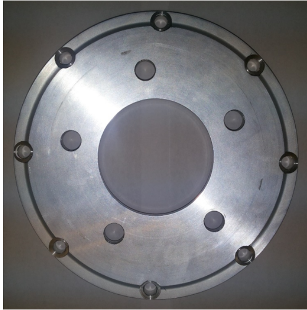
Figure 5.7: Customized Brake Rotor Hat
