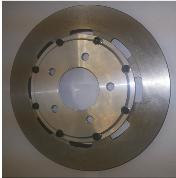
Figure 5.8: Assembly of brake rotor and rotor hat. Reprinted Figure 13 from [16] with permission from ASME publications.
