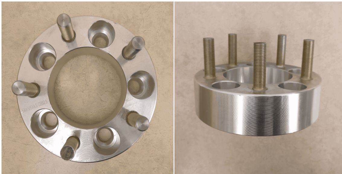
Figure 5.10: Wheel Spacer with new studs installed. Reprinted Figure 14 from [16] with permission from ASME publications.
