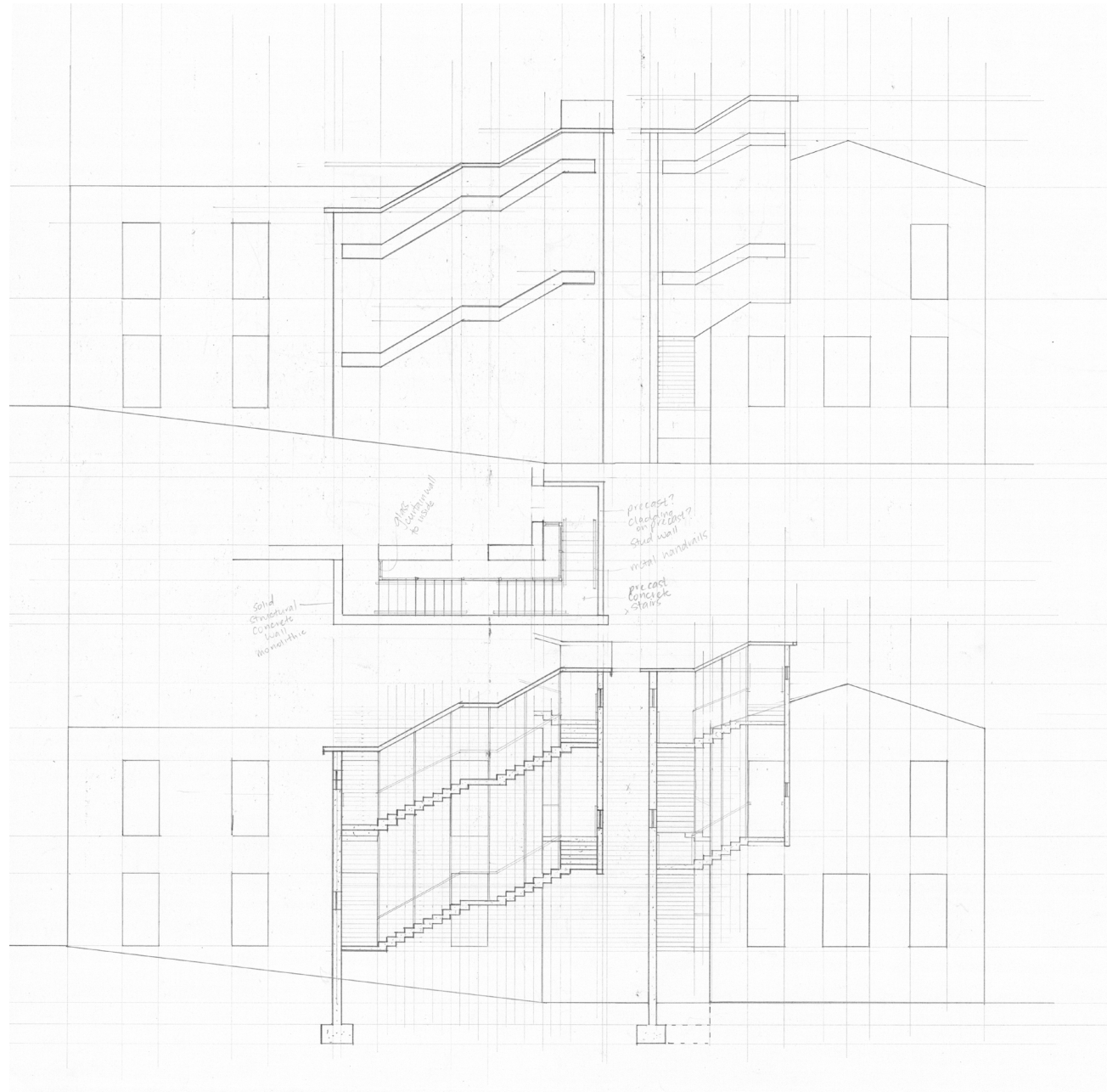
Stair Variations: Steretomic stair study (left) utilizing a single concrete wall for structure. Tectonic stair study (right) utilizing a steel structural system similar to interior frame.
