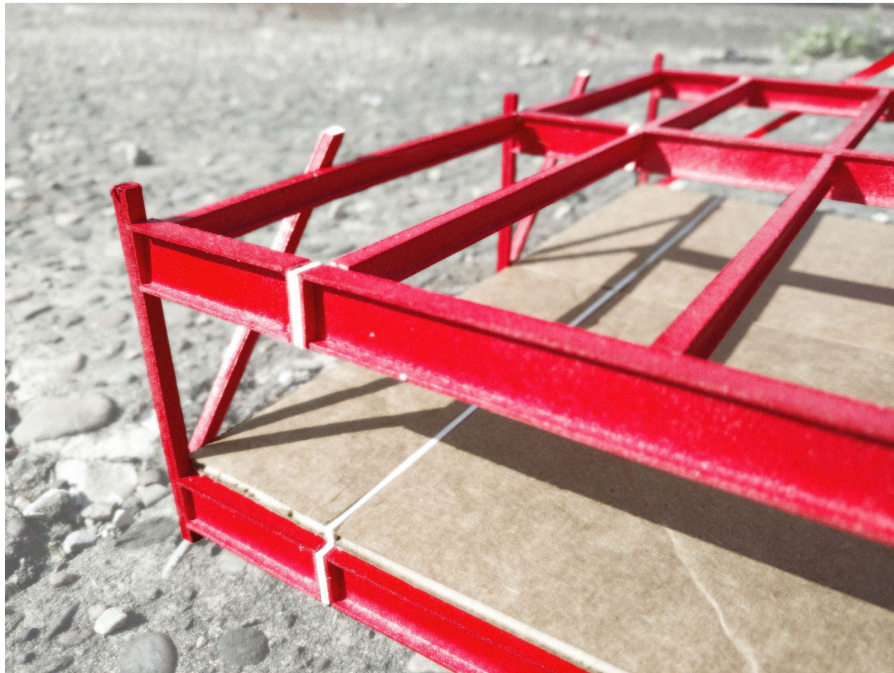
thermal breaks at the balcony edge
