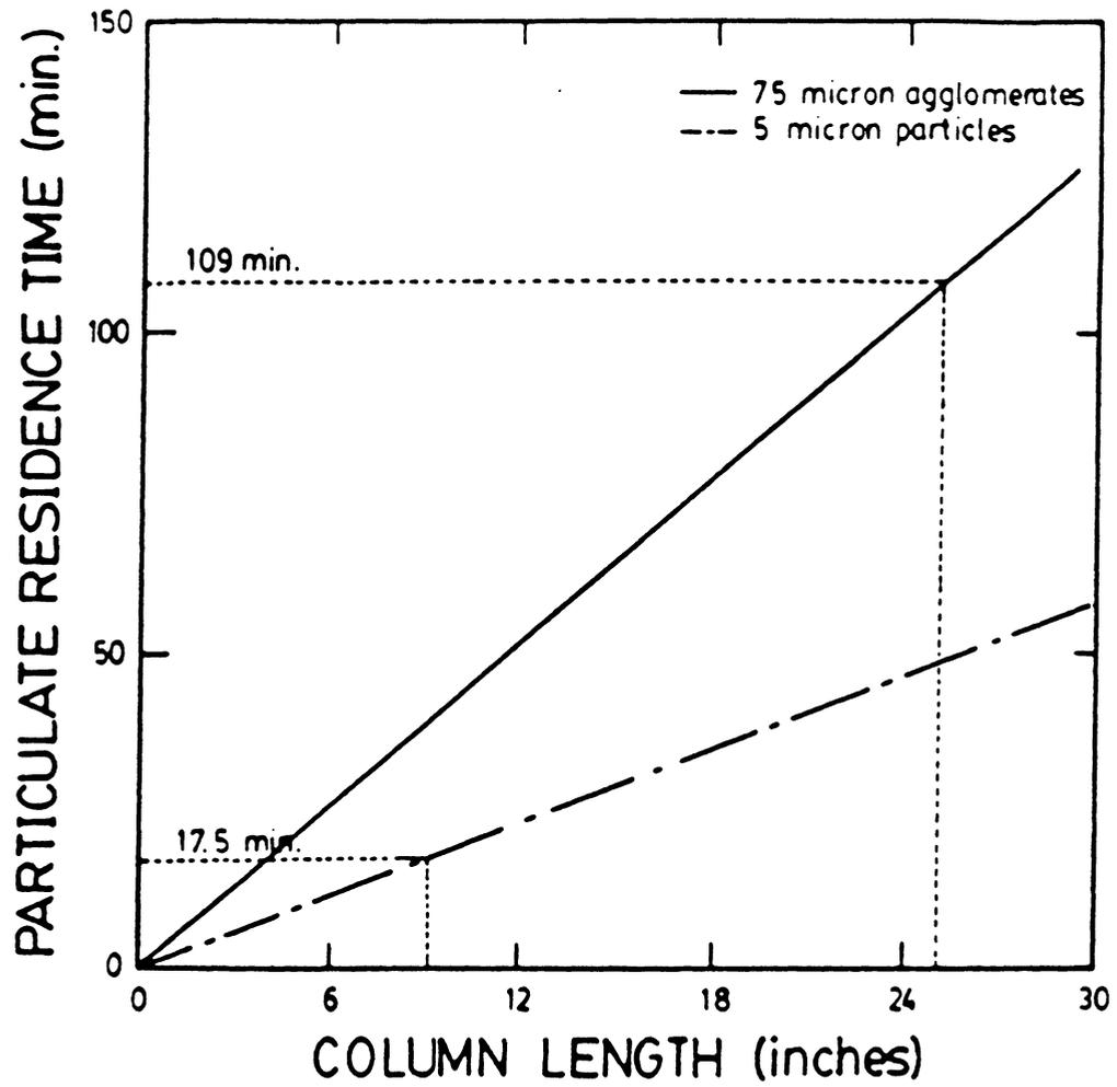
Figure 4.13 Particulate residence time versus column length for 75 micron agglomerates and 5 micron particles
