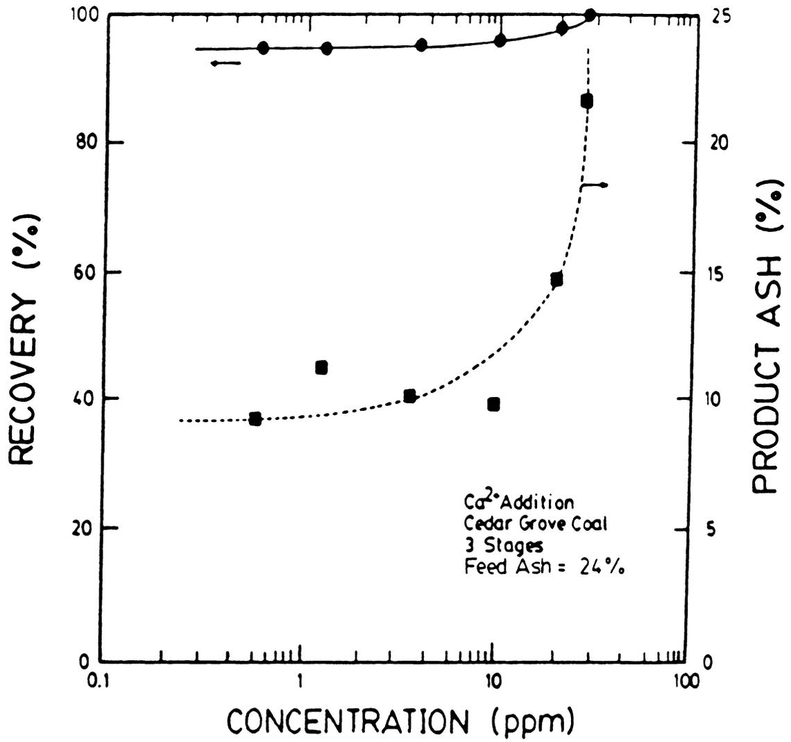
Figure 2.17 Effect of Ca<sup>2+</sup> concentration on coal recovery and product ash percent using double distilled water at pH 9
