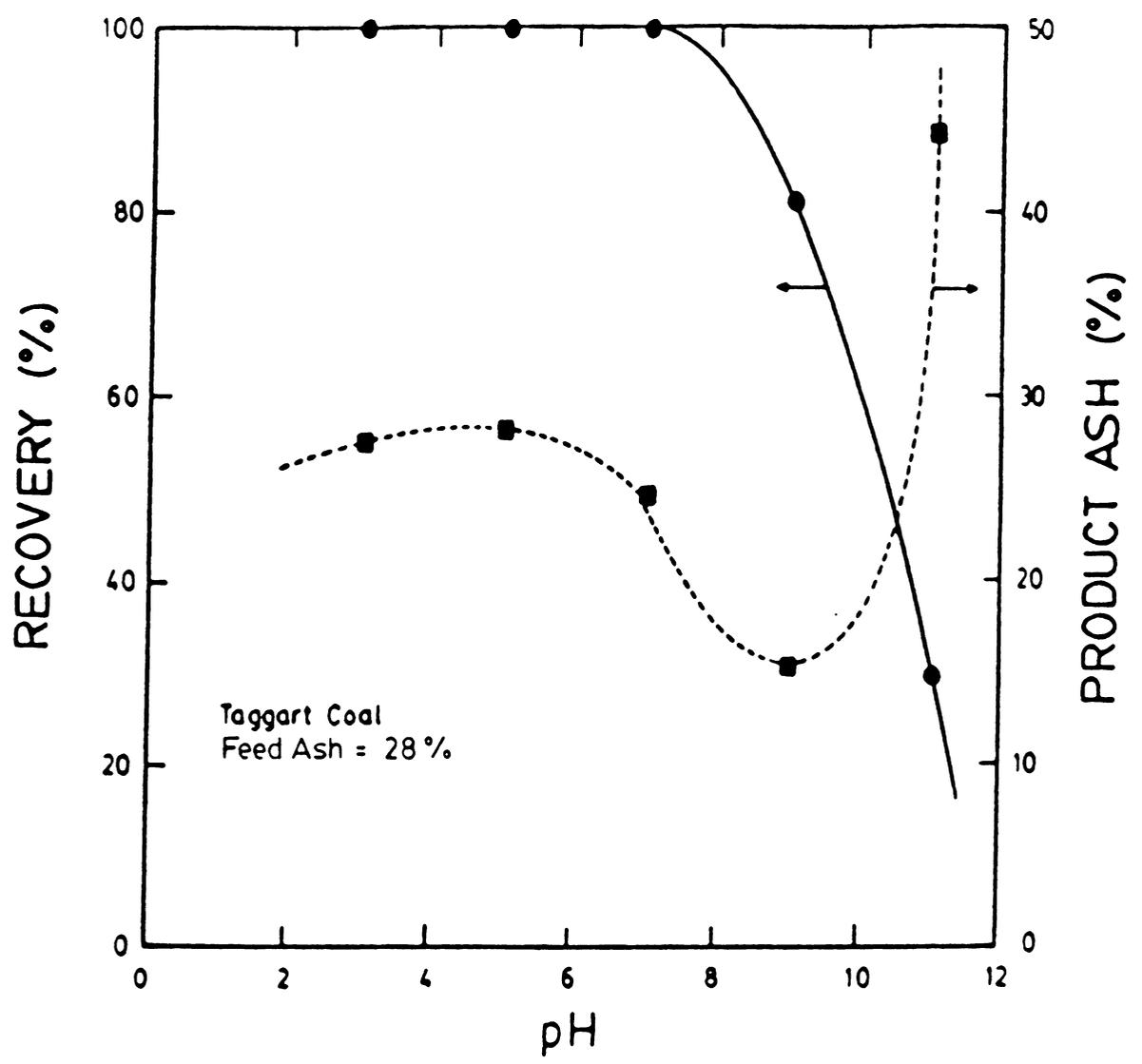
Figure 2.10 The effect of pH on coal recovery and product ash percent for the Taggart coal seam containing 28.0% ash in tap water using 3 cleaning stages.
