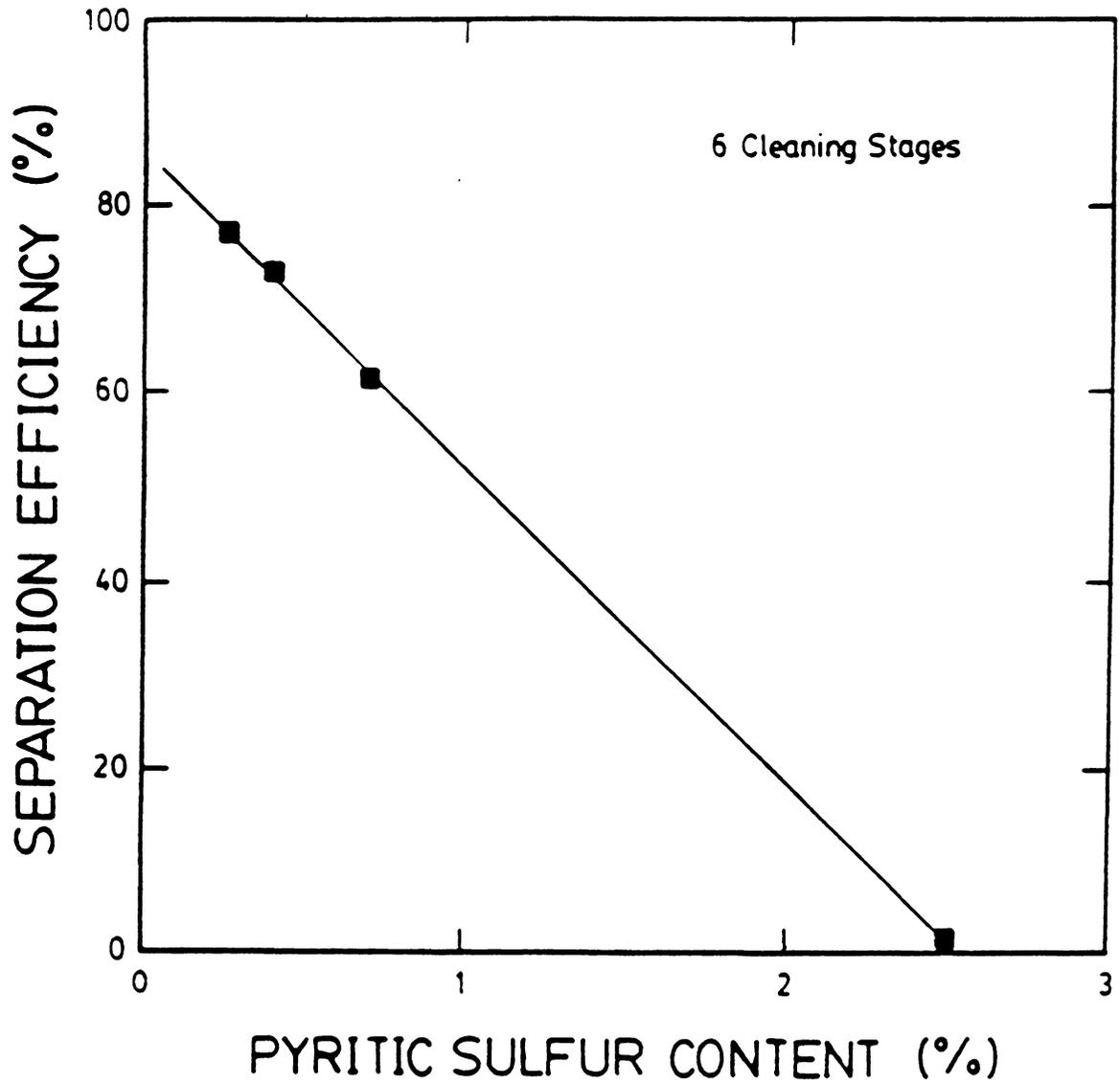
Figure 2.15 The effect of pyritic sulfur content in the feed coal sample on separation efficiency.
