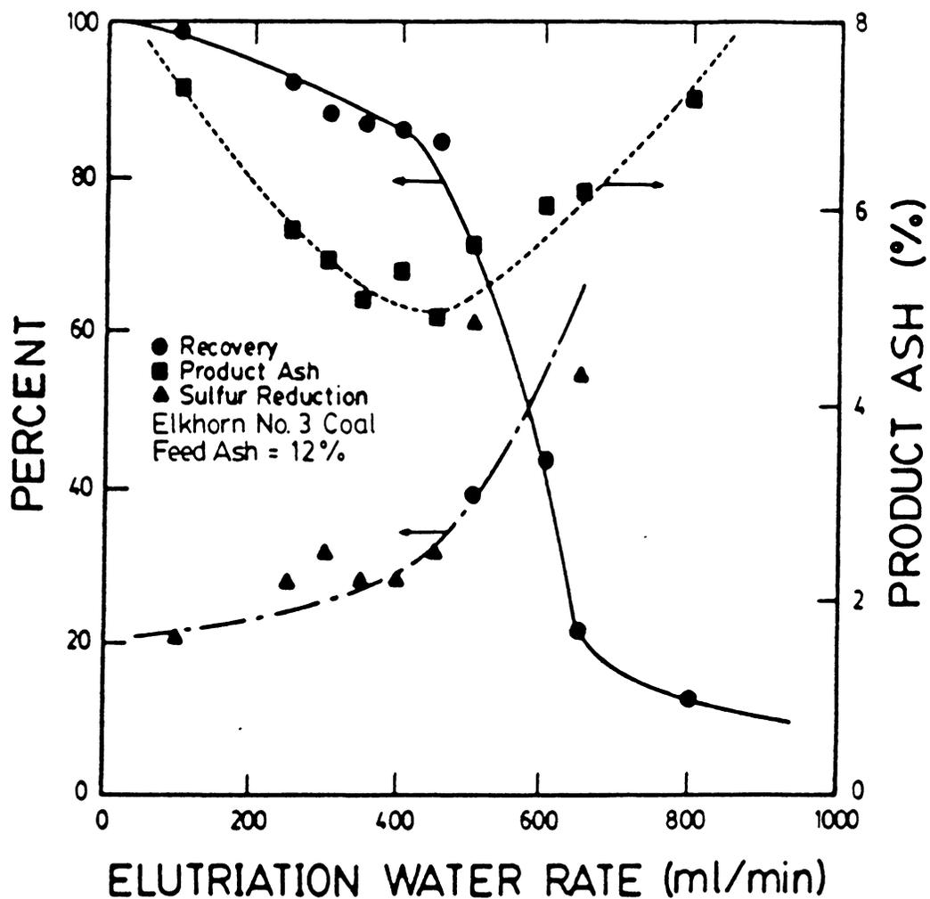
Figure 4.3 The effect of elutriation water rate on coal recovery, sulfur reduction, and product ash percent - feed rate = 50 ml/min.
