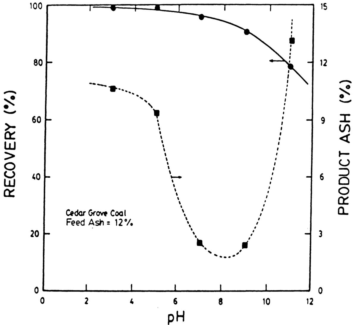
Figure 2.6 The effect of pH on coal recovery and product ash percent for the Upper Cedar Grove coal seam containing 12.0% ash in tap water using 8 cleaning stages.
