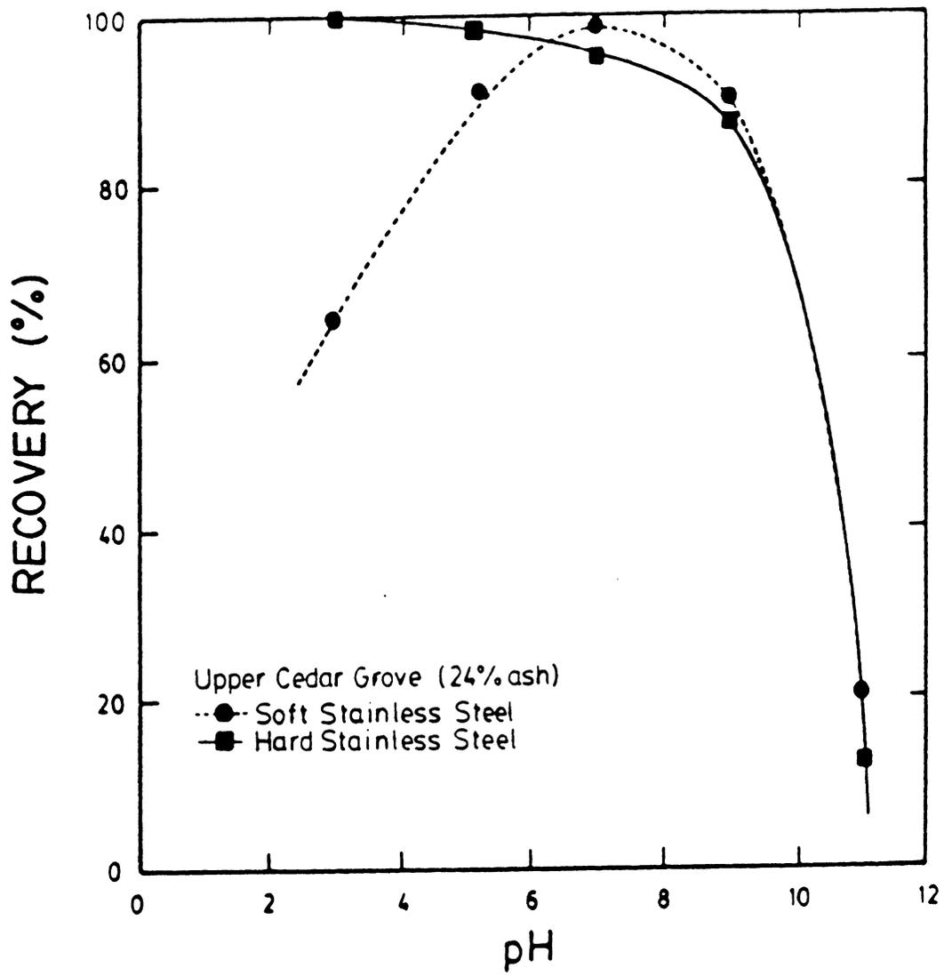
Figure 2.19 Effect of pH on coal recovery when using soft and hard grinding media.
