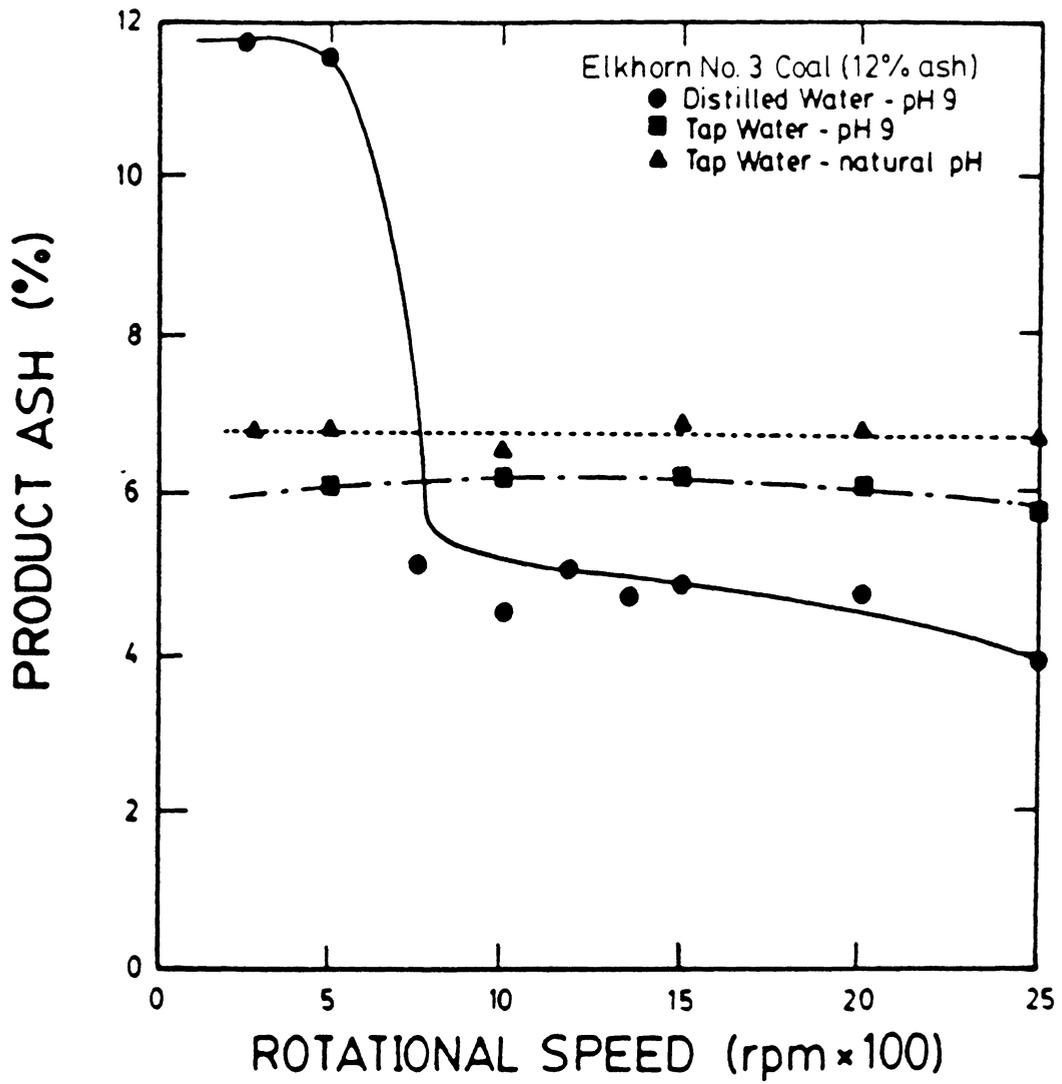
Figure 3.16 Product ash percent versus rotational speed curves for three different media conditions.
