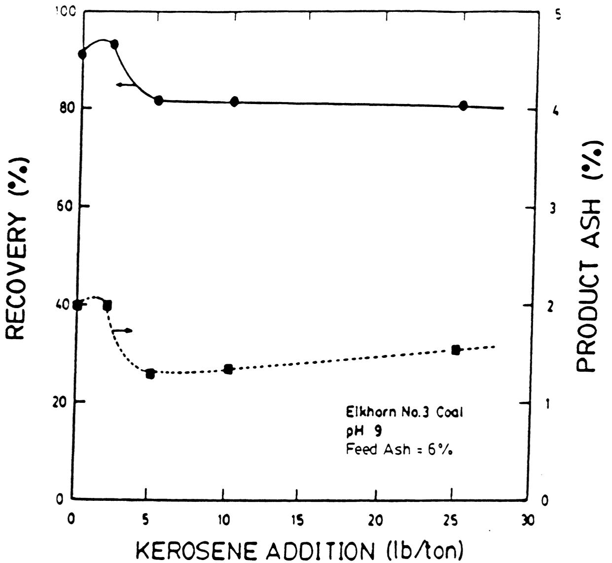
Figure 2.23 The effect of kerosene addition on coal recovery and product ash percent for the Elkhorn No.3 coal seam.
