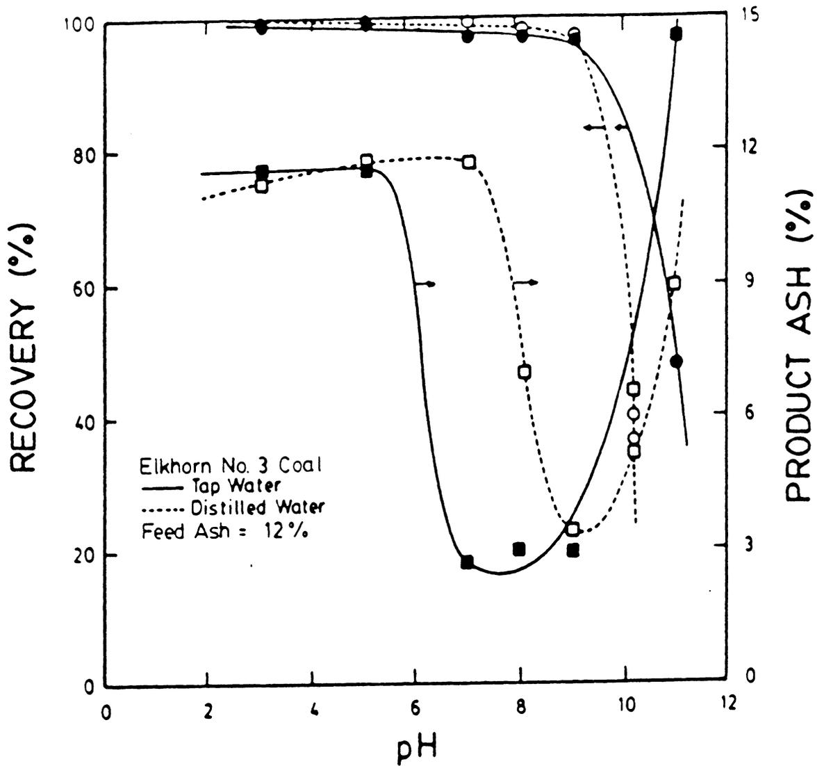
Figure 2.16 A comparison between using tap water and distilled water as the slurry medium over a range in pH for the Elkhorn No.3 coal seam using 3 cleaning stages.
