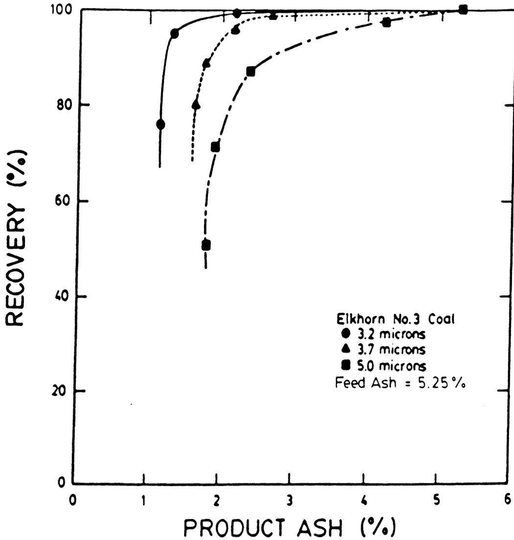
Figure 3.10 Coal recovery versus product ash percent curves for three particle sizes using an Elkhorn No.3 coal seam sample containing 5.25% ash.
