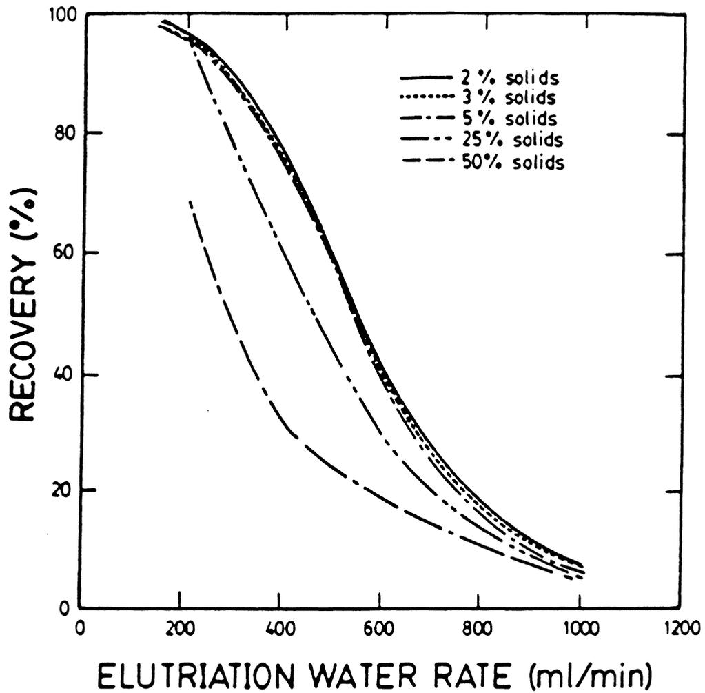
Figure 5.7 Model predictions showing coal recovery versus elutriation water rate for various feed percent solids values.
