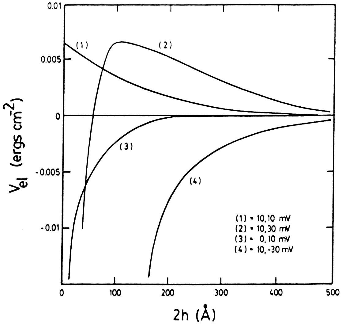
Figure 2.32 The electrostatic potential energy of interaction versus 2 times the particle-particle separation distance -  $c = 1$  mmol/liter - 1-1 electrolyte (Usui, 1984).
