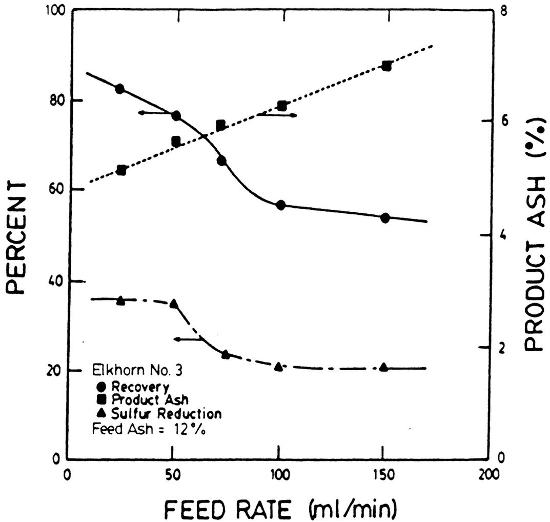
Figure 4.4 The effect of feed rate on coal recovery, sulfur reduction, and product ash percent - elutriation water rate = 400 ml/min.
