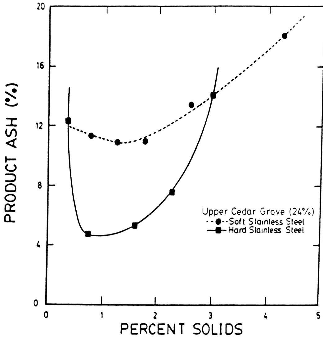
Figure 2.22 The effect of the grinding environment on product ash percent.
