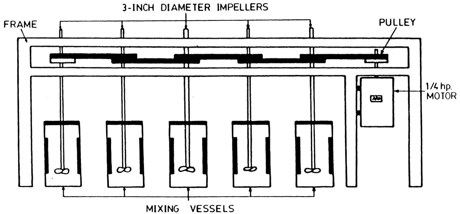
Figure 2.1 The five-cell mixing device used for the batch-type experiments .
