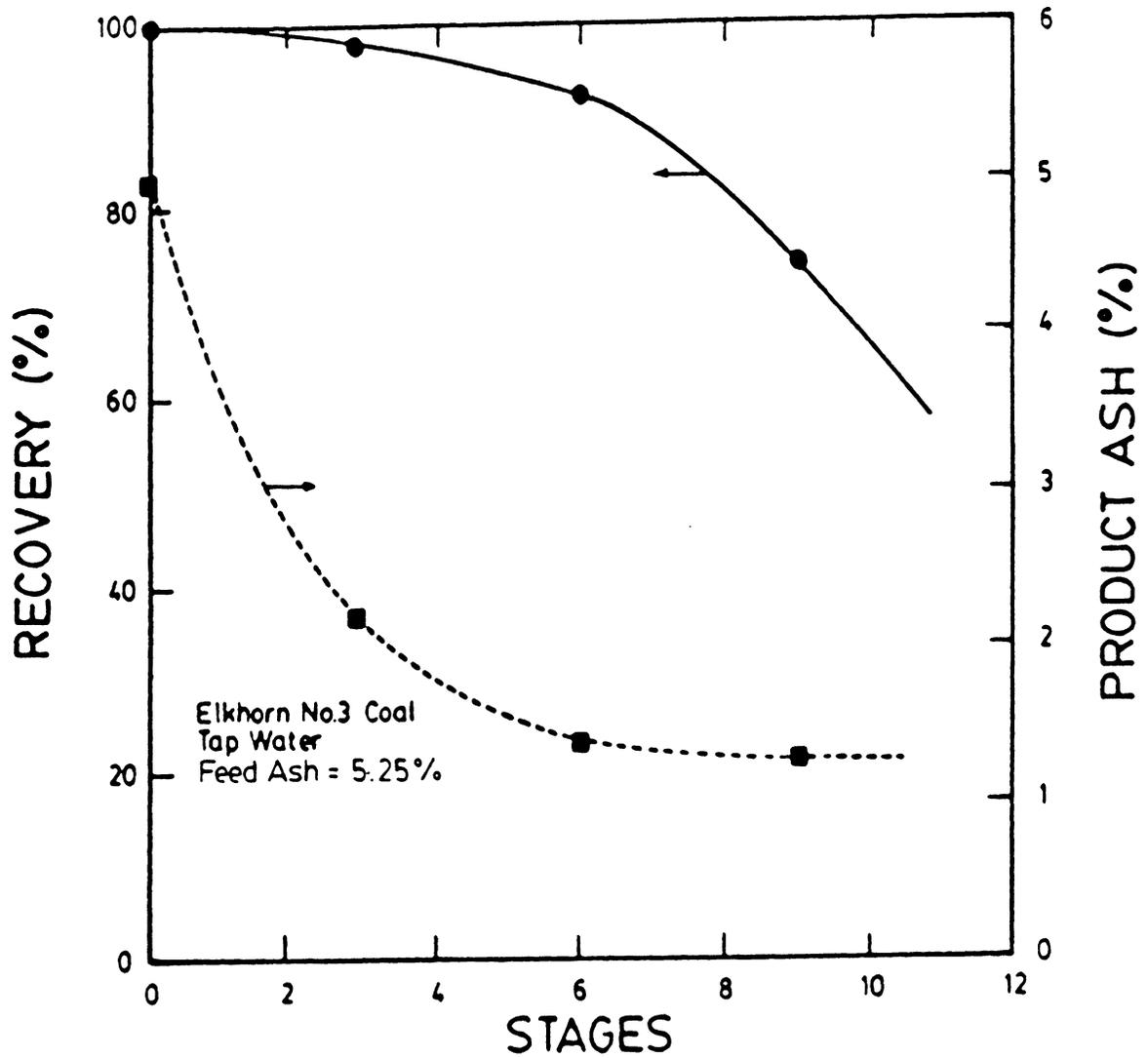
Figure 3.2 The effect of cleaning stages on recovery and product ash percent for the Elkhorn No.3 coal seam containing 5.25% ash.
