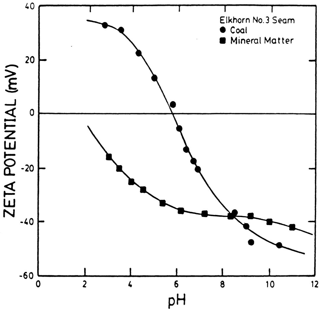
Figure 2.25 Zeta potential measurements over a range in pH for Elkhorn No.3 coal and mineral matter in distilled water.
