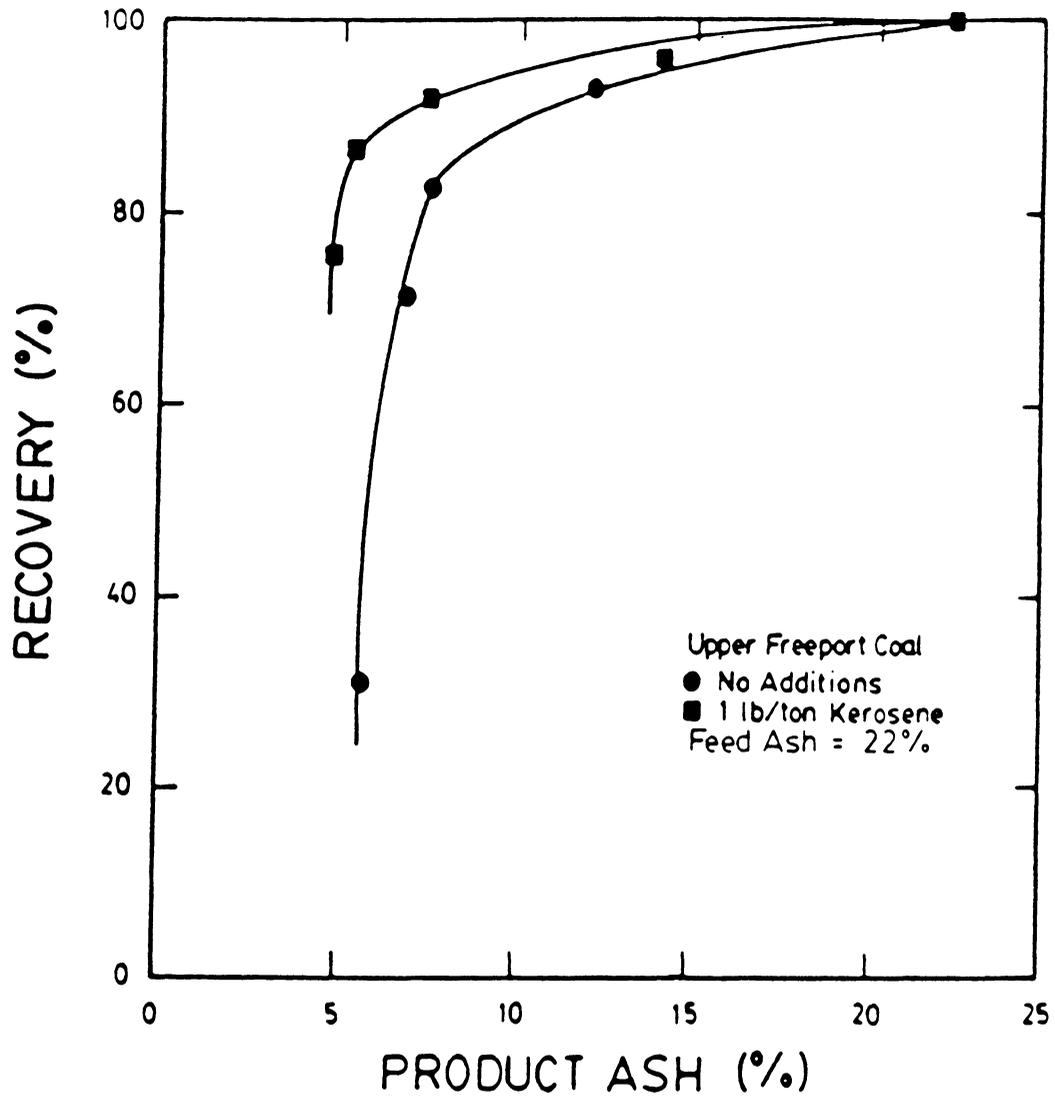
Figure 2.24 The effect of adding 1 lb/ton of kerosene on coal recovery and product ash percent for the Upper Freeport coal seam.
