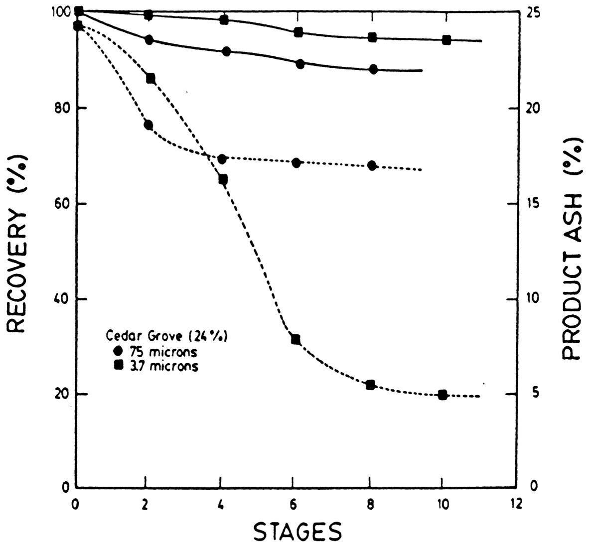
Figure 3.9 Coal recovery versus product ash percent curves for two particle sizes using the Upper Cedar Grove coal seam containing 24% ash.
