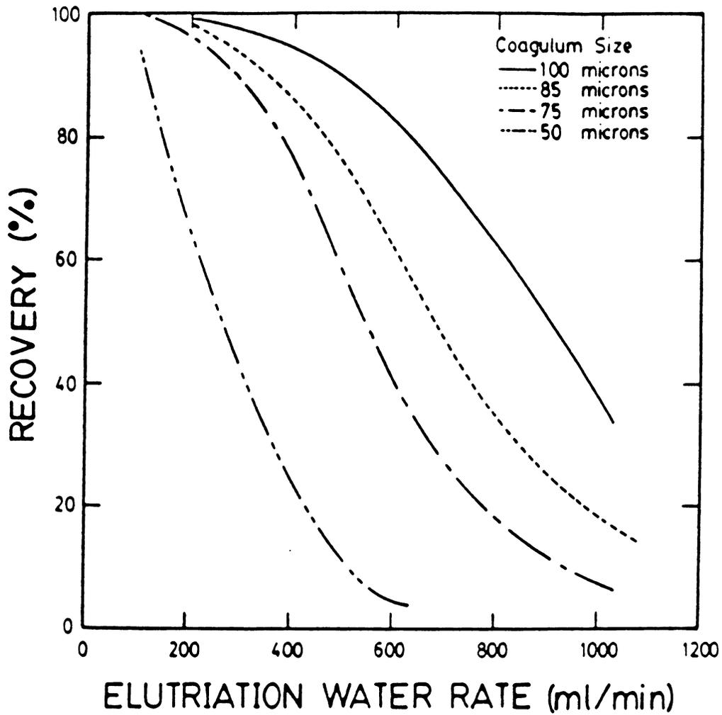
Figure 5.4 Model predictions on the effect of elutriation water rate on coal recovery over a range of coagulum sizes.
