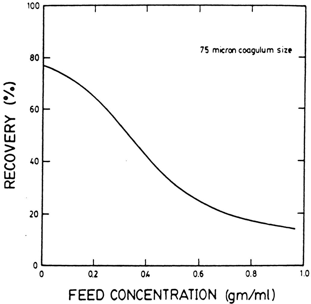
Figure 5.6 Model predictions on the effect of feed solids concentration on coal recovery.
