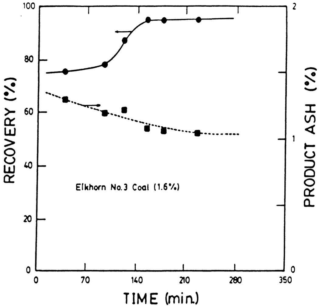
Figure 4.10 Coal recovery and product ash percent versus accumulated operation time for Elkhorn No.3 coal seam containing 1.6% ash.
