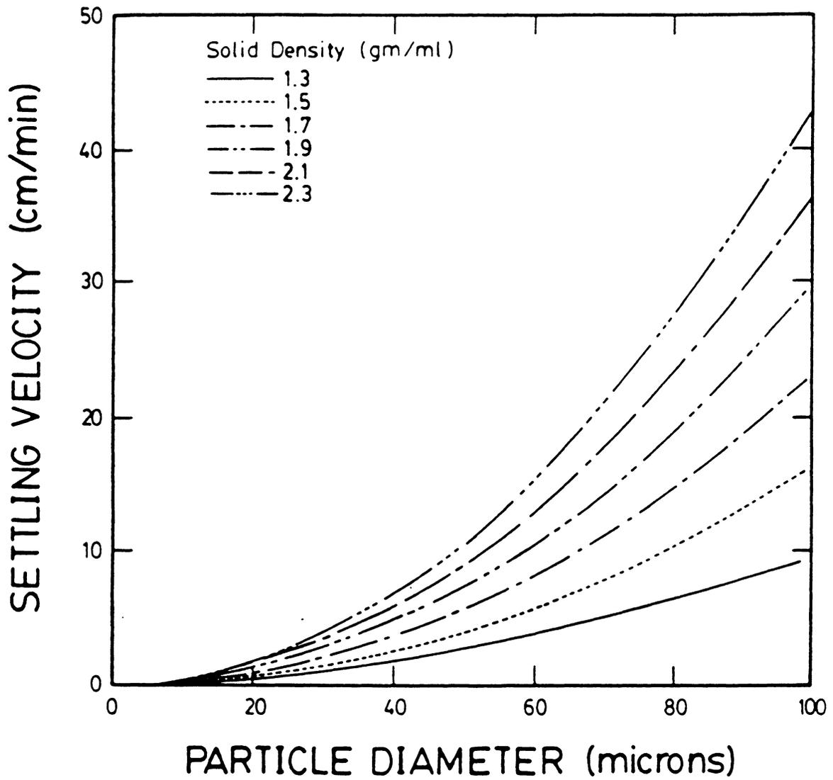
Figure 4.12 The effect of particle diameter and solid density on particle settling velocity according to Stoke's equation.
