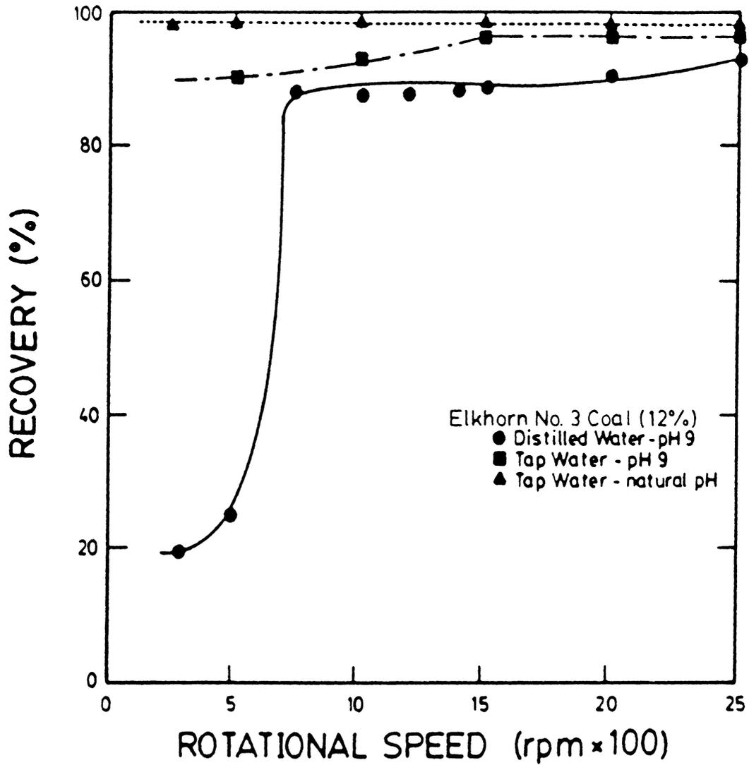
Figure 3.15 Coal recovery versus rotational speed curves for three different media conditions.
