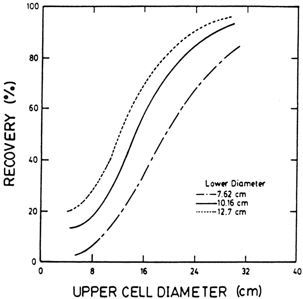
Figure 5.10 Model predictions showing the effect of both the upper and lower cell diameters on coal recovery.
