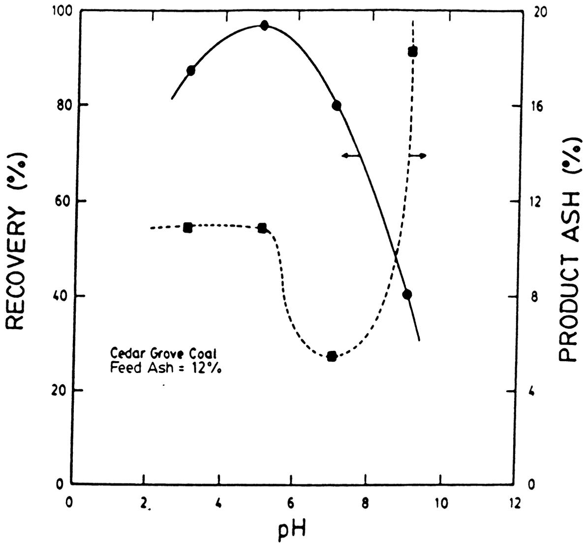
Figure 2.8 The effect of pH on coal recovery and product ash percent for the Upper Cedar Grove coal seam containing 12 % ash in tap water using 3 cleaning stages.
