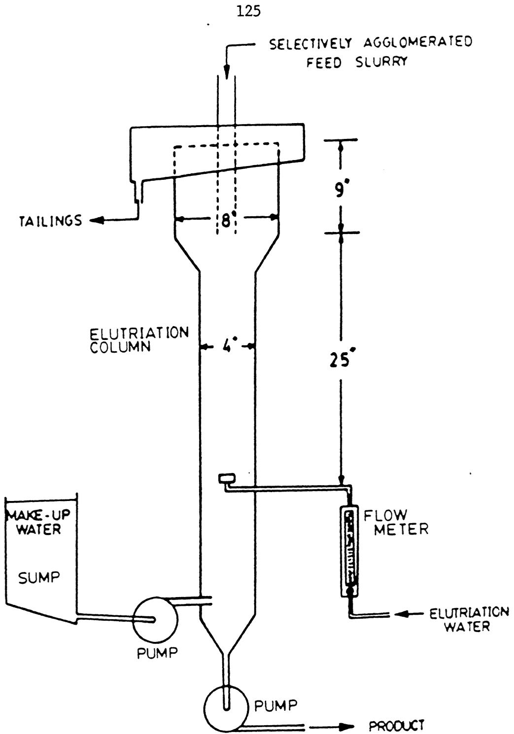
Figure 4.2 Diagram of the continuous elutriation column.
