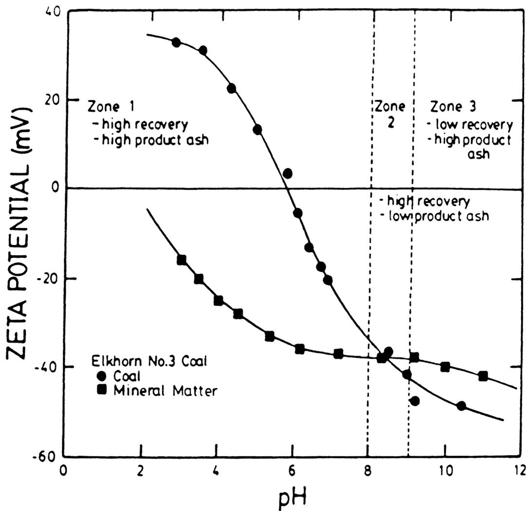
Figure 2.31 A comparison of process performance and zeta potential measurements over a range in pH - distilled water.
