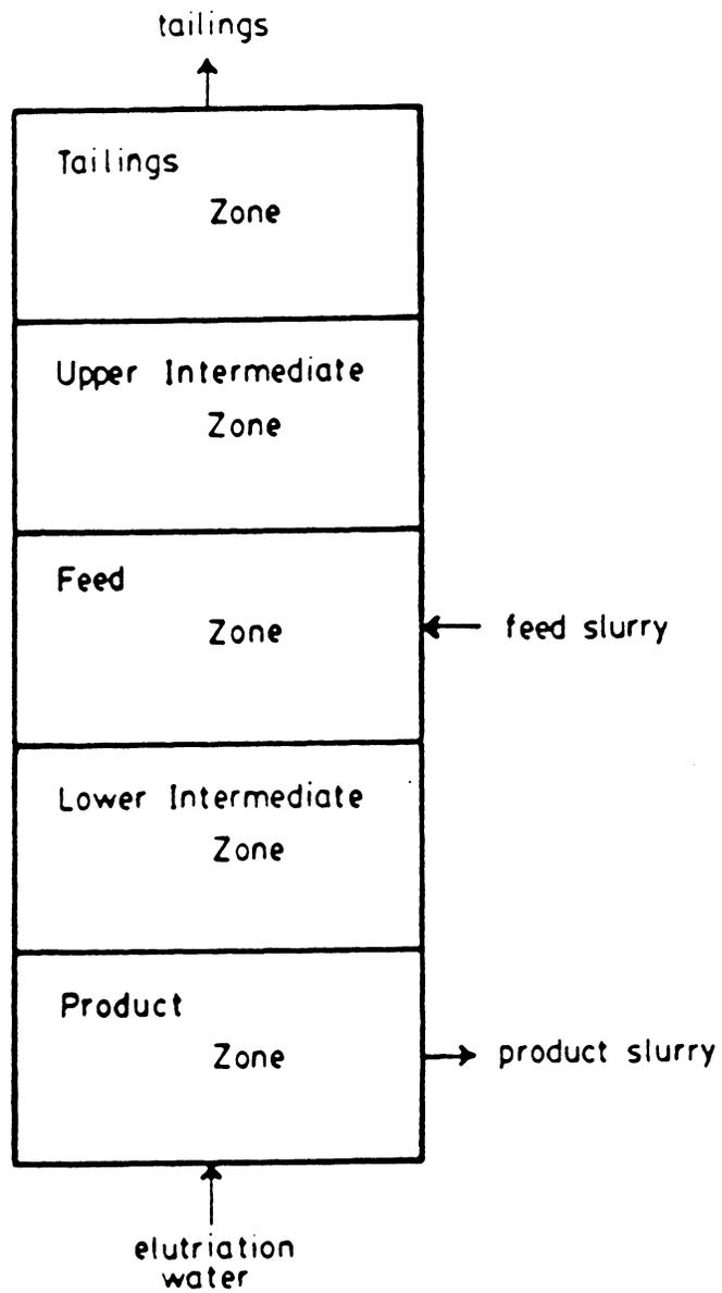
Figure 5.2 Schematic representation of the sections in an elutriation column.
