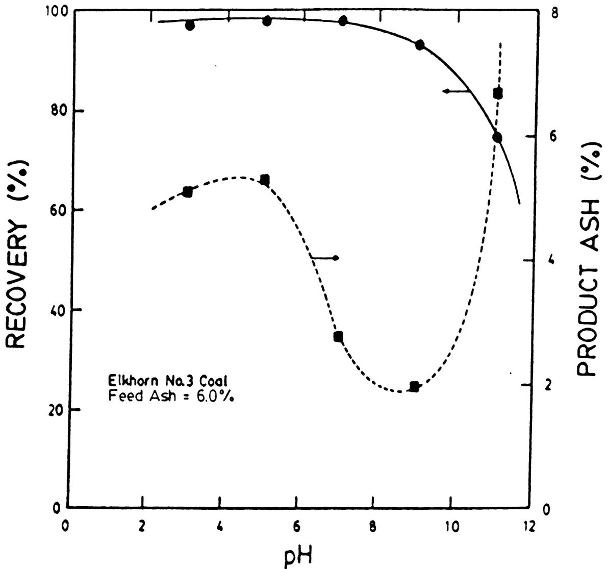
Figure 2.5 The effect of pH on coal recovery and product ash percent for the Elkhorn No. 3 coal seam containing 6.0% ash in tap water using 3 cleaning stages.
