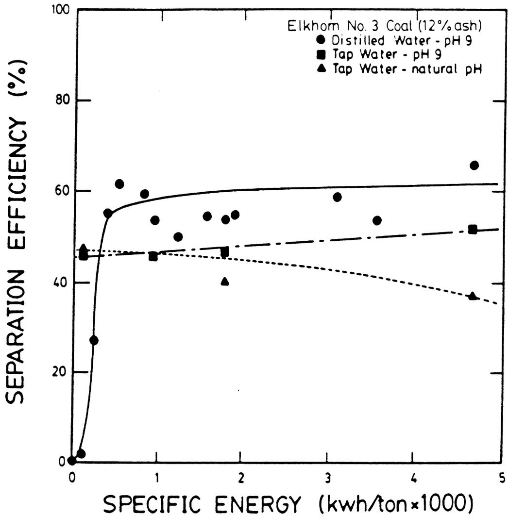
Figure 3.19 The effect of specific energy input on separation efficiency for 3 media conditions; specific energy accumulated over 3 cleaning stages.
