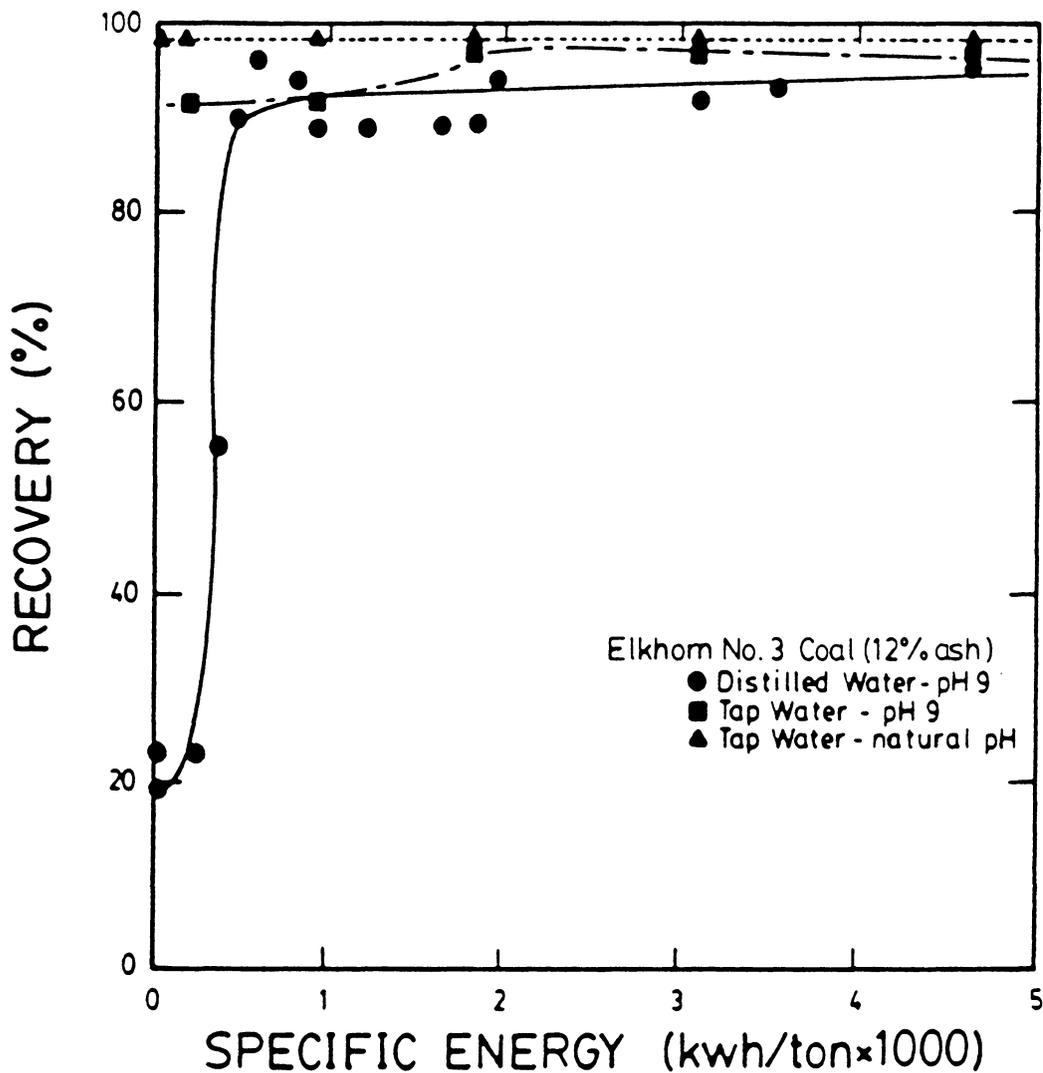
Figure 3.17 The effect of specific energy input on recovery for 3 media conditions; specific energy accumulated over 3 cleaning stages.
