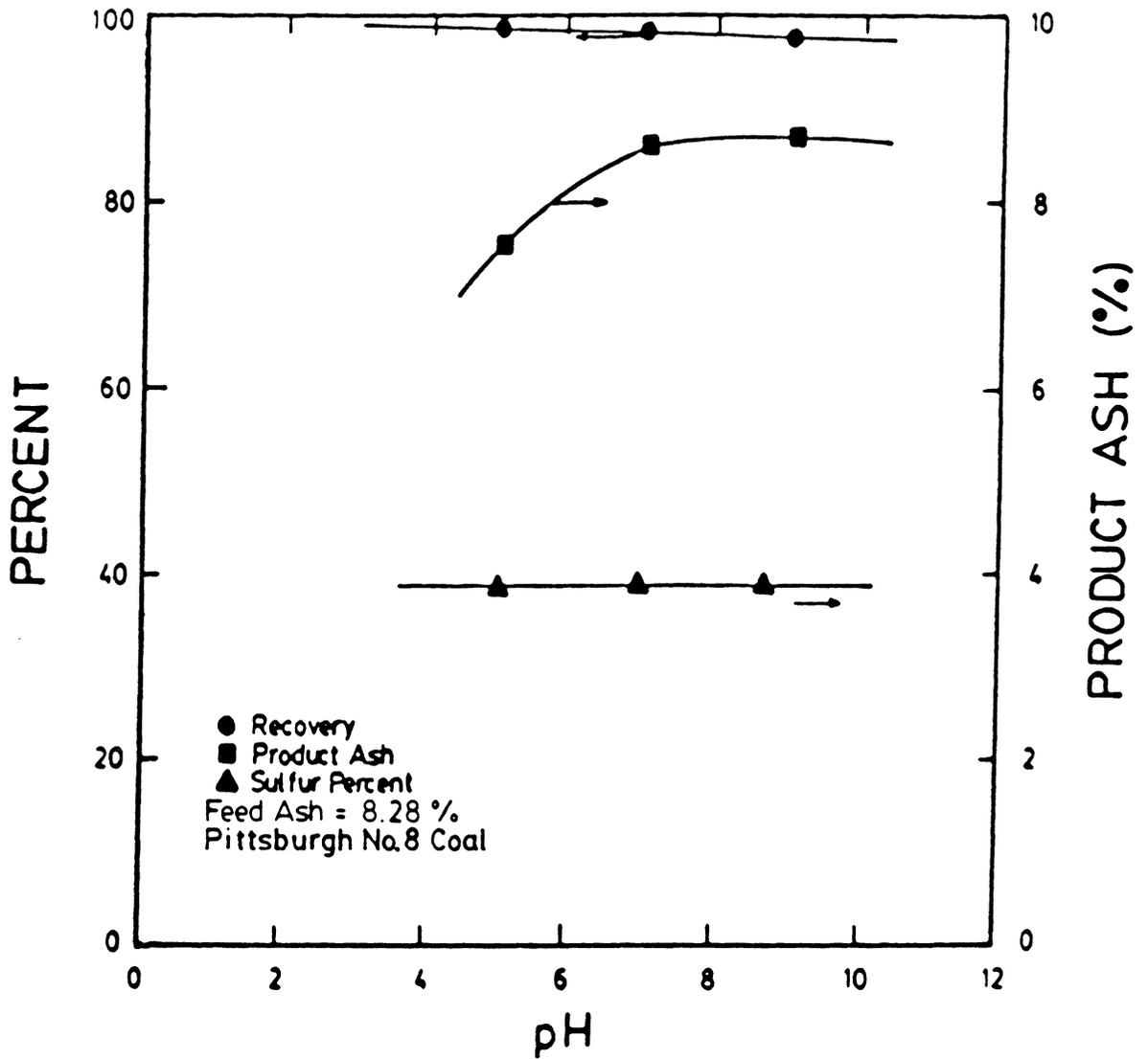
Figure 2.14 The effect of pH on coal recovery and product ash percent for the Pittsburgh No. 8 coal seam containing 8.28% ash in tap water using 3 cleaning stages.
