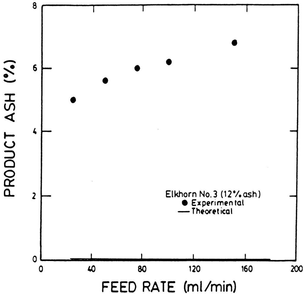
Figure 5.14 A comparison between model predictions and experimental results showing the effect of feed rate on product ash percent.
