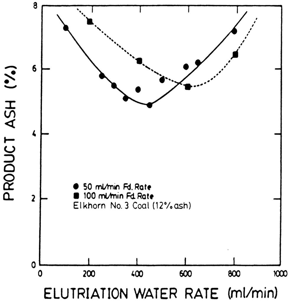
Figure 4.6 Product ash percent versus elutriation water rate curves for 2 feed rates.
