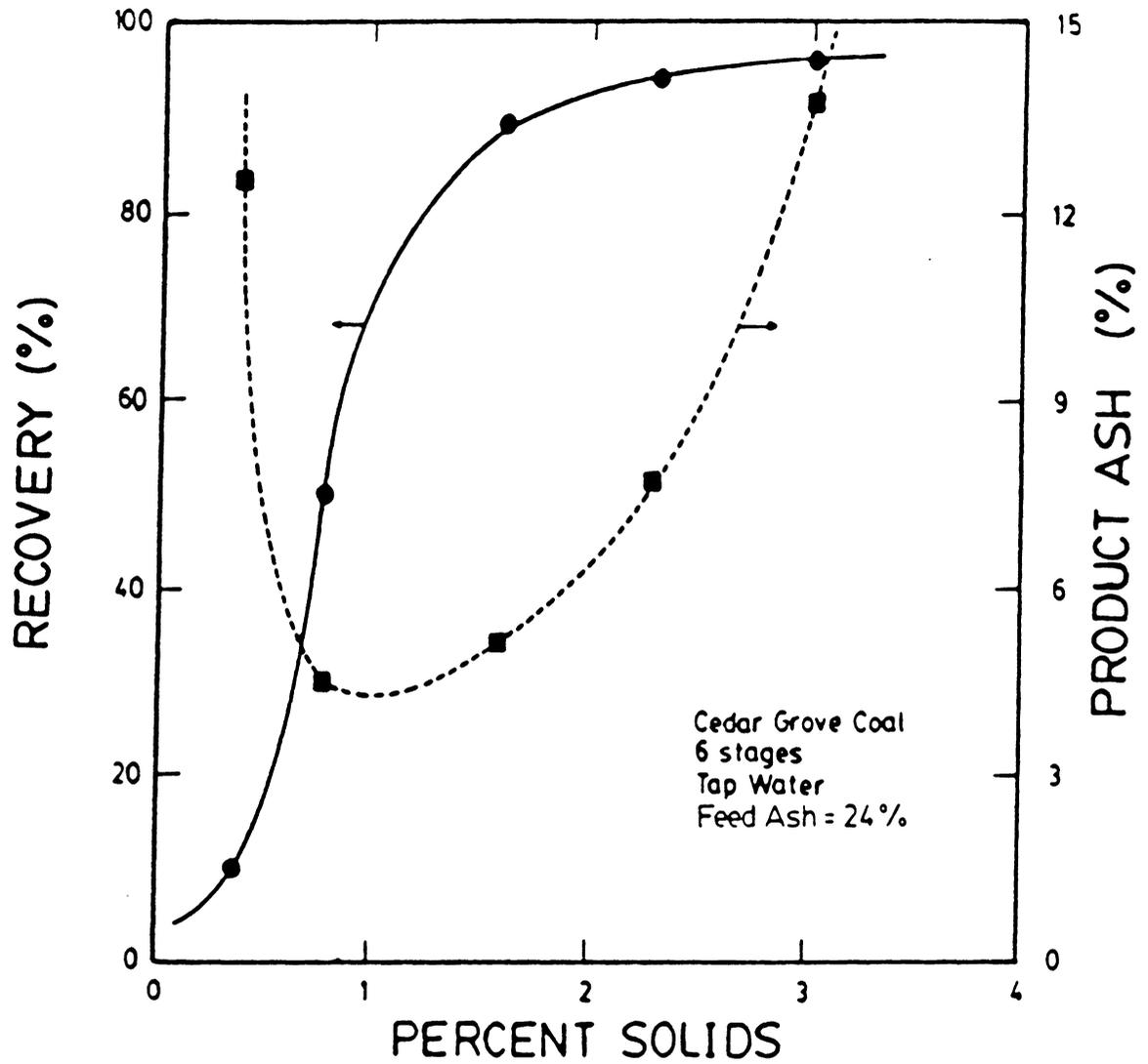
Figure 3.6 The effect of % solids on coal recovery product ash percent for the Upper Cedar Grove coal seam containing 24% ash.
