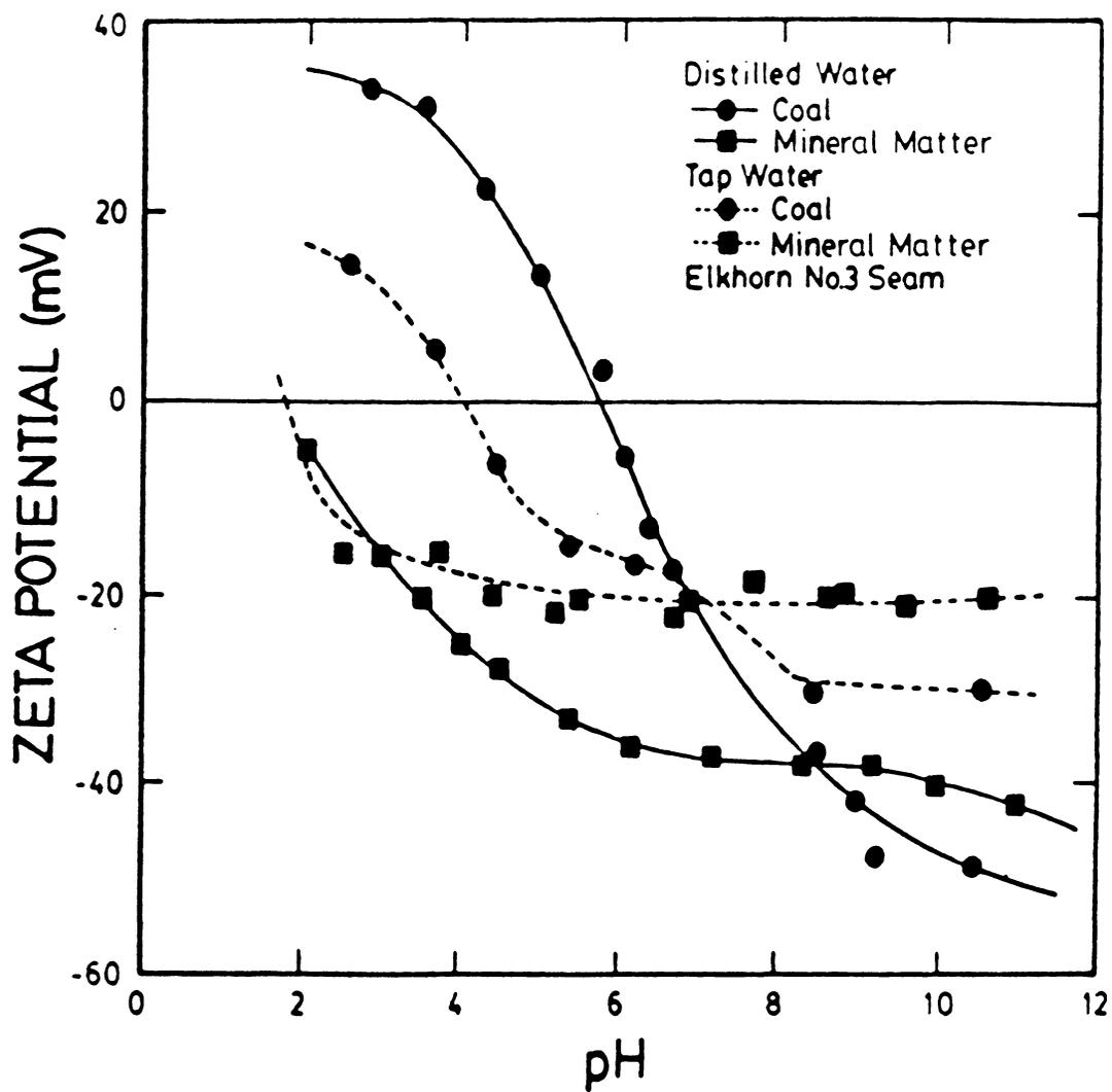
Figure 2.28 A comparison of zeta potential measurements over a range in pH between tap water and distilled water mediums.
