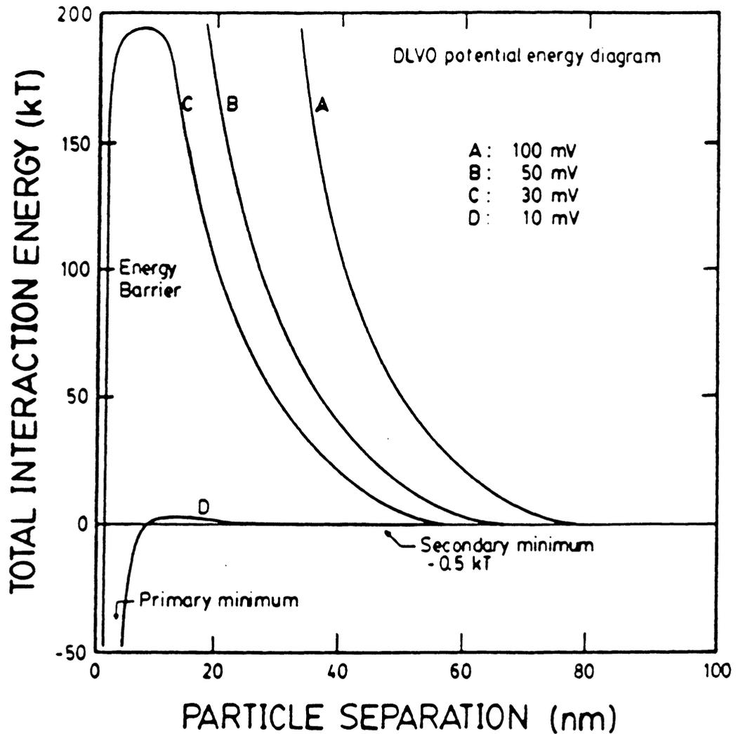
Figure 3.21 Total potential energy of interaction between particles of 1 micron diameter in 0.001 M electrolyte, as calculated by DLVO theory - constant potential assumption (Wiese and Healy, 1970).
