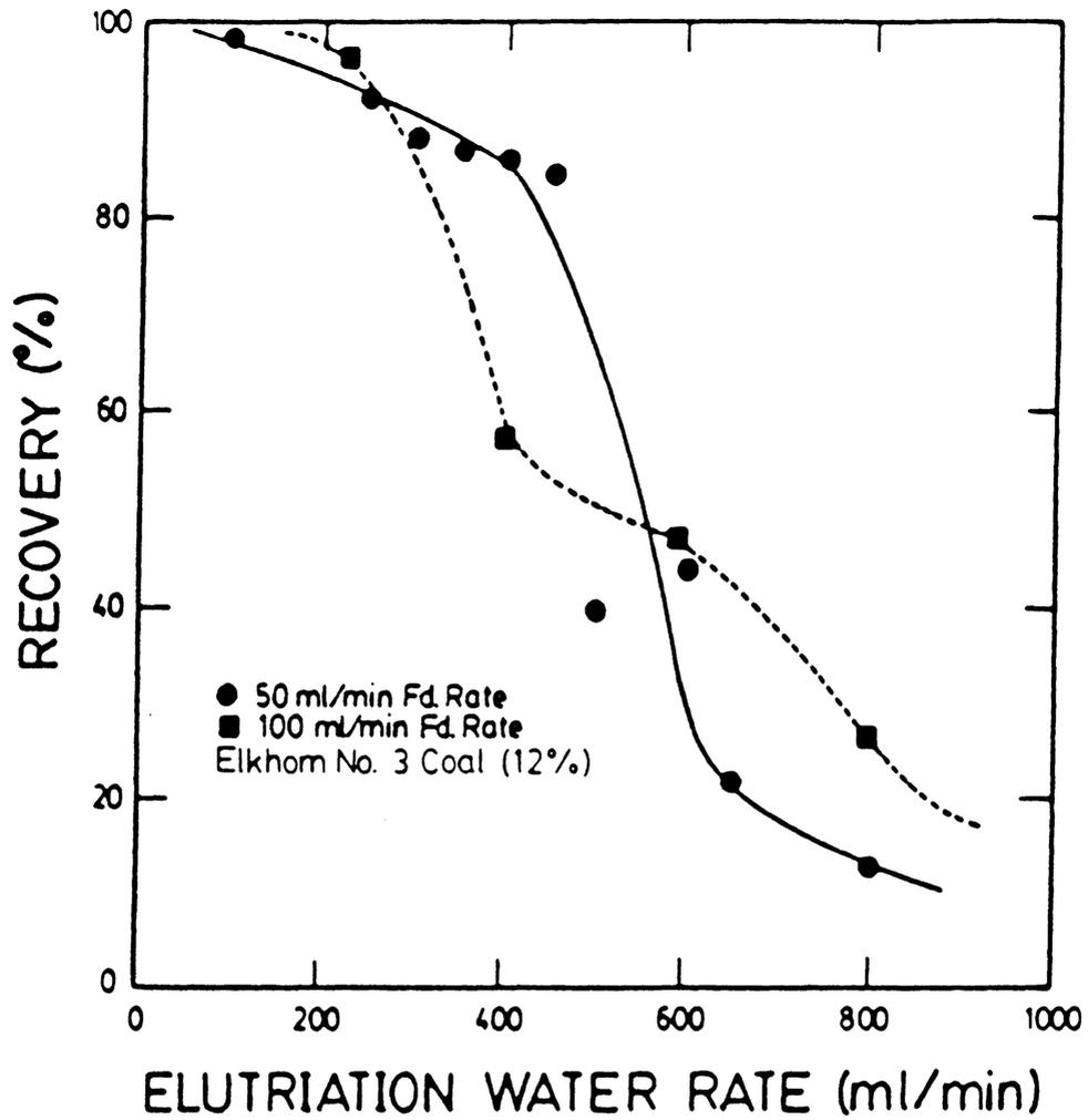
Figure 4.5 Coal recovery versus elutriation water rate curves for 2 feed rates.
