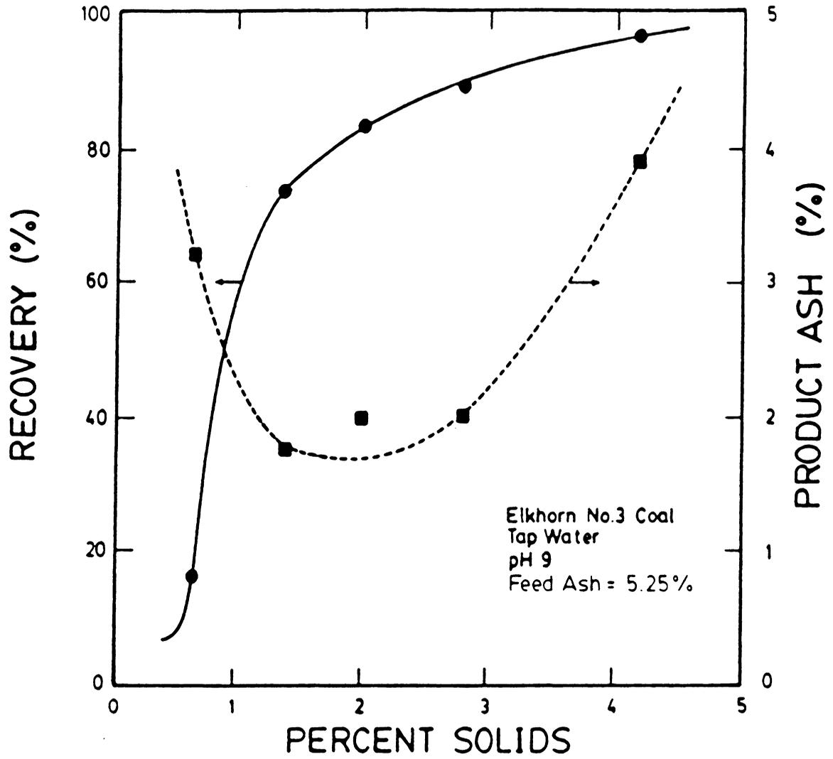
Figure 3.7 The effect of percent solids on coal recovery and product ash percent for the Elkhorn No.3 coal seam containing 5.25% ash.
