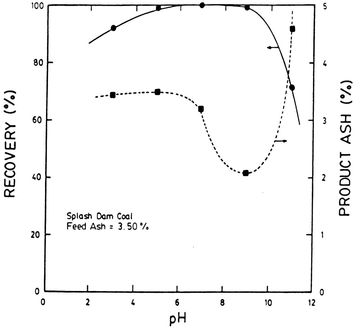
Figure 2.11 The effect of pH on coal recovery and product ash percent for the Splash Dam coal seam containing 3.5% ash in tap water using 3 cleaning stages.
