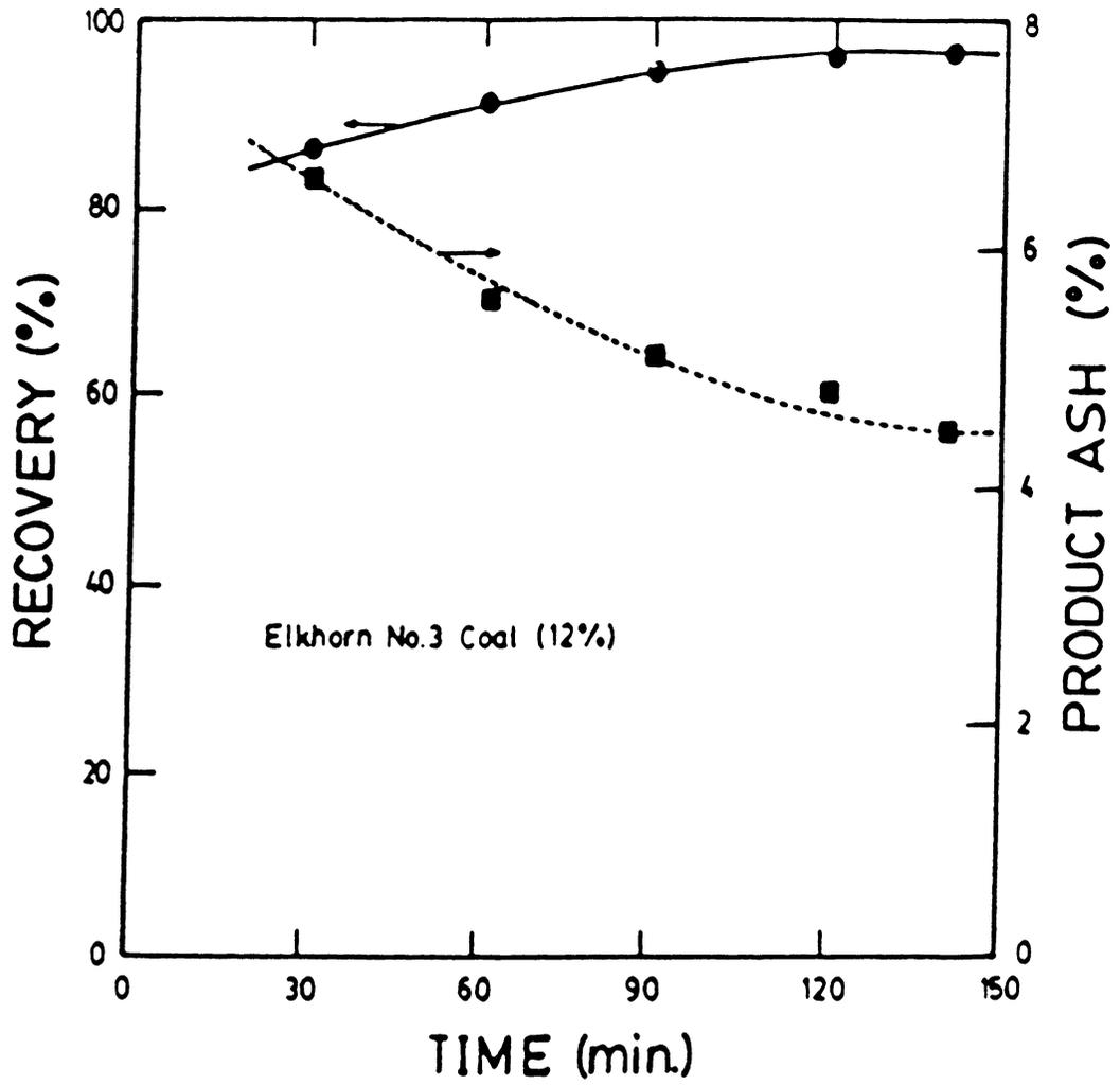
Figure 4.9 Coal recovery and product ash percent versus accumulated operation time for Elkhorn No.3 coal seam containing 12% ash.
