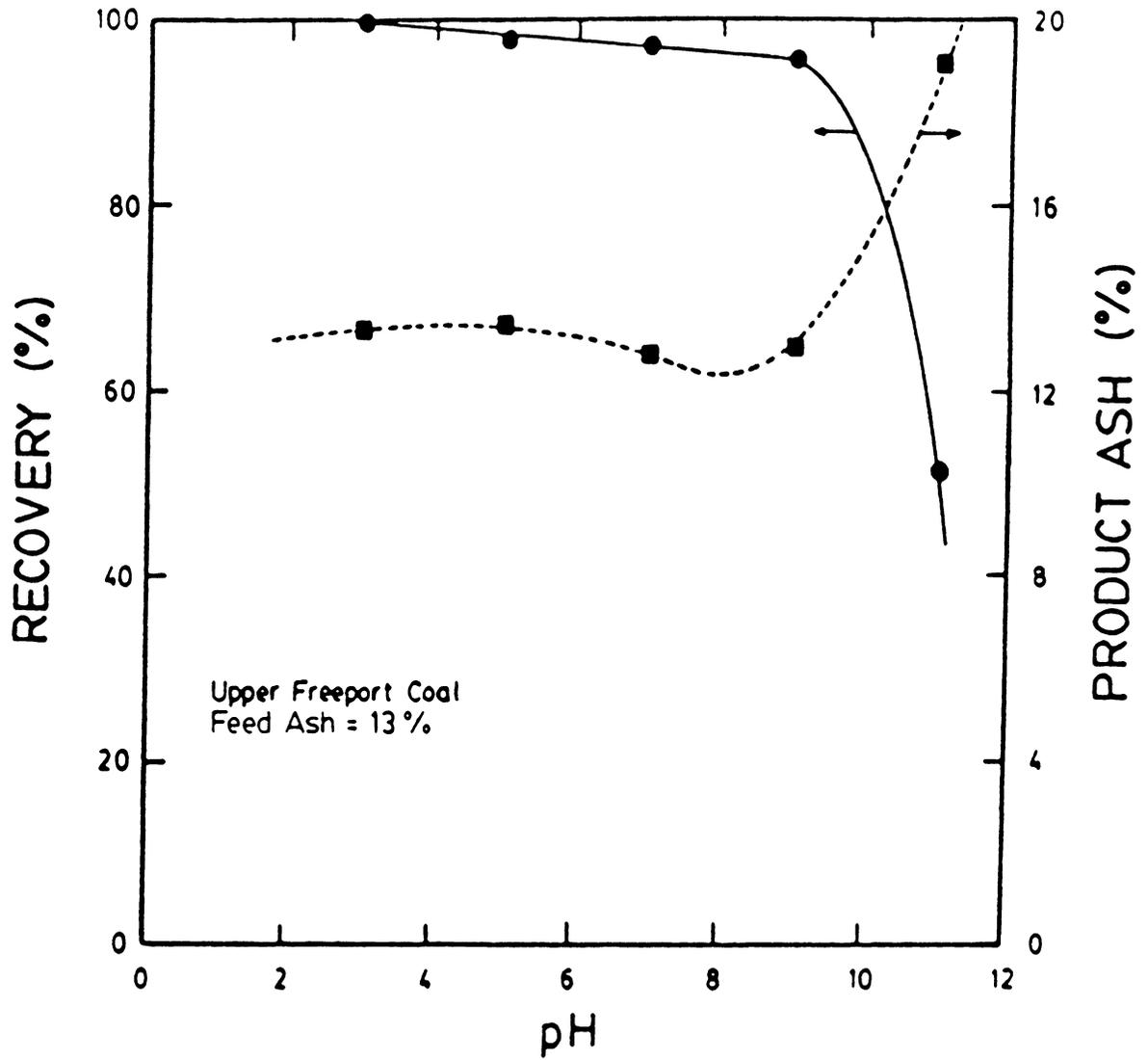
Figure 2.12 The effect of pH on coal recovery and product ash percent for the Upper Freeport coal seam containing 13.0% ash in tap water using 3 cleaning stages.
