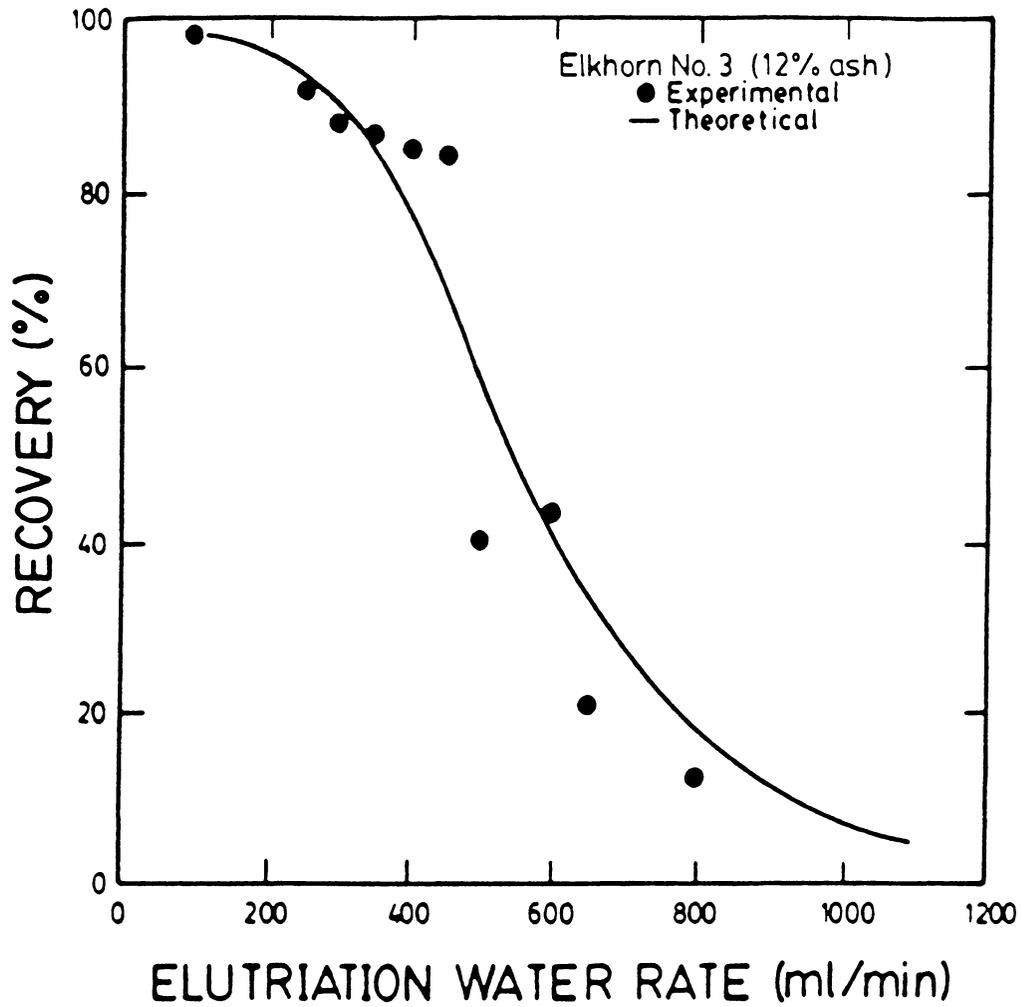
Figure 5.11 A comparison between model predictions and experimental results showing the effect of elutriation water rate on coal recovery.
