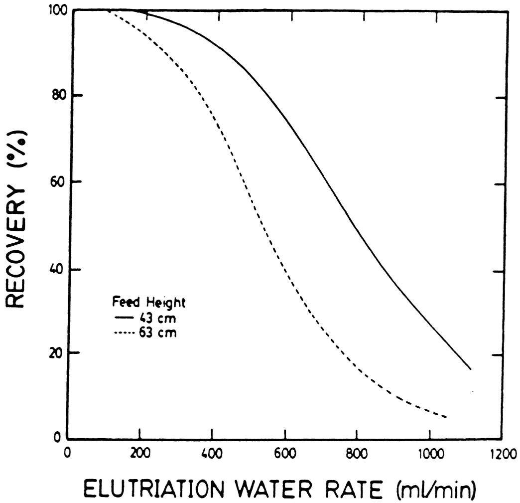
Figure 5.8 Model predictions showing the effect of feed height on coal recovery over a range of elutriation water rates.
