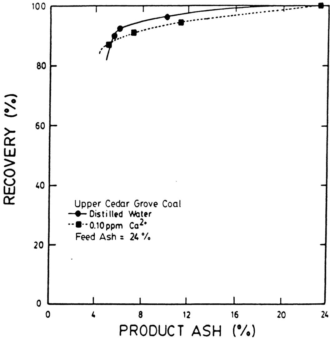
Figure 2.18 Effect of a small  $\text{Ca}^{2+}$  concentration on coal recovery and product ash percent.
