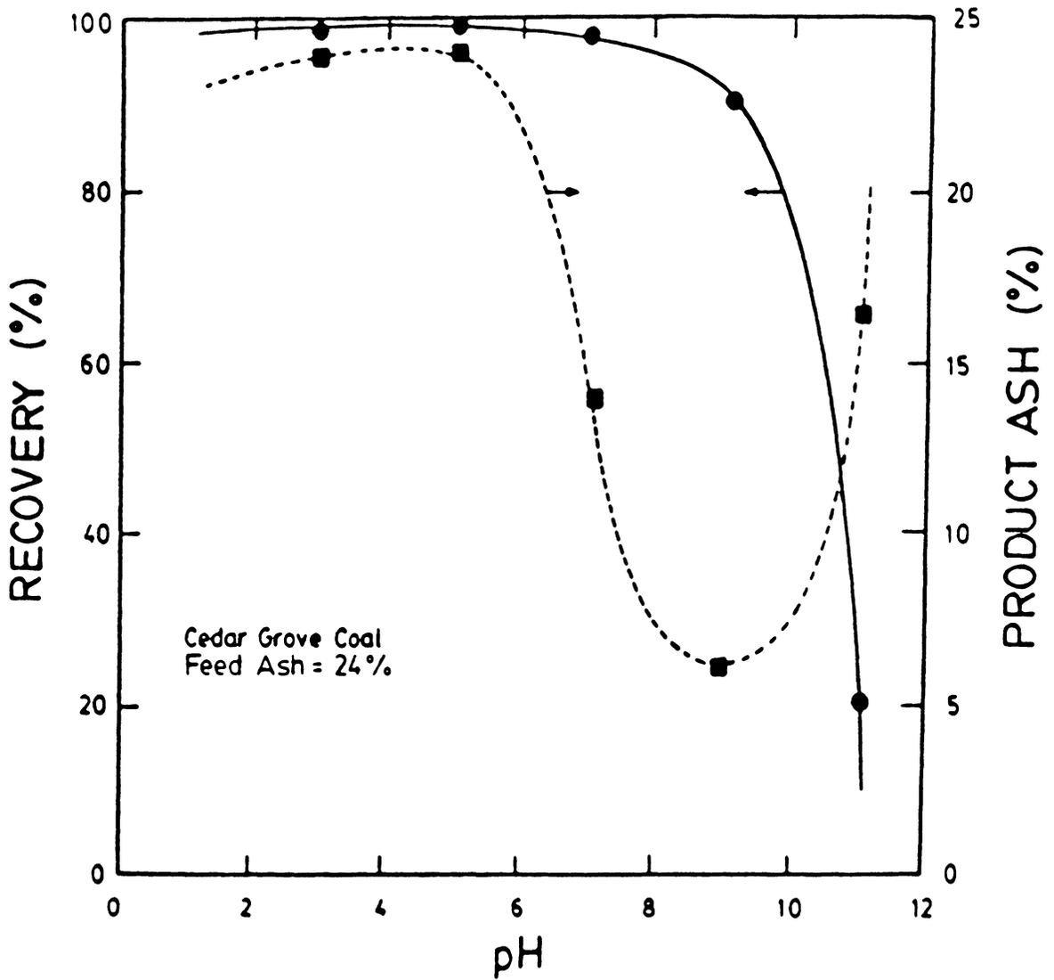
Figure 2.7 The effect of pH on coal recovery and product ash percent for the Upper Cedar Grove coal seam containing 24.0 % ash in distilled water using 8 cleaning stages.
