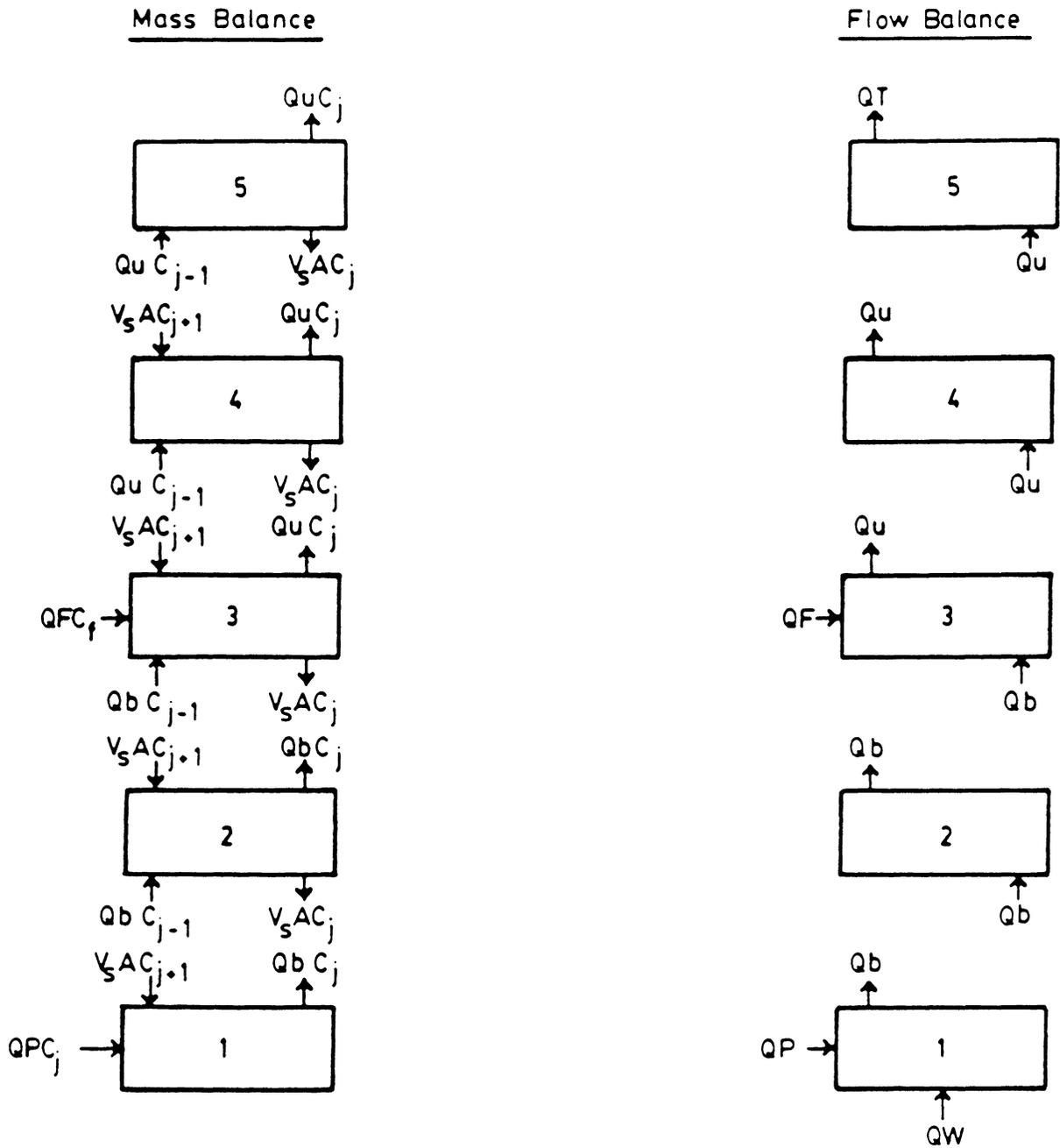
Figure 5.3 Schematic representation of the mass and volumetric flow balances for the column.
