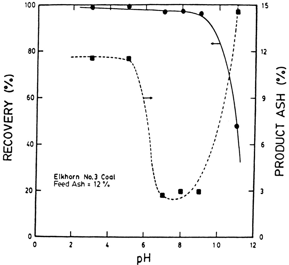
Figure 2.4 The effect of pH on coal recovery and product ash percent for the Elkhorn No.3 coal seam containing 12% ash in tap water using 3 cleaning stages.
