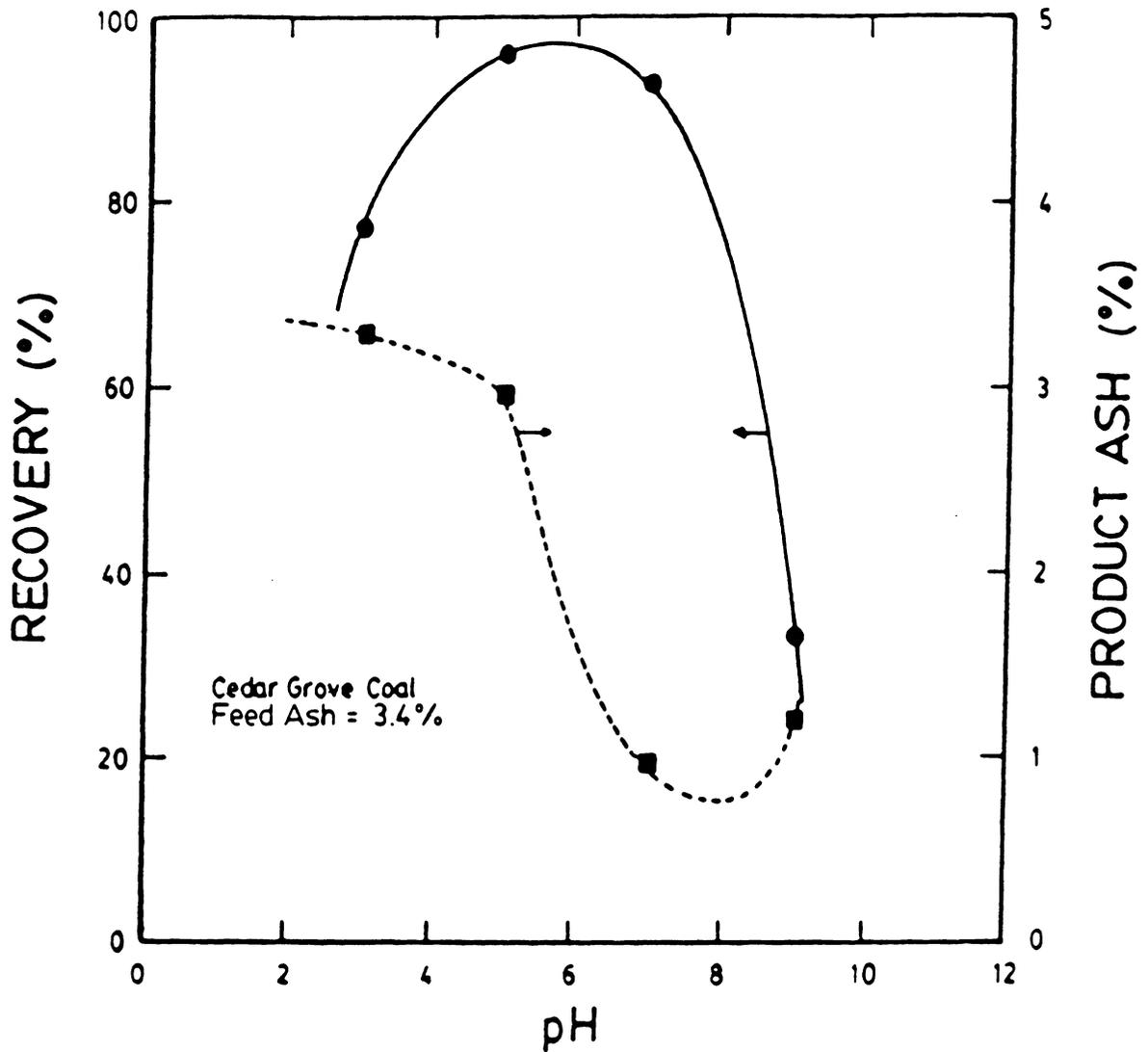
Figure 2.9 The effect of pH on coal recovery and product ash percent for the Upper Cedar Grove coal seam containing 3.4% ash in tap water using 8 cleaning stages.
