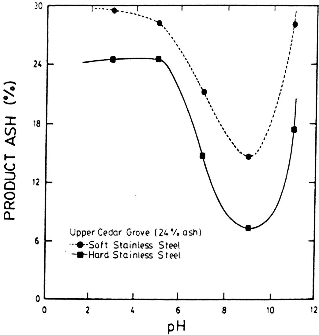
Figure 2.20 Effect of pH on product ash percent when using soft and hard grinding media.
