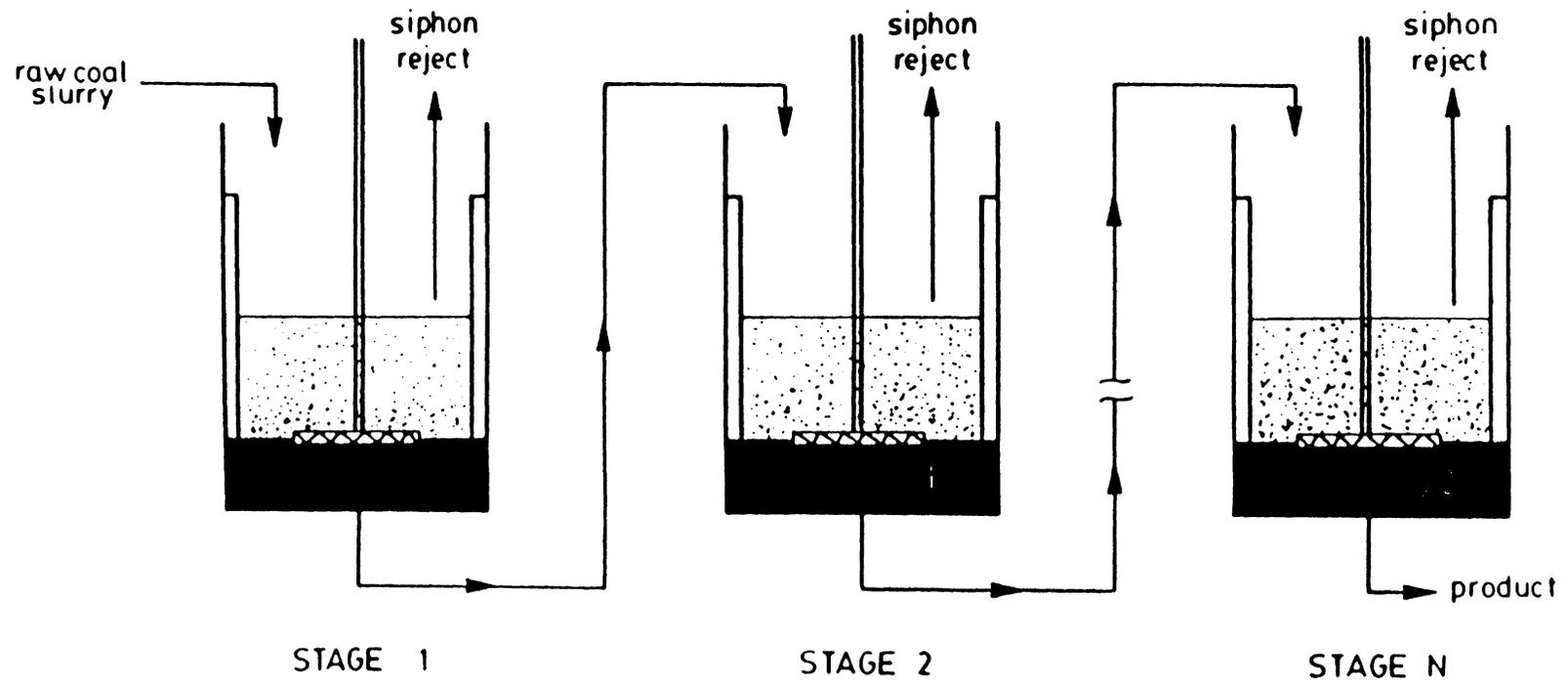
Figure 2.3 Schematic illustration of multiple cleaning stages.
