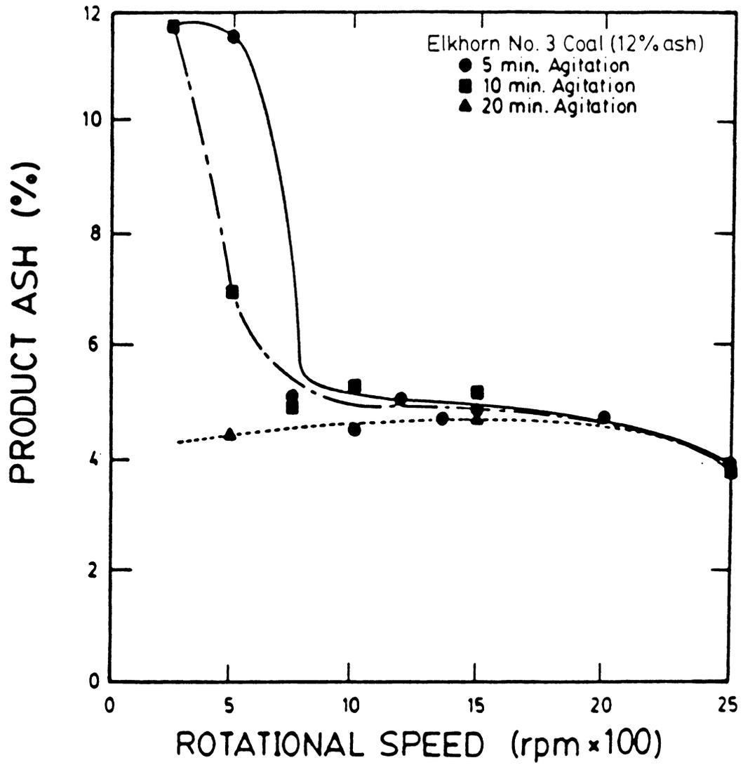
Figure 3.14 The effect of rotational speed on product ash percent for three agitation times.
