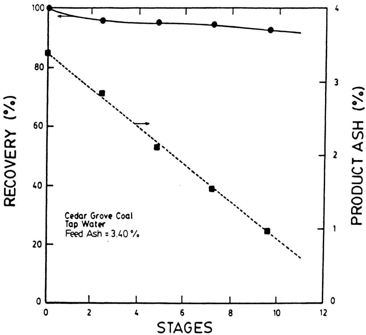
Figure 3.4 The effect of cleaning stages on recovery and product ash percent for the Upper Cedar Grove coal seam containing 3.4% ash.
