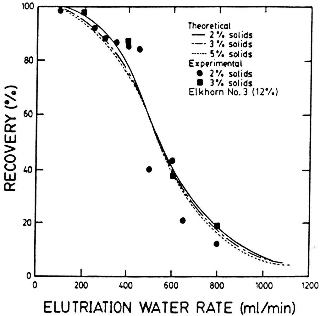
Figure 5.15 A comparison between model predictions and experimental results showing the effect of feed percent solids on coal recovery over a range of elutriation water rates.
