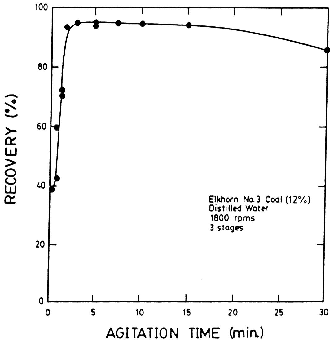
Figure 3.11 The effect of agitation time on coal recovery.
