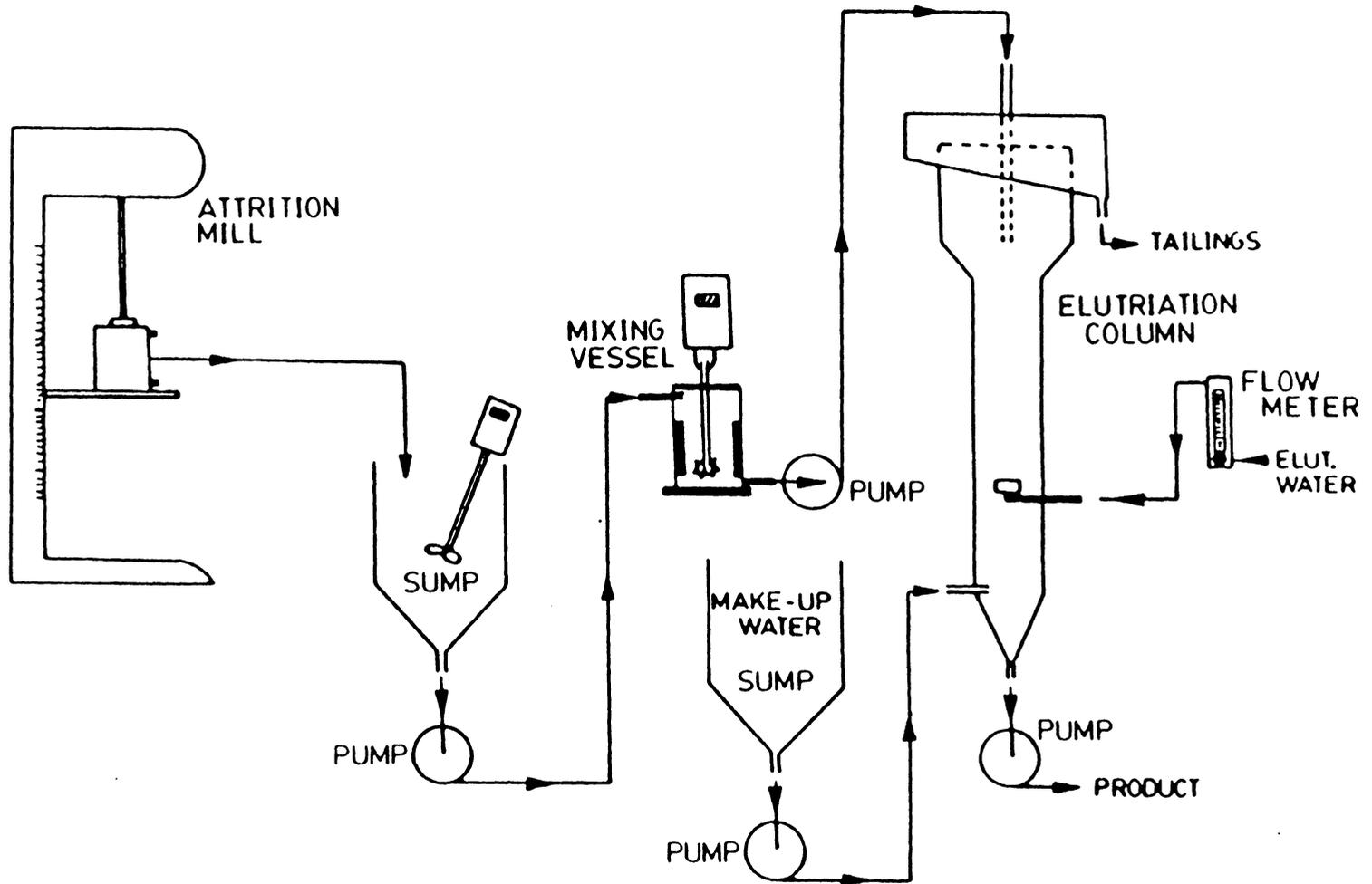
Figure 4.1 Flowsheet for the continuous selective coagulation/elutriation process.
