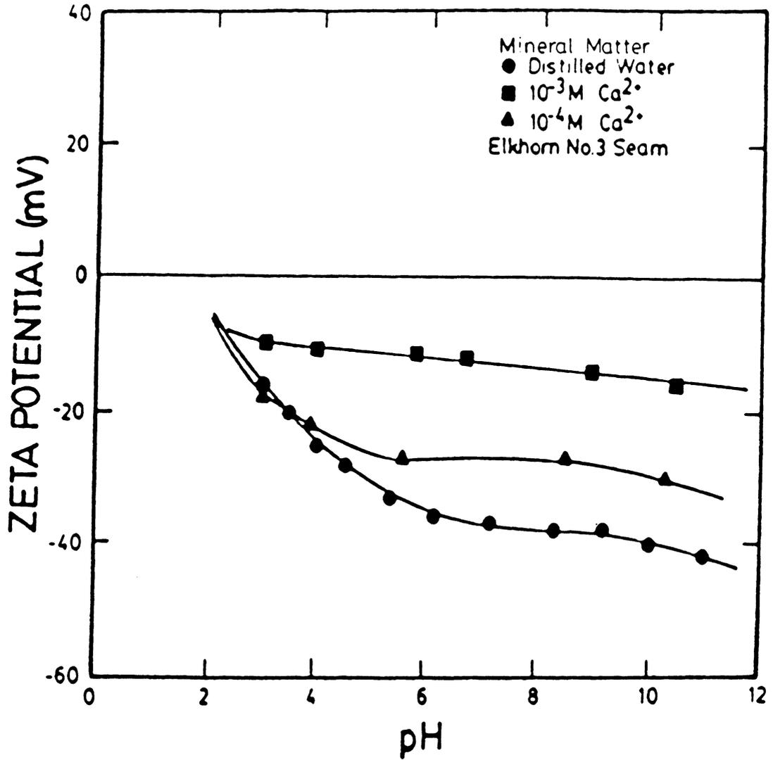
Figure 2.30 The effect of calcium additions on the zeta potentials of mineral matter.
