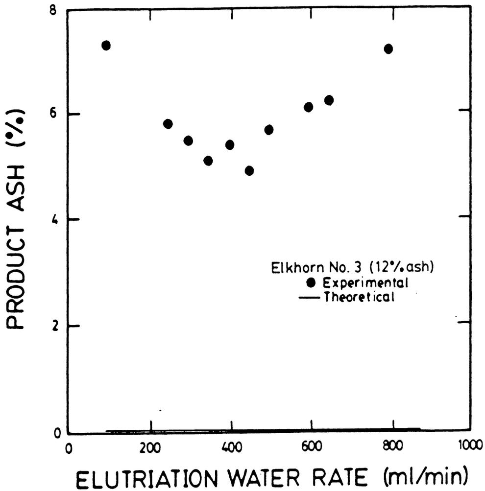
Figure 5.12 A comparison between model predictions and experimental results showing the effect of elutriation water rate on product ash percent.
