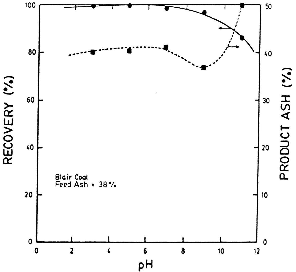
Figure 2.13 The effect of pH on coal recovery and product ash percent for the Blair coal seam containing 38.0% ash in tap water using 3 cleaning stages.
