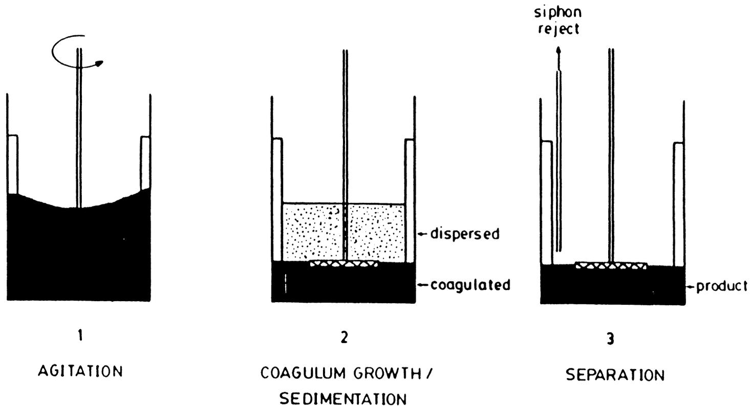
Figure 2.2 Schematic representation of the steps used in the batch-type experiments .
