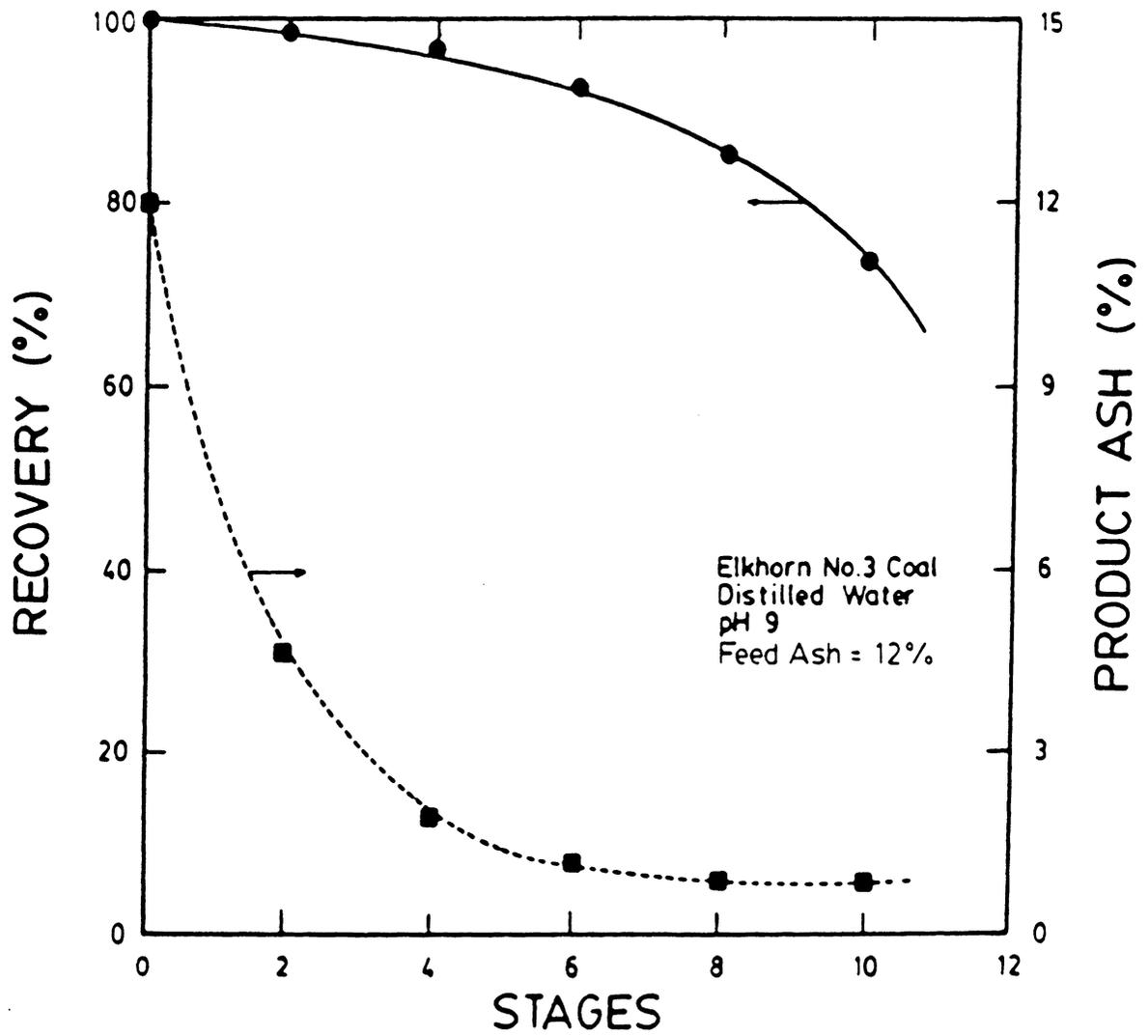
Figure 3.1 The effect of cleaning stages on recovery and product ash percent for the Elkhorn No.3 coal seam containing 12% ash.
