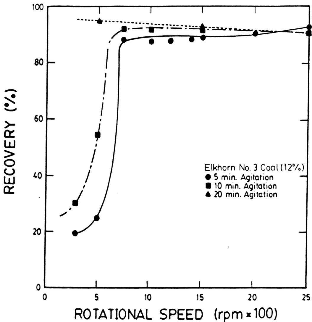
Figure 3.13 The effect of rotational speed on coal recovery for three agitation times.
