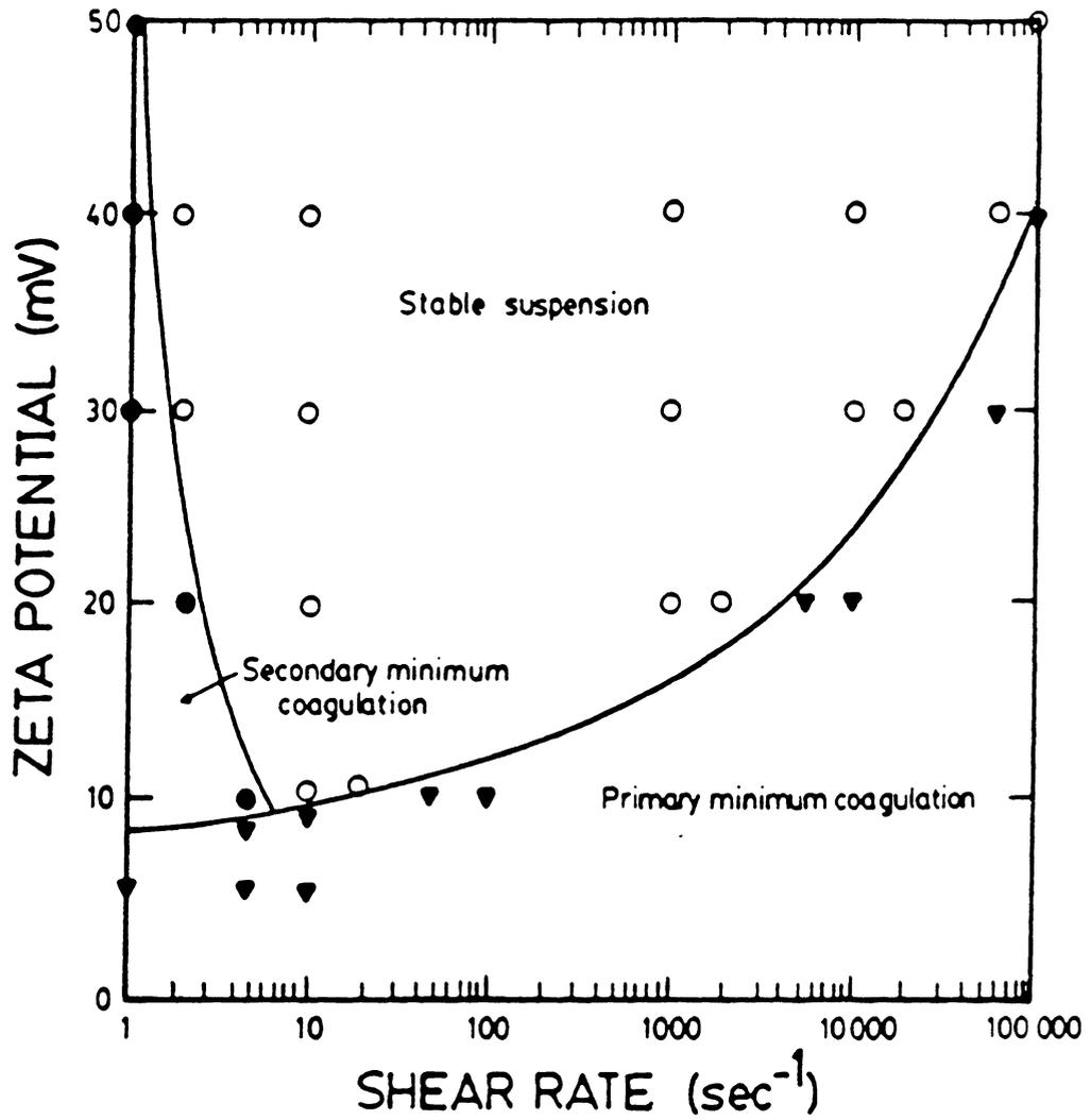
Figure 3.20 Shear coagulation domain for 1 micron particles as a function of shear rate and zeta potential (Warren, 1982).
