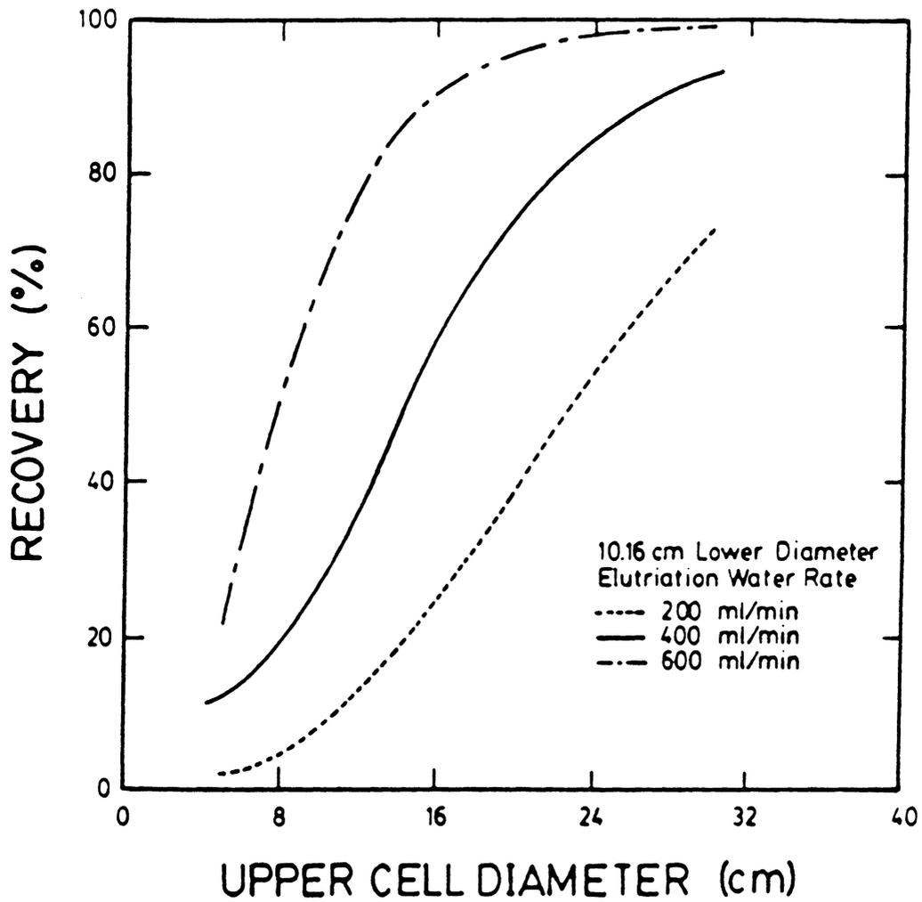
Figure 5.9 Model predictions showing the effect of upper cell diameter on coal recovery for three elutriation water rates.
