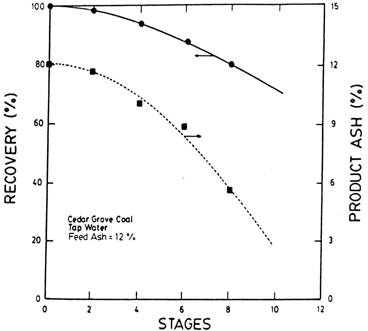
Figure 3.3 The effect of cleaning stages on recovery and product ash percent for the Upper Cedar Grove coal seam containing 12% ash.
