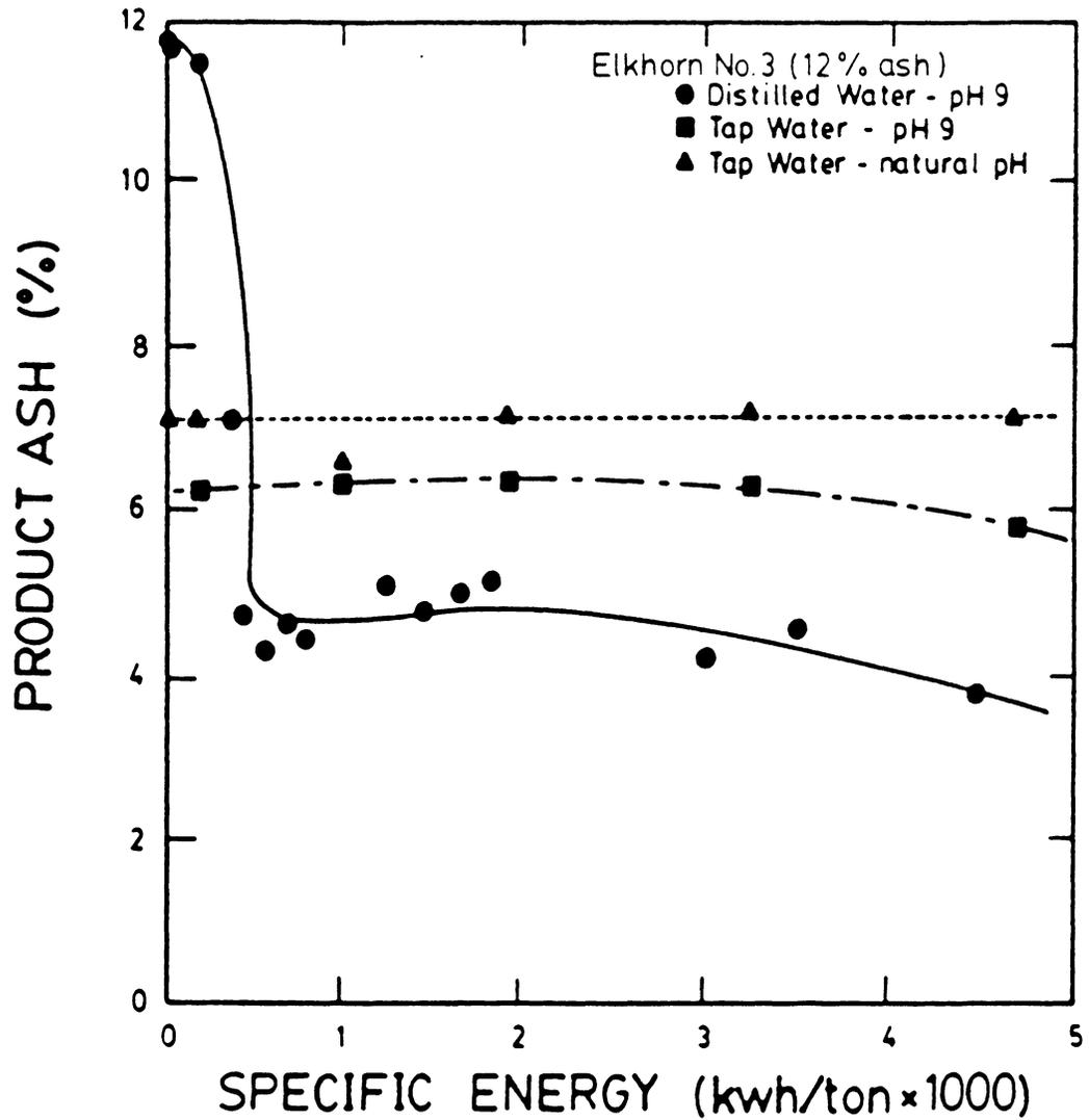
Figure 3.18 The effect of specific energy input on product ash percent for 3 media conditions; specific energy accumulated over 3 cleaning stages.
