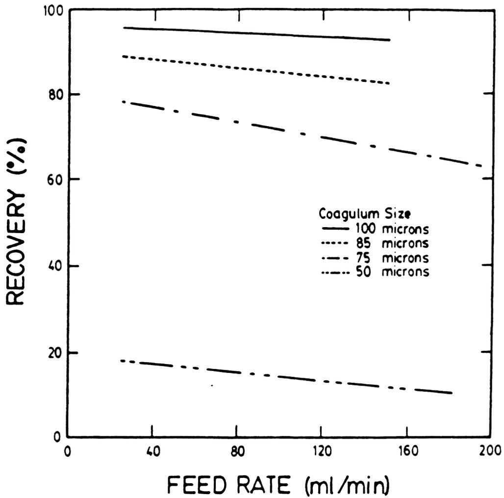
Figure 5.5 Model predictions on the effect of feed rate on coal recovery over a range of coagulum sizes.
