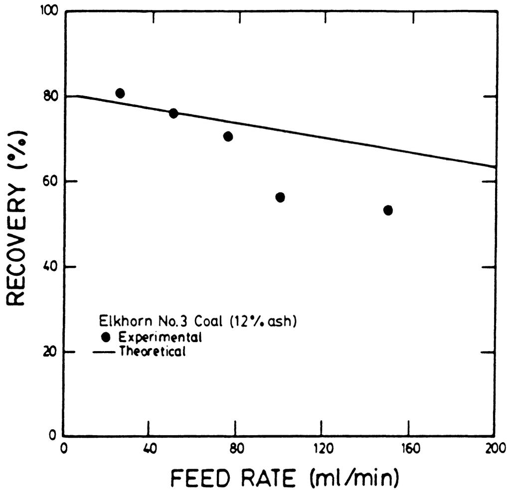
Figure 5.13 A comparison between model predictions and experimental results showing the effect of feed rate on coal recovery.
