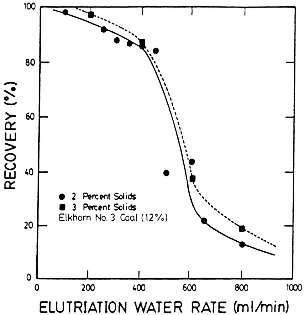
Figure 4.7 Coal recovery versus elutriation water rate curves for 2 percent solids.
