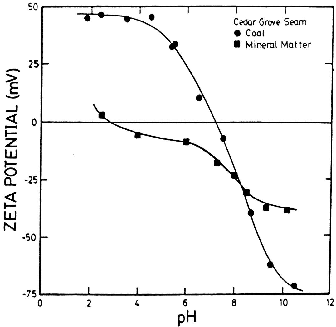
Figure 2.26 Zeta potential measurements over a range in pH for Upper Cedar Grove coal and mineral matter in distilled water.
