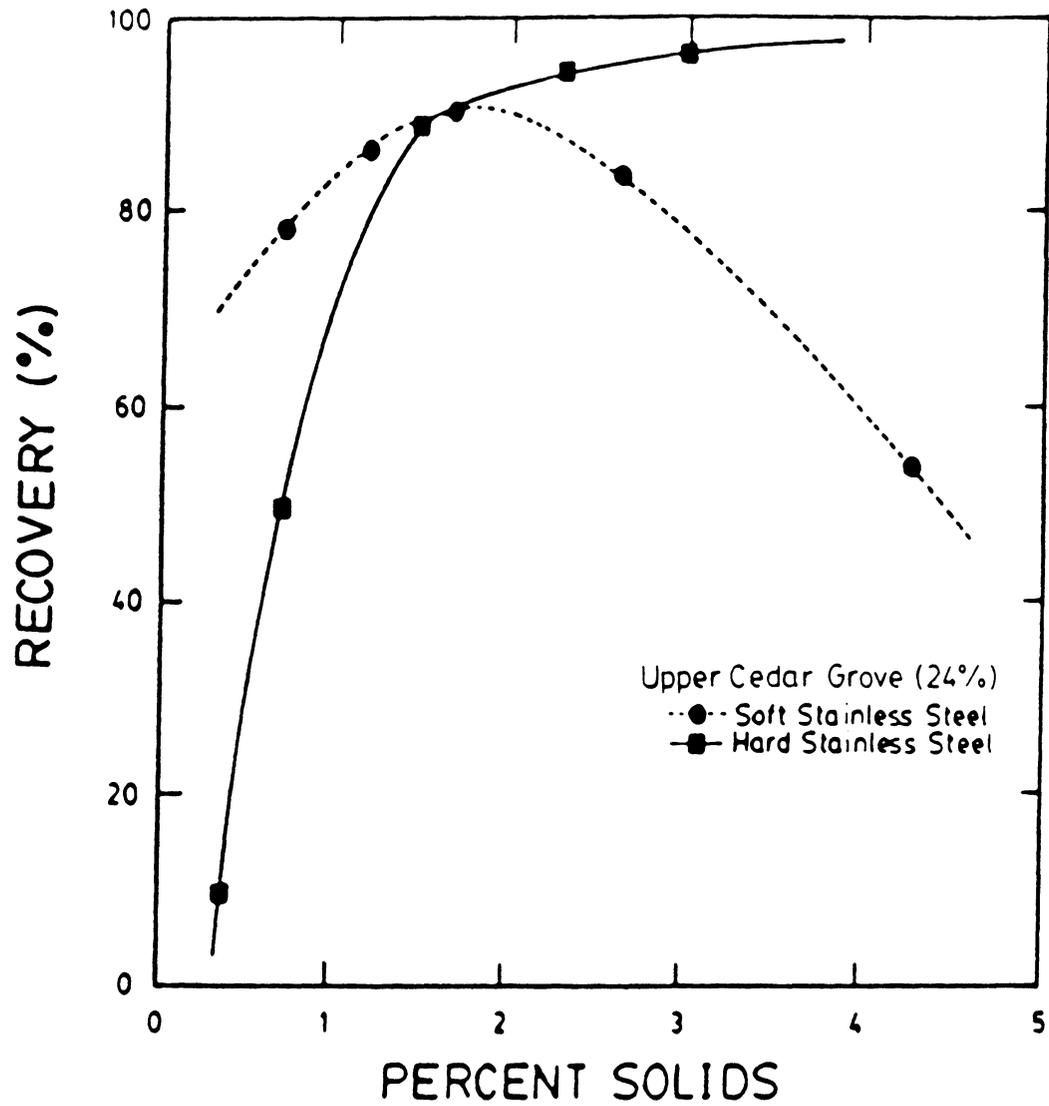
Figure 2.21 The effect of the grinding environment on recovery.
