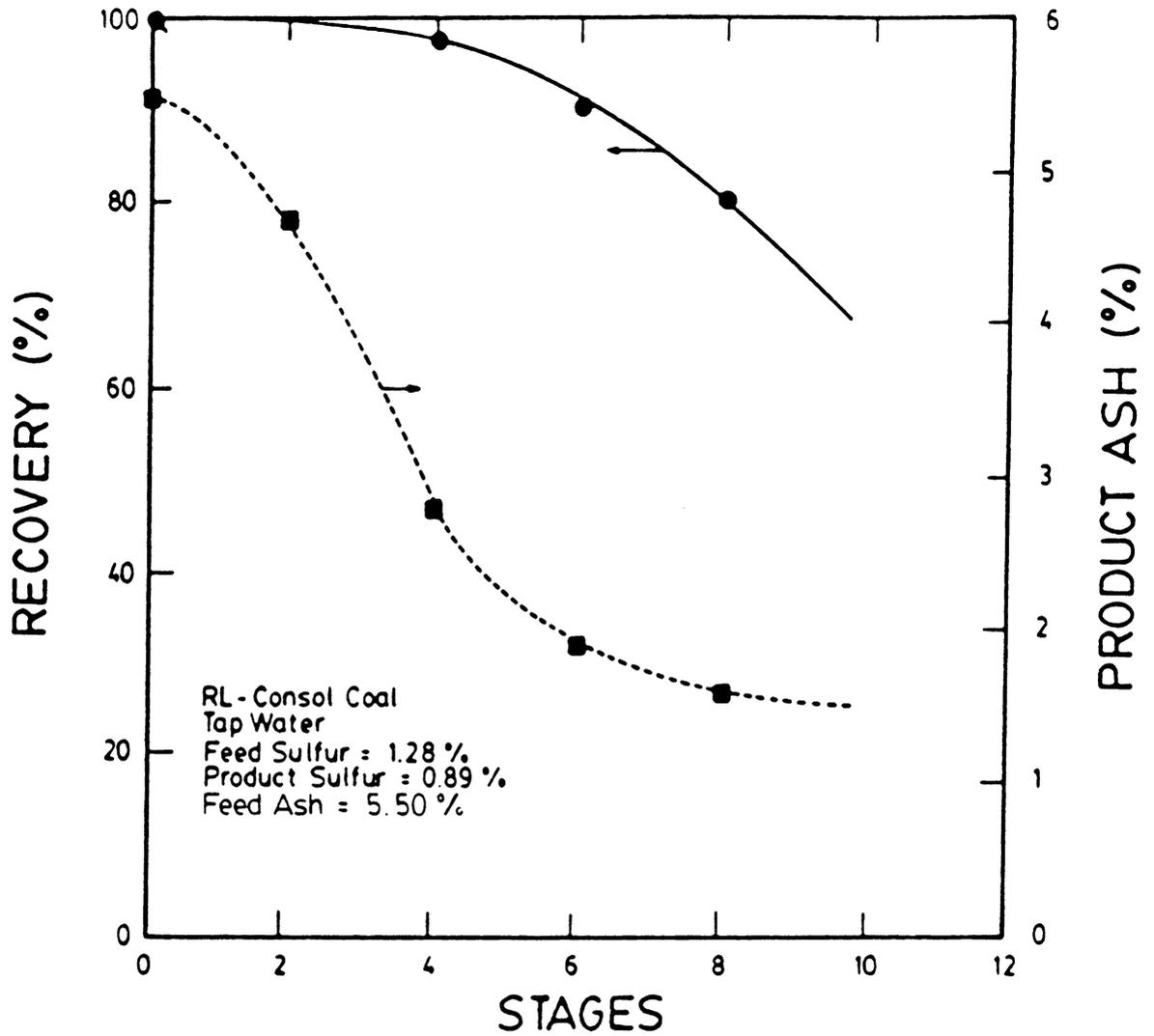
Figure 3.5 The effect of cleaning stages on recovery and product ash percent for the RL-Consol coal sample containing 5.5% ash.
