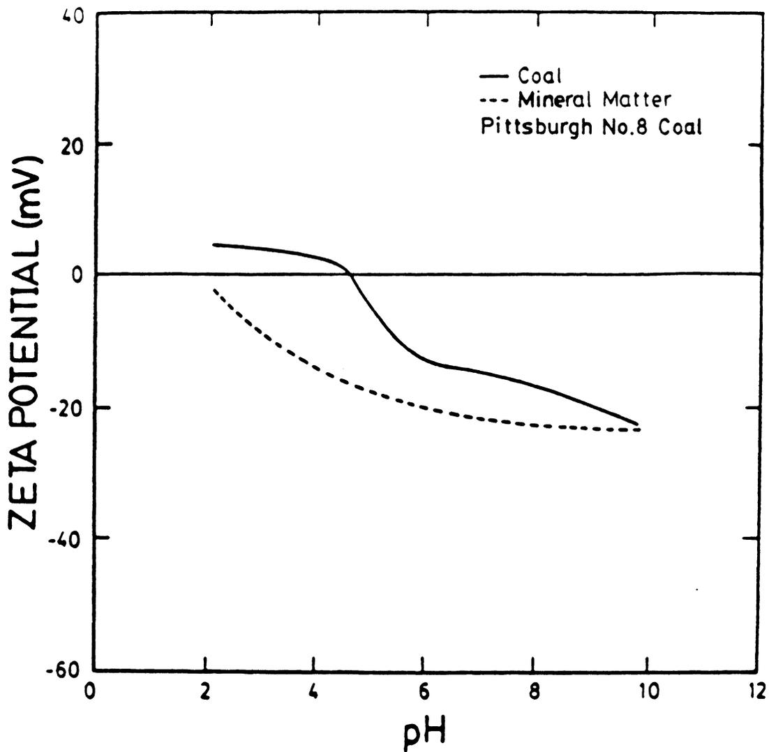
Figure 2.27 Zeta potential measurements over a range in pH for Pittsburgh No.8 coal and mineral matter in tap water.
