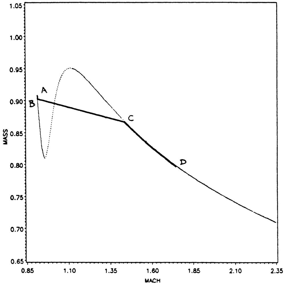
Fig.35: Projection of the trajectory on mass-velocity plane for  $P_{\max} = \infty$
