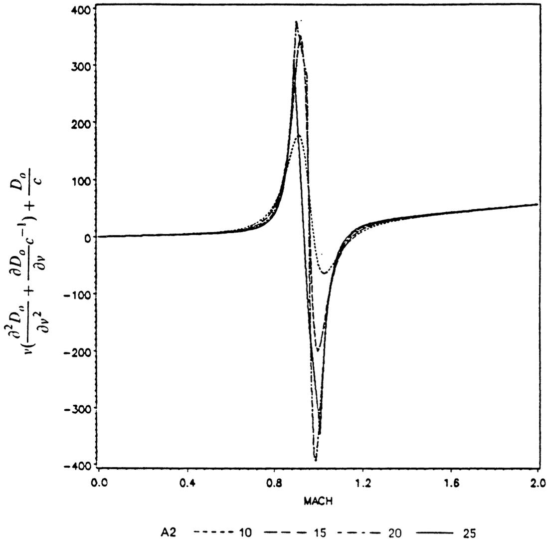
Fig.30: Variation of  $v\left(\frac{\partial^2 D_o}{\partial v^2} + \frac{\partial D_o}{\partial v} c^{-1}\right) + \frac{D_o}{c}$  with Mach number
