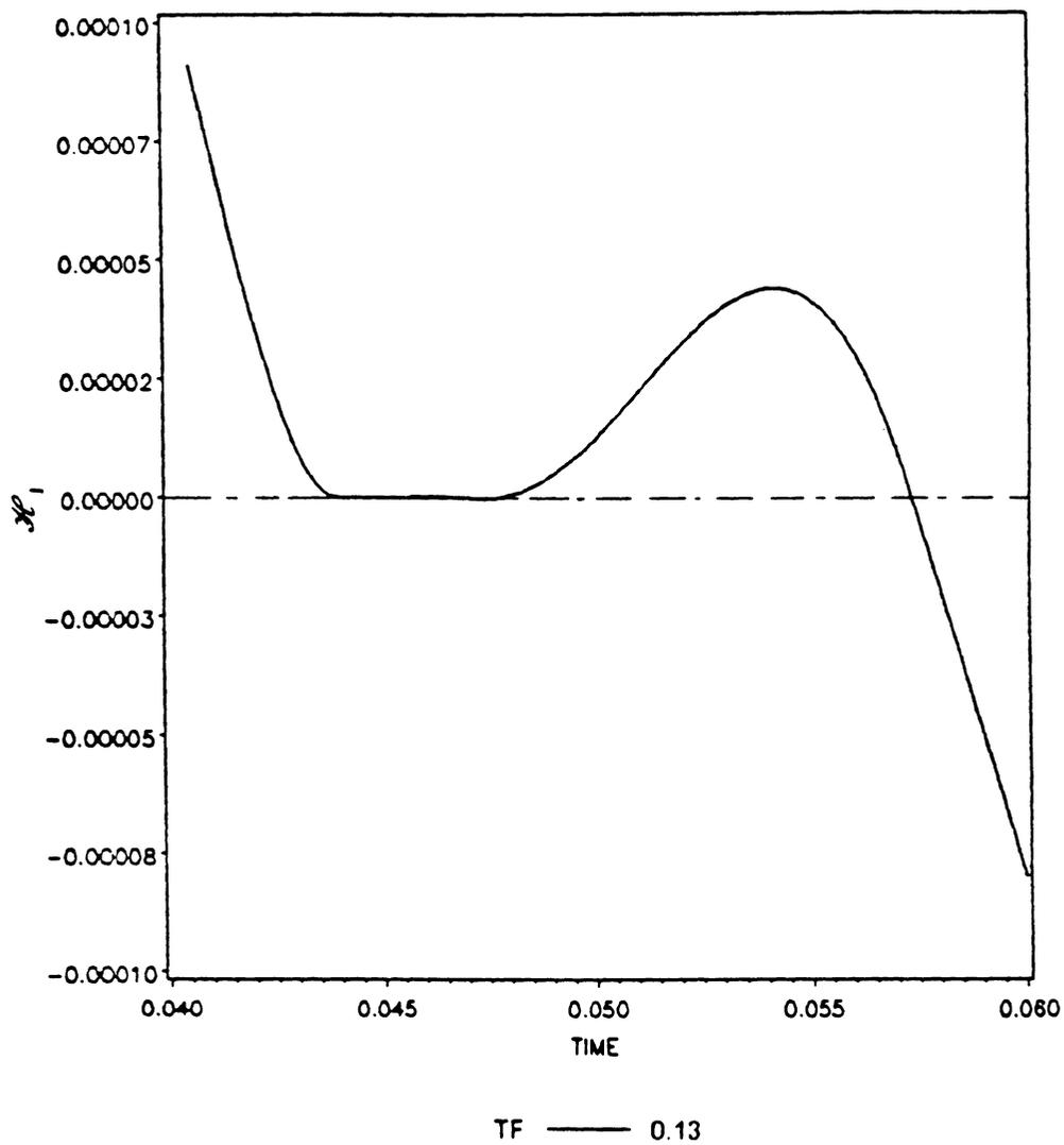
**Fig.19:** Switching function  $\mathcal{H}_1$  vs. time for full-singular-full-coast sequence
