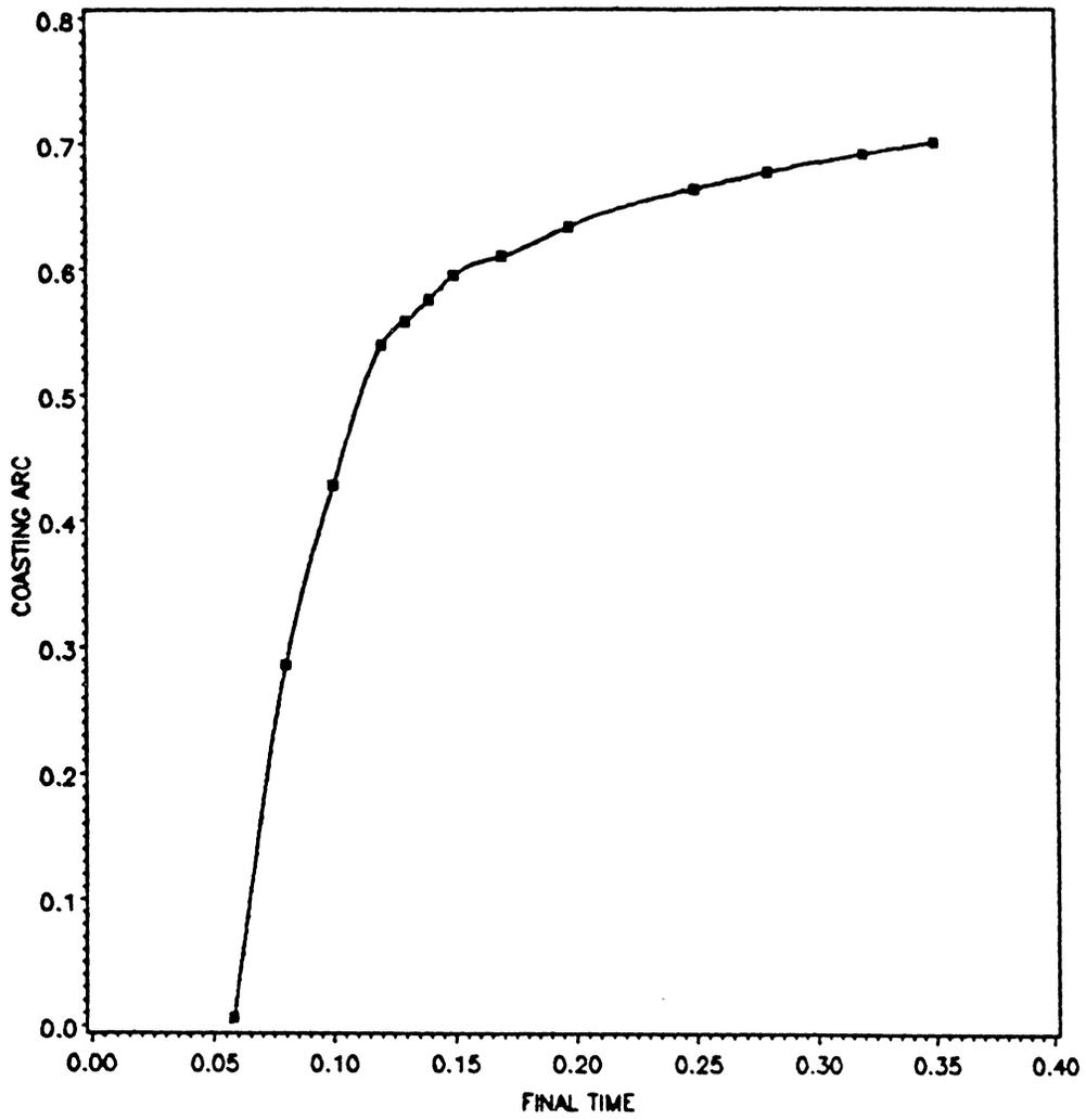
Fig.7: Variation of zero-thrust subarc with final time
