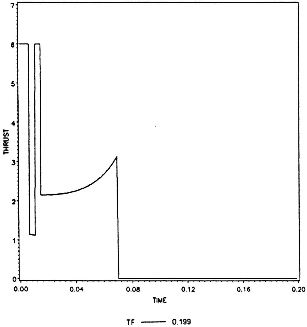
Fig.40: Variation of thrust  $P$  with time for  $P_{max} = 6$
