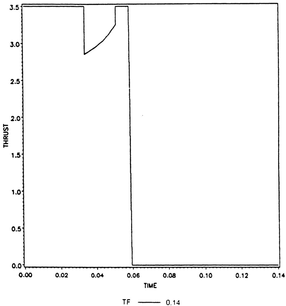
**Fig.12:** Variation of thrust P with time for full-singular-full-coast sequence
