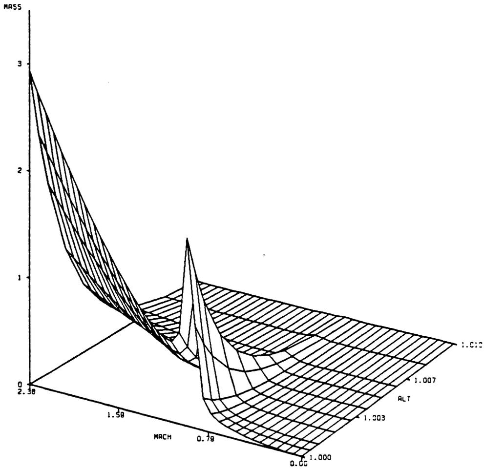
**Fig.31:** Singular surface for Mach dependent drag coefficient
