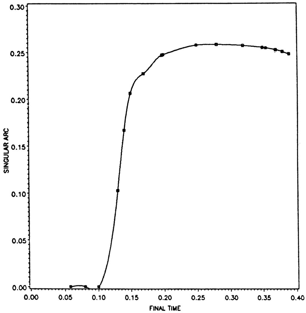
**Fig.6:** Variation of singular-thrust subarc with final time
