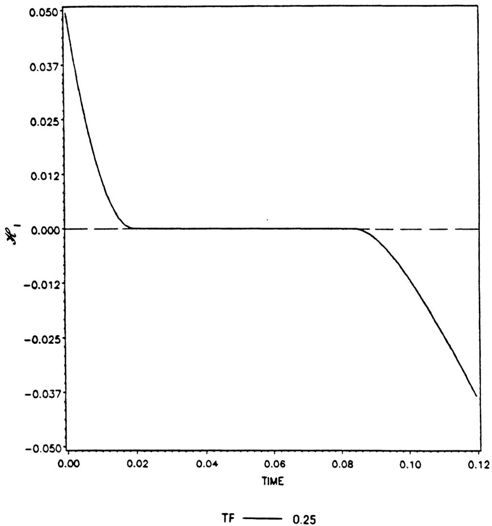
Fig.20: Switching function  $\mathcal{H}_1$  vs. time for full-singular-coast sequence
