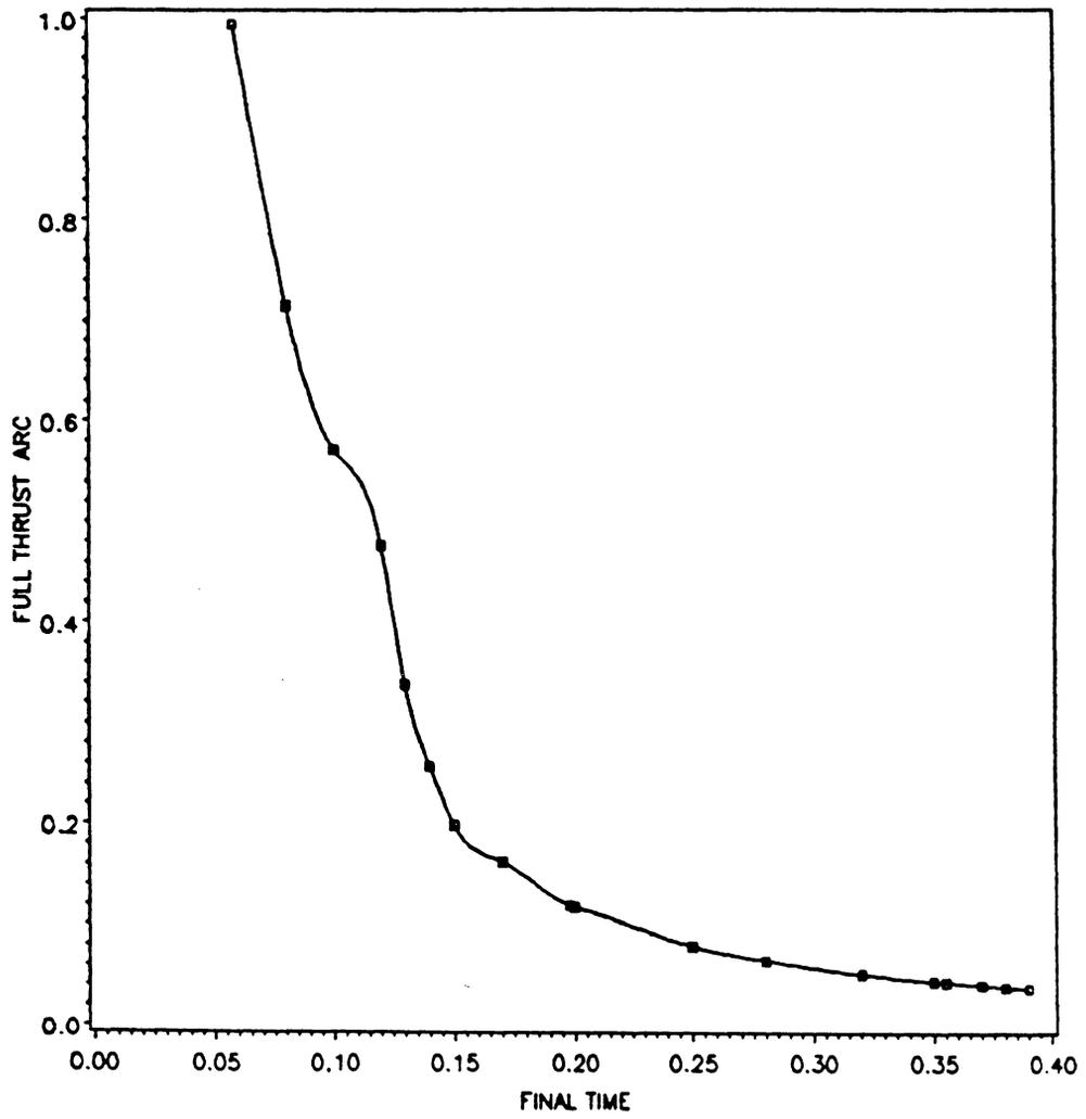
Fig.5: Variation of full-thrust subarc with final time
