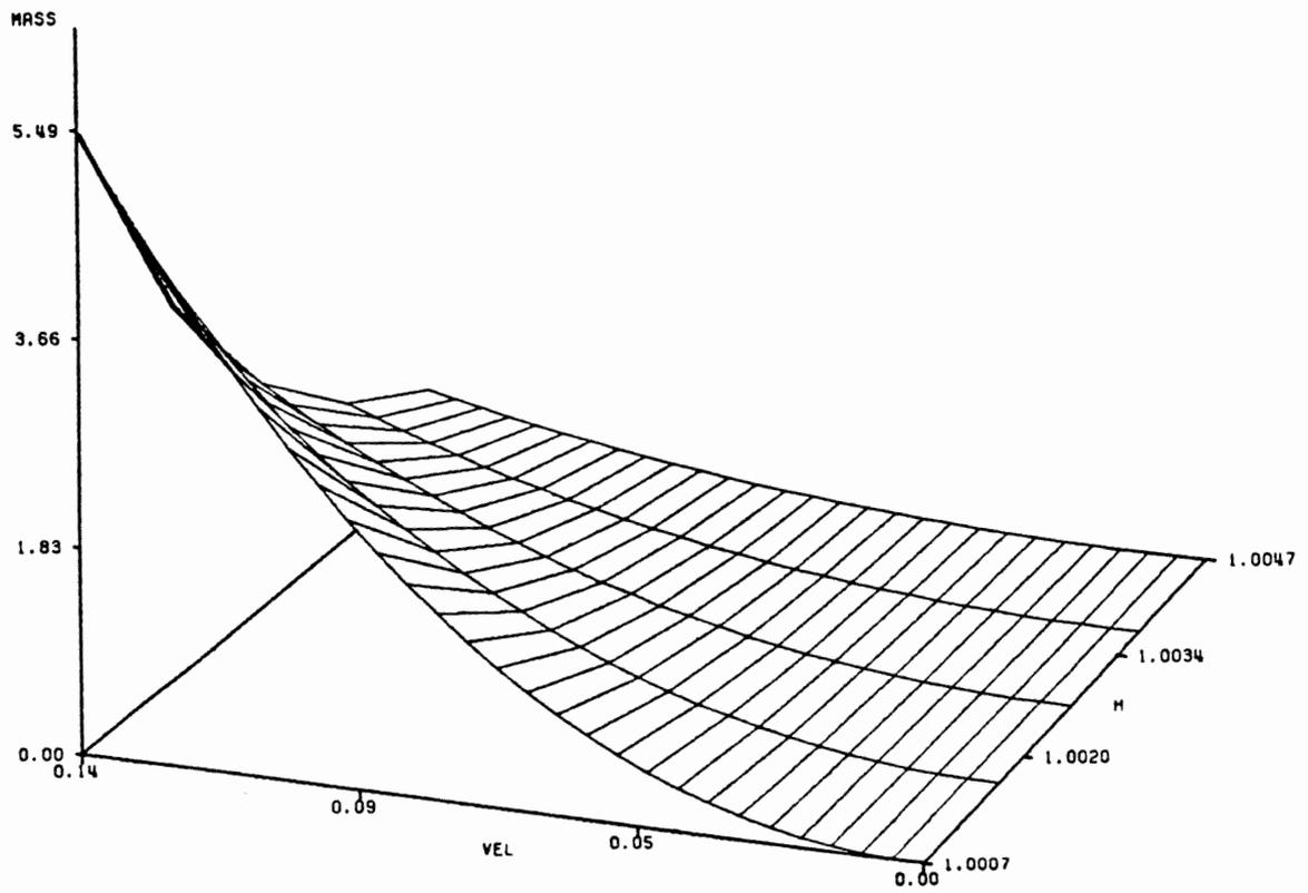
Fig.1: Singular surface in  $h, m, v$  space
