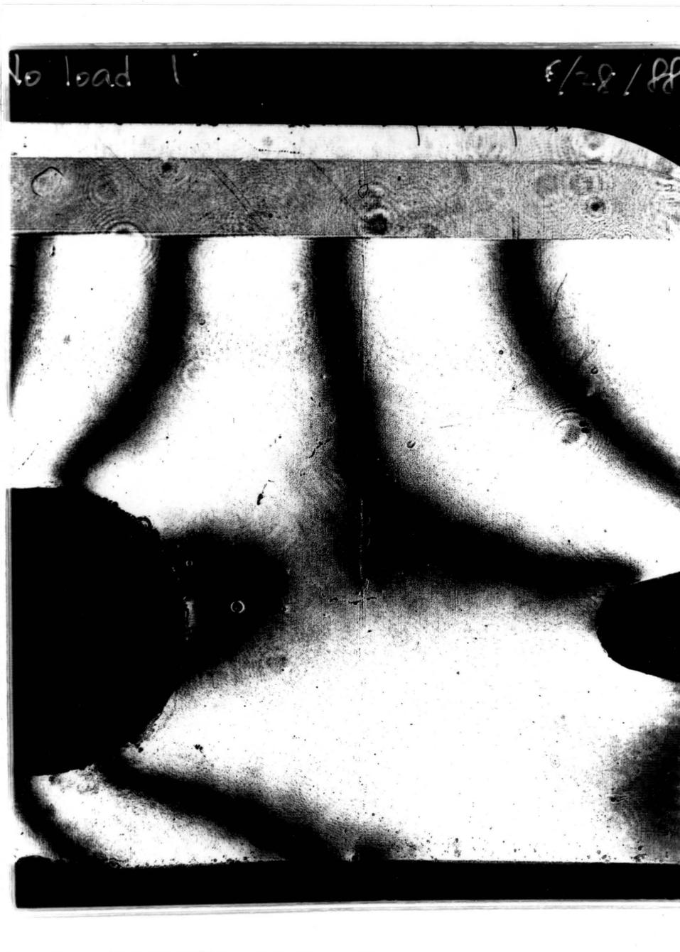
Fig. 5.2 No-Load Horizontal (X) Displacement Field
