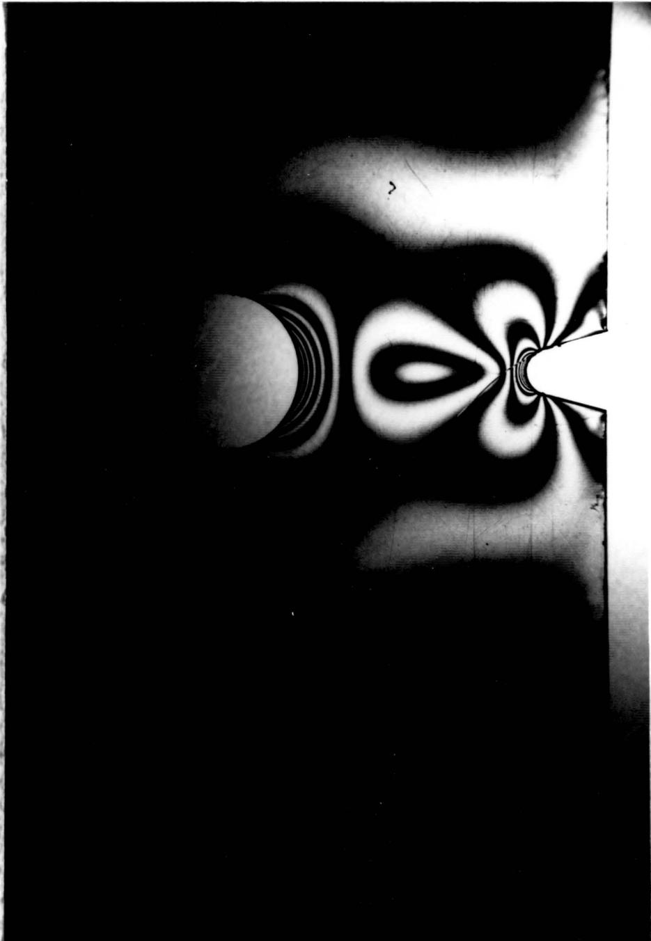
Fig. 6.1 Photoelastic Stress Contour Axial/Bending Load
