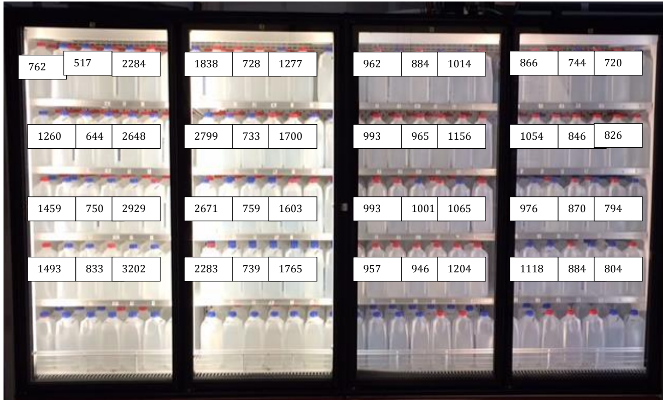
Figure 20. The front loading, closed-door retail case with fluorescent (3500K, left two doors) and LED (right two doors; 3500K on left and center positions 4000K on far right position) lighting that was used for the study. Light intensity readings (lux) are represented for each position throughout the retail case. Treatment packages were not placed on the bottom row of the case due to lower light intensity and increased light intensity variability in these locations. Treatment packages were randomly placed throughout the front row of this case.
