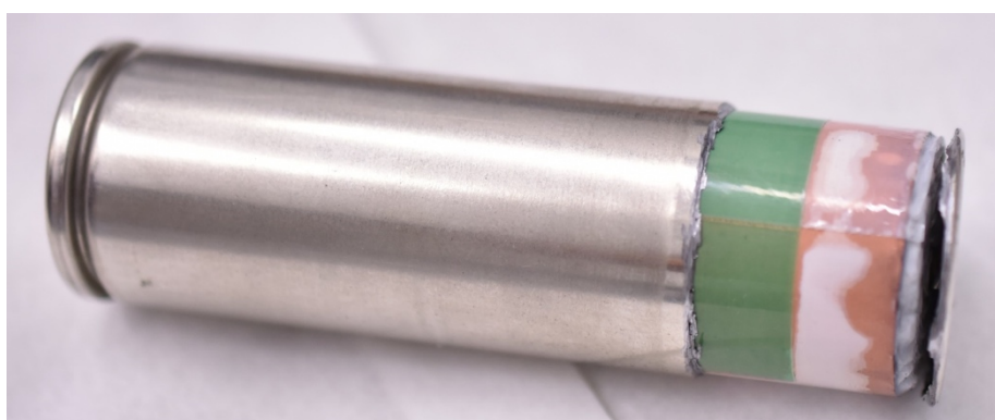
Figure 3.10: Battery core removed from cell case after cathode cutting completed
