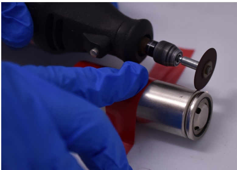
Figure 3.11: Dremel tool used to cut the anode section of the battery case
