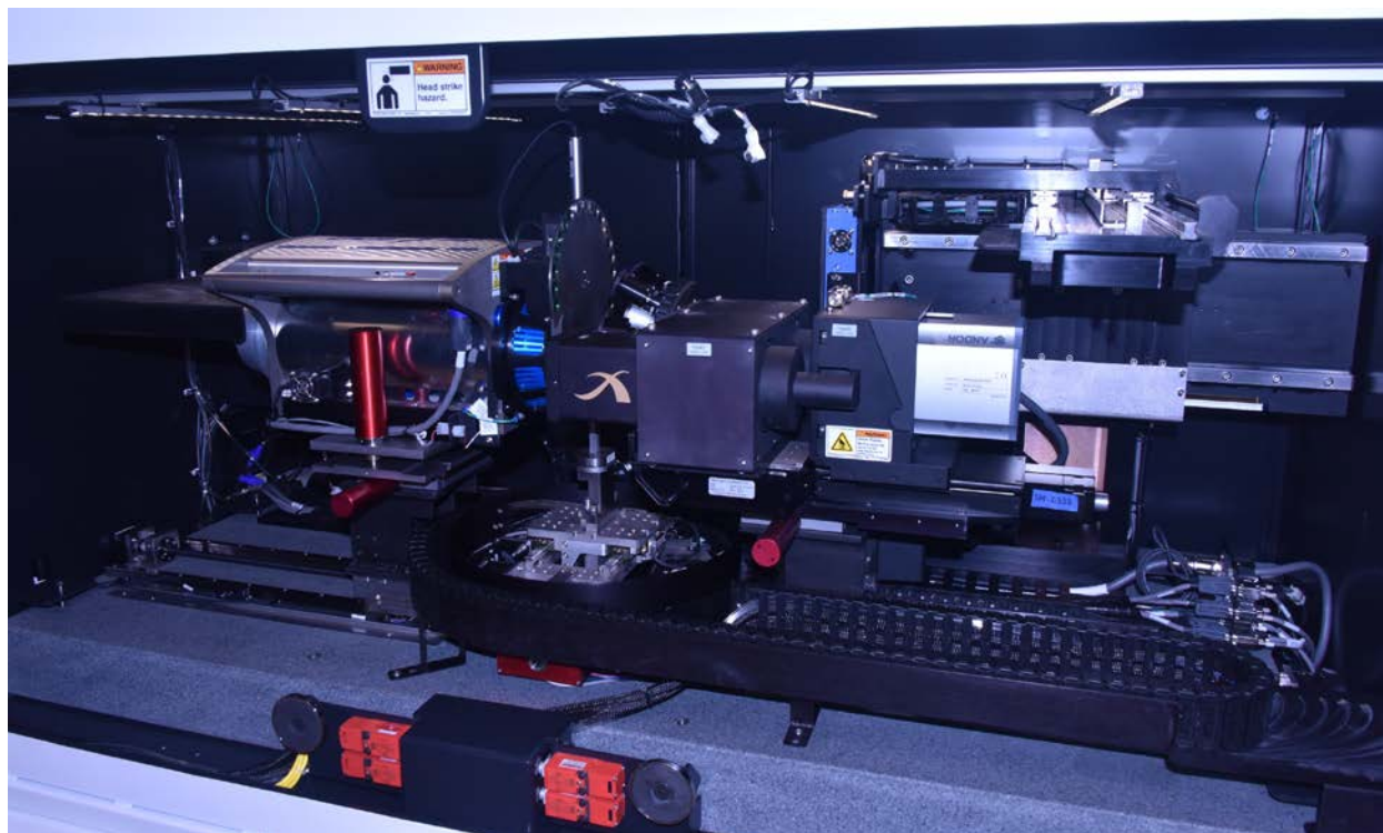
Figure 3.16: Interior of Zeiss Xradia 520 Versa with the X-ray source on the left, sample stage in the middle, and detector on the right
