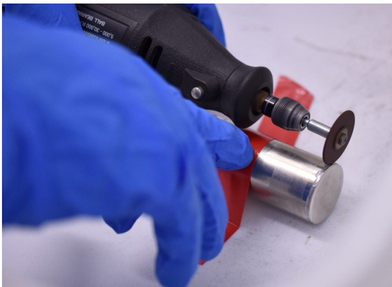
Figure 3.9: Dremel cutter is used to open the battery case to expose the cathode electrical connections
