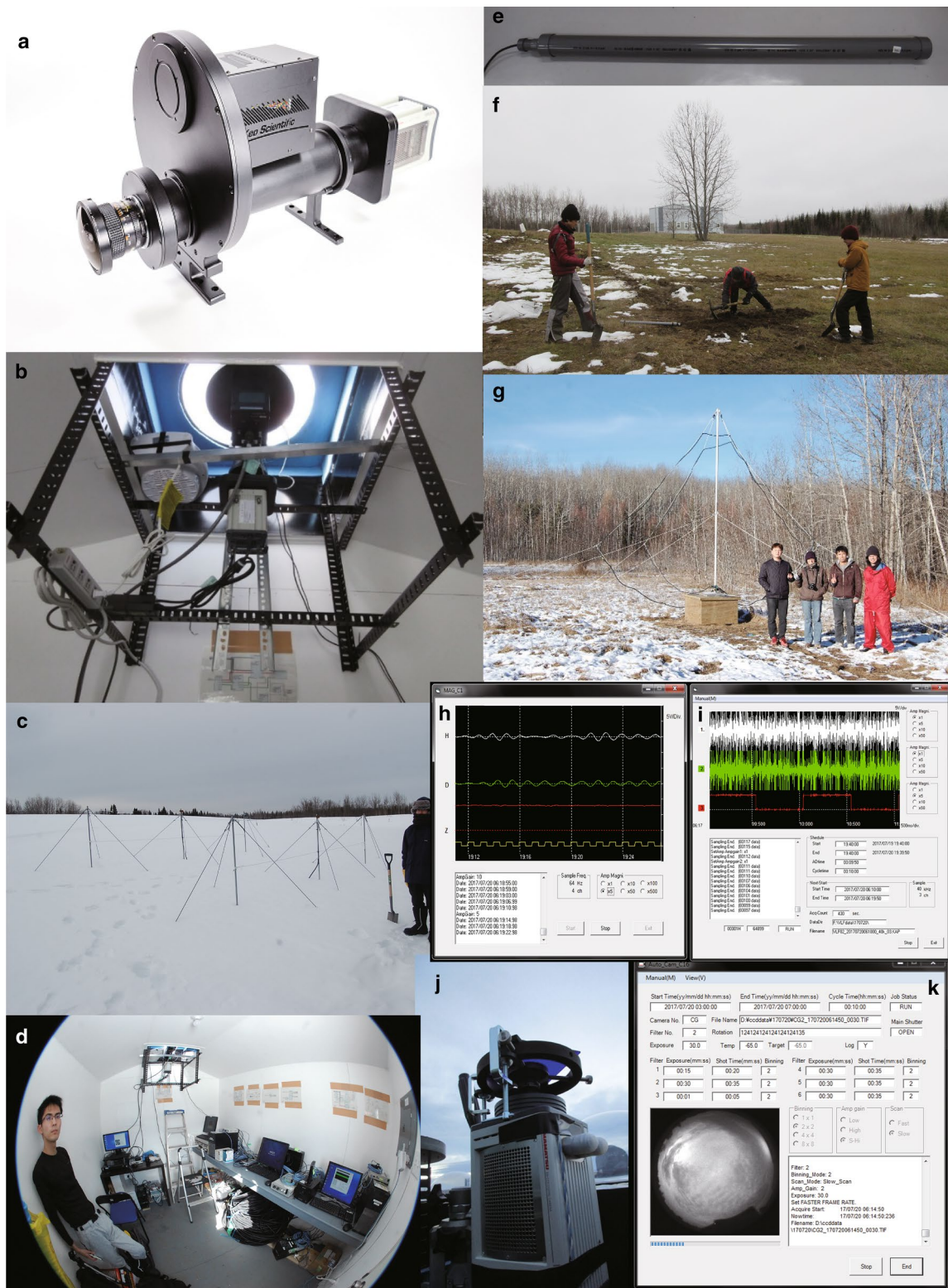
Fig. 2 Photographs of the five instruments installed by the PING project for a, b all-sky airglow/aurora camera at KAP, c riometer at KAP, d inside of container house at KAP, e, f induction magnetometer at ATH, g loop antenna at ATH, h PC window for magnetometer and riometer, i PC window for loop antenna, j EMCCD camera at ATH, and k PC window for all-sky airglow/aurora imager
