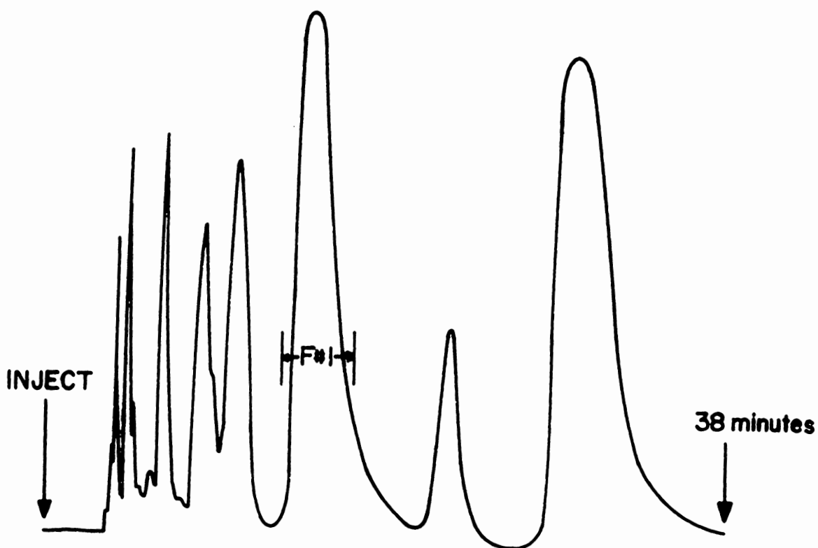
Figure 16. Preparative HPLC separation of 3,4-di(p-bromophenyl)-1,2,5-triphenylcyclopentadien-1-methyl ether (F #1). Column: 0.5 in. O.D. x 20 cm x 9.9 mm I.D.; packing material: 10 \mu m Lichrosorb SI-100; mobile phase: 0.08% ethyl acetate in n -hexane at 9.6 ml/min; detector: UV at 254 nm and 0.08 ABS attenuation; sample size: 502 \mu l.
