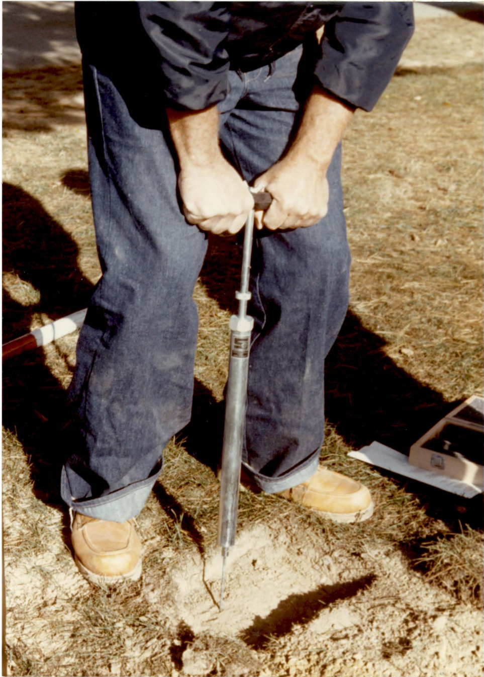
Figure 11: Proctor penetrometer used for testing soil compaction.
