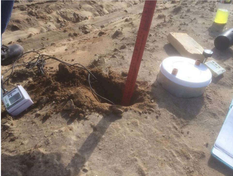
**Figure 3: In-Field Soil Respiration Measurement Set Up.**
