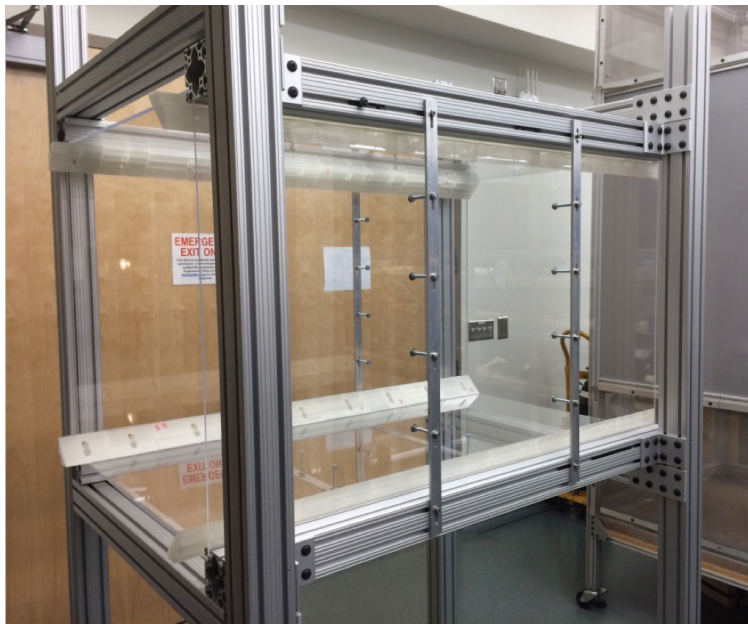
Figure 4.6: Acrylic-wall enclosed test section with corner gussets
