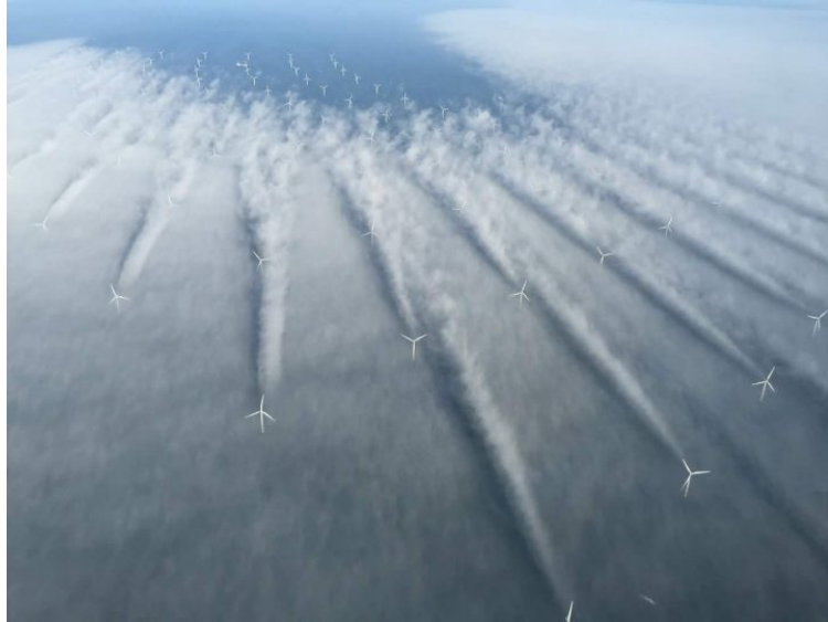
Figure 2.1: Horns Rev wind farm illustrating unsteady inflow from upstream turbines [27]
