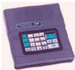
Figure 1: A typical phone alarm system allows growers to remotely monitor house conditions.
