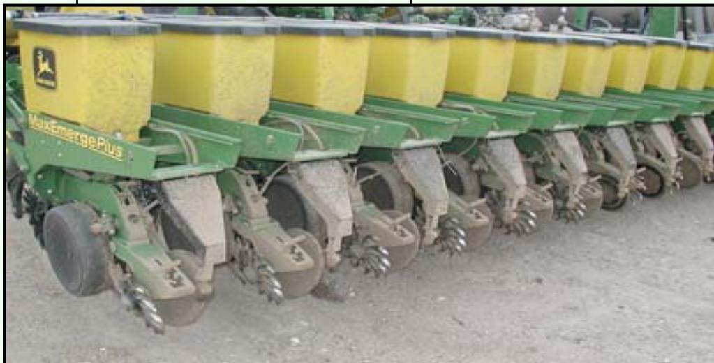
This planter uses one spoked wheel on each row to close the soil around the seed and one standard press wheel to firm the soil while providing depth control. This reduces the aggressiveness of spoked closing wheels to reduce over-drying of the seed zone.
