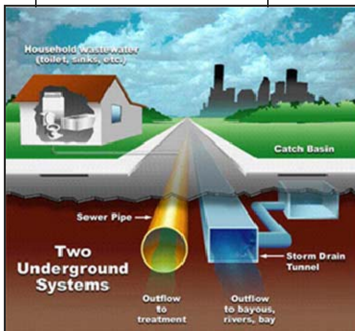
Stormwater System, Illustrating Outflows are Untreated
