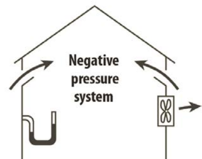
Figure 2. Negative pressure system with inlets and an exhaust fan.
