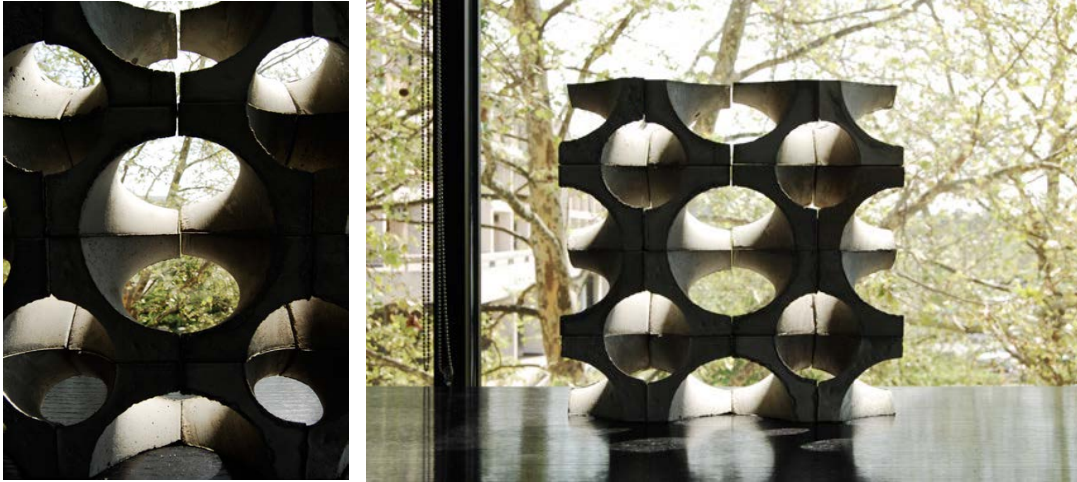
Figure 154: Self-continuous concrete module designed in transLAB
