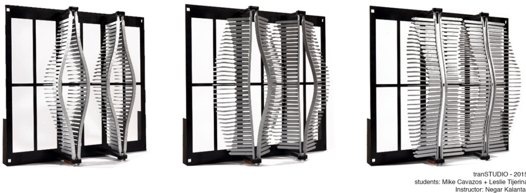
Figure 144: Transformable shading system. The Pedagogy of Motion endeavors to create a better understanding how an exploratory concept of motion can be codified to suit different technical, economic, and cultural considerations.
