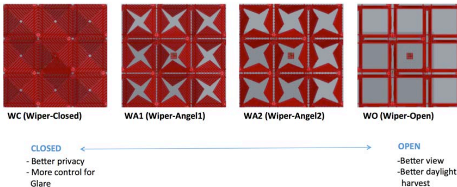
Figure 92: Scheme 1: Wiper Rotation.
