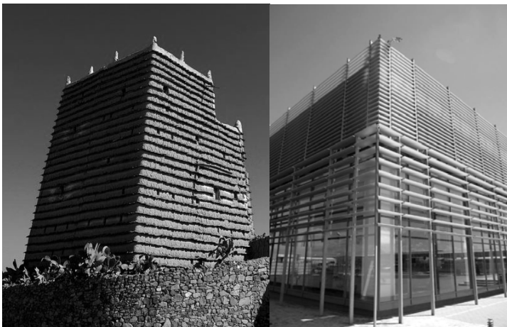
Figure 3: The same shading concept in old and new buildings. Shading devices are the layer that can accept most of adaptive concepts. They can control light, glare, view, air quality and the amount of heat transfer.
