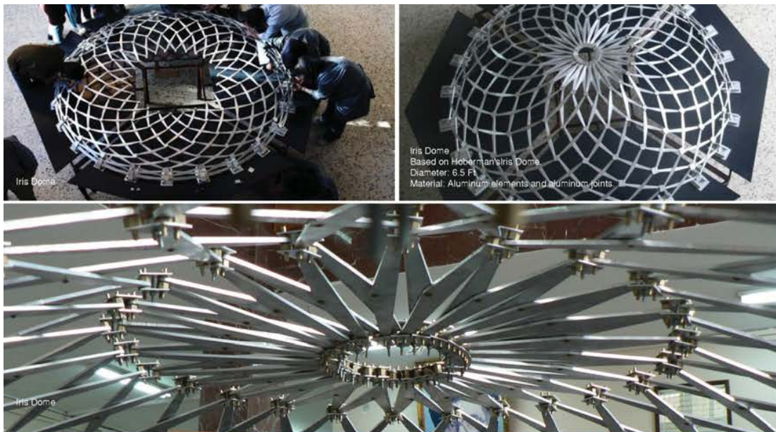
Figure 34: Deployable Iris Dome
