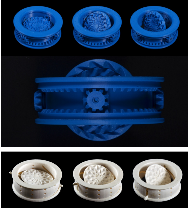
Figure 131: In the AURA design process, 3D printing opened up new design opportunities. Thinking 3-dimensionally and integrating elements are two main advantages.
