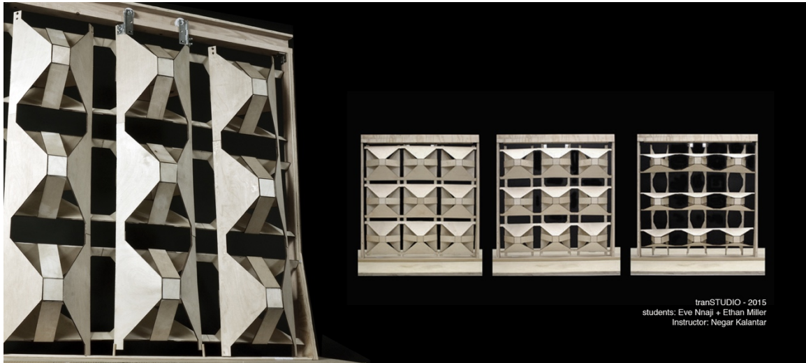
Figure 157: A transformable shading system. The fold system flattens out and covers the entire opening. Elastic fabrics were laminated in between two layers of veneer to provide a hardware-free hinge for the fold system.
