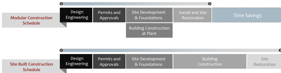
Figure 4.5: Time savings in modular construction, adopted from the Permanent Modular Construction-2011 Annual Report
