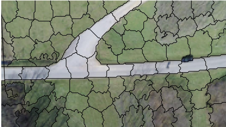
Figure 74. Example of SLIC Superpixel Segmentation of Road Image
