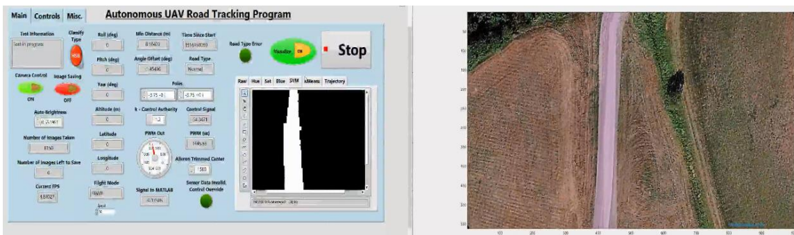
Figure 37. HIL Simulation Segmentation – As seen in the LabVIEW GUI, the road pixels (white) are correctly classified from the surrounding land pixels (black)
