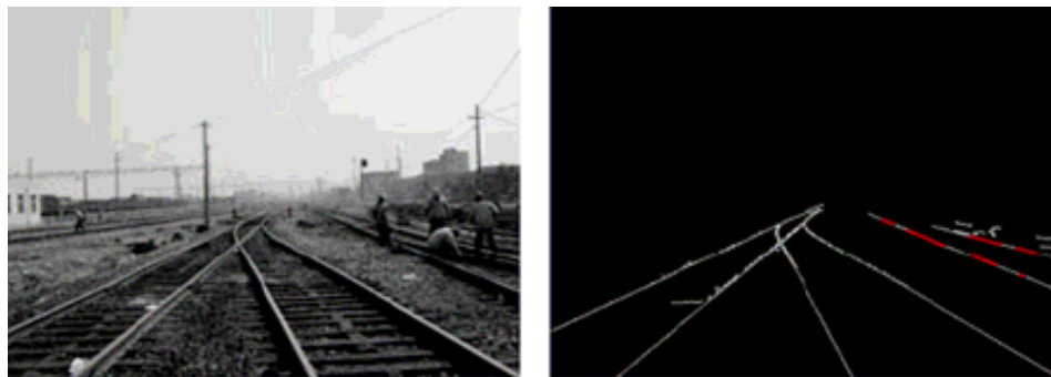
Figure 46. Hough Transform Detecting Railroad Obstacles
