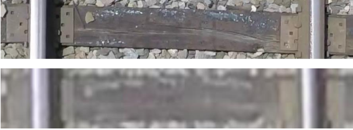
Figure 8. Effect of GSD on Image Quality - Diagram showing sharp details in a railroad tie image taken at a low GSD value (top) as opposed to the poor details in a high GSD value image (bottom)
