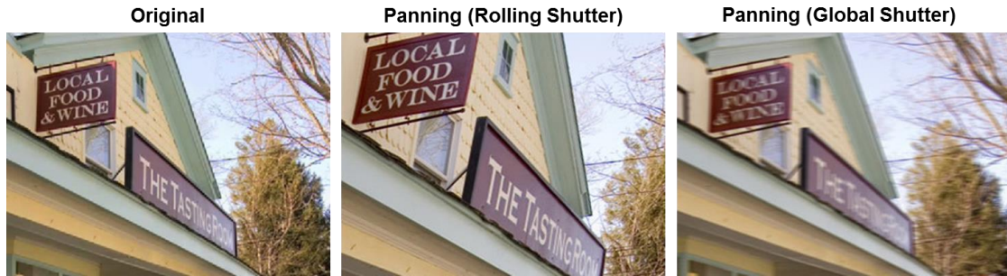
Figure 9. Consequences of Rolling and Global Shutters for Moving Cameras
