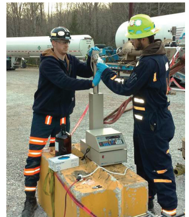
Team researchers Kyle Louk (l) and Joseph Amante inject tracer gas into an existing well in Tennessee.
