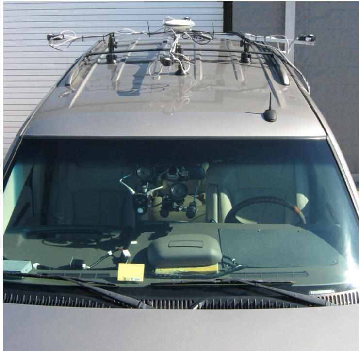
Figure 4. Photo. RLMMS components mounted on and inside a vehicle.
