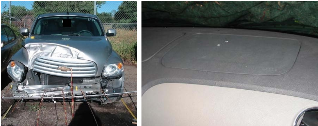
Figure 62. NASS Case Number 2010-75-160, Chevrolet HHR During Inspection Showing Damage to the Right Front of the Vehicle ( left ) and Instrument Panel Showing the Airbag Did Not Deploy ( right )
