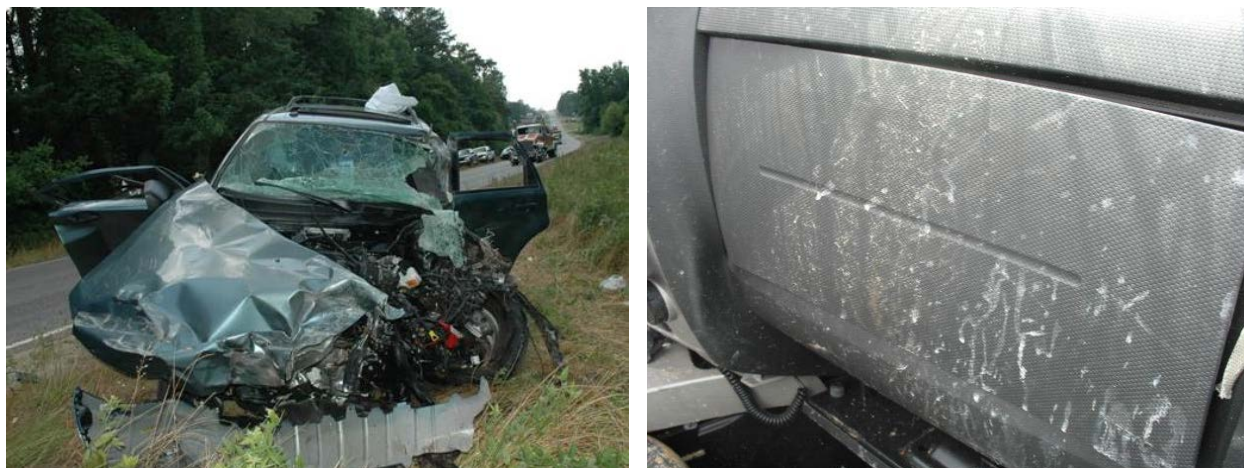
Figure 64. NASS Case Number 2011-48-111, Ford Escape at the Scene Showing Damage to the Front of the Vehicle ( left ) and the Instrument Panel for the Suppressed Passenger Airbag ( right )
