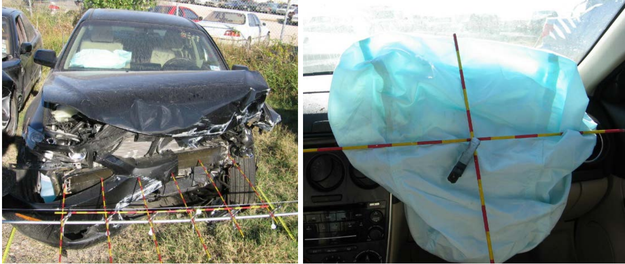
Figure 57. NASS Case Number 2006-50-135 Vehicle 1, Mazda 6 During Investigation Showing More Damage to the Driver's Side ( left ) and the Passenger Airbag ( right )
