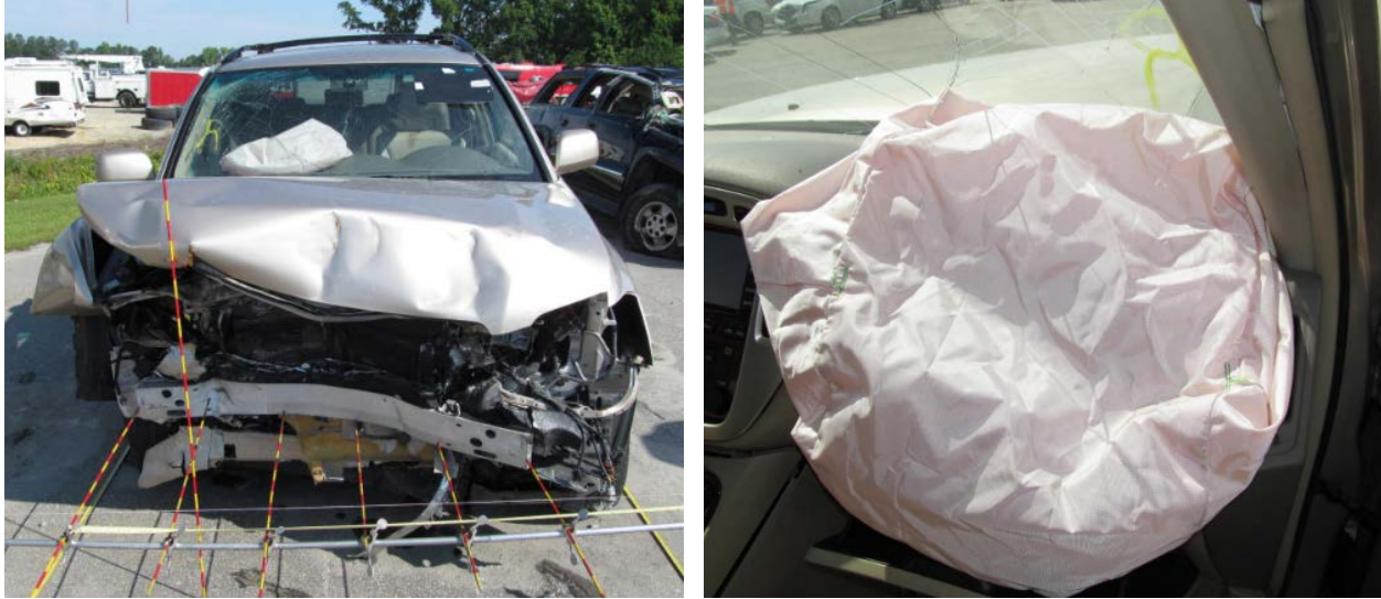
Figure 61. NASS Case Number 2012-43-102 Vehicle 1, Showing Damage to Front of Toyota Highlander ( left ) and Top-Mounted Passenger Airbag ( right )
