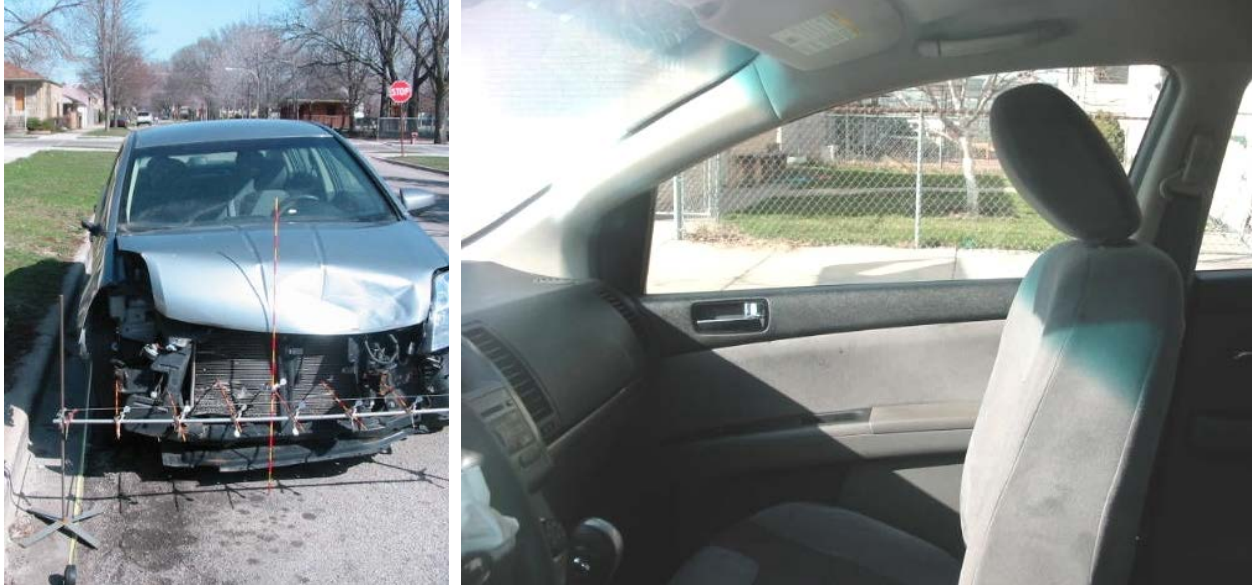
Figure 59. NASS Case Number 2010-72-027 Vehicle 2 Showing the Damage to the Front of the Vehicle ( left ) and the RFP Seat Fully Forward, No Airbag Deployment ( right )
