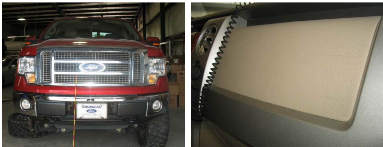
Figure 69. NASS Case Number 2012-48-80, Ford F-150 Pickup during Investigation which Occurred After Repairs Began ( left ) and the Passenger Mid-Instrument Panel Mounted Airbag ( right )
