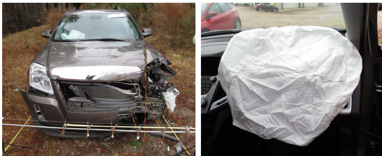
Figure 74. NASS Case Number 2012-43-208, GMC Terrain During Investigation Showing More Damage to the Front Driver's Side ( left ) and the Instrument Panel Showing a Deployed Passenger Airbag ( right )
