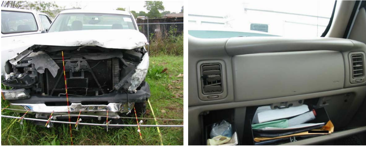
Figure 65. NASS Case Number 2009-49-161, Chevrolet C/K-Series Pickup During Investigation Showing More Damage to the Driver's Side ( left ) and the Instrument Panel Showing a Suppressed Passenger Airbag ( right )
