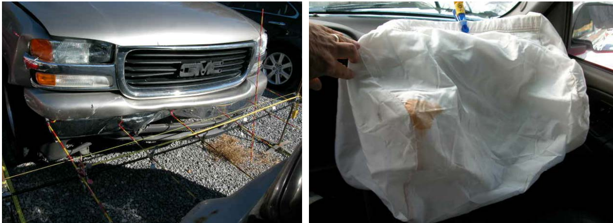
Figure 73. NASS Case Number 2011-48-206, GMC Yukon During Investigation Showing Damage to the Front ( left ) and the Instrument Panel Showing a Deployed Passenger Airbag ( right )
