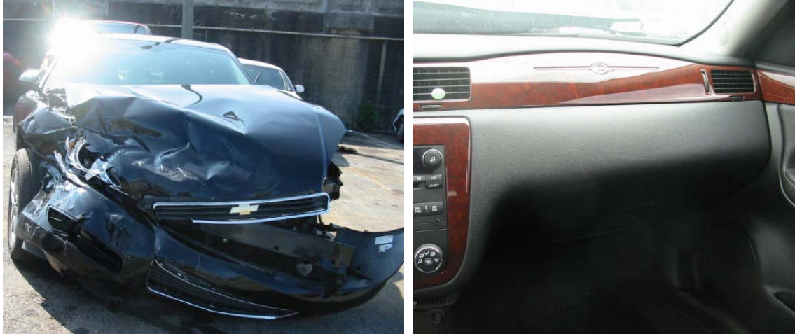
Figure 71. NASS Case Number 2010-45-166, Chevrolet Impala During Investigation Showing More Damage to the Passenger’s Side ( left ) and the Instrument Panel Showing a Suppressed Passenger Airbag ( right )
