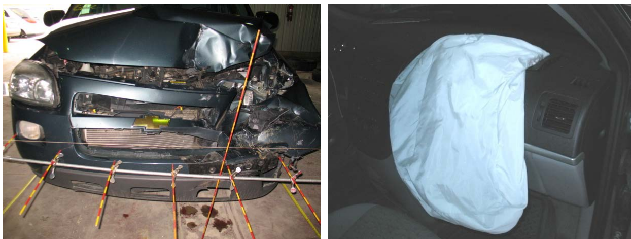
Figure 72. NASS Case Number 2010-12-78, Chevrolet Uplander During Investigation Showing More Damage to the Driver's Side ( left ) and the Instrument Panel Showing a Deployed Passenger Airbag ( right )
