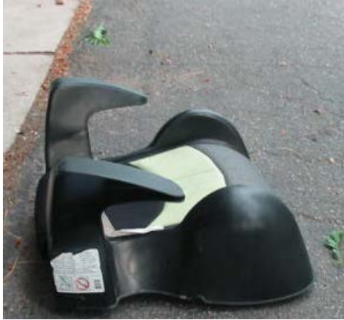
Figure 63. Cosco Ambassador Belt Positioning Booster Seat Used in NASS Case Number 2010-75-160 by a 7 year old RFP in Front of an Advanced Airbag that Suppressed
