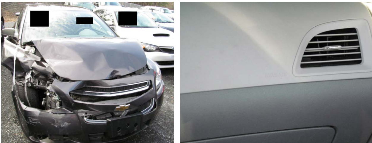
Figure 70. NASS Case Number 2012-4-92, Chevrolet Malibu During Investigation Showing More Damage to the Passenger's Side ( left ) and the Instrument Panel Showing a Suppressed Passenger Airbag ( right )
