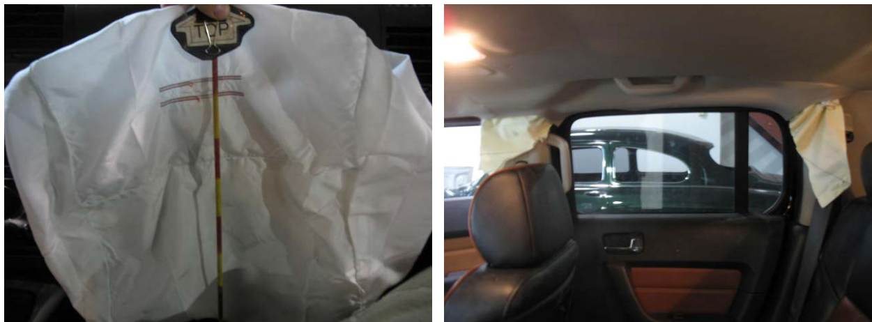
Figure 67. NASS Case Number 2010-75-081, Hummer H3 Interior Showing Passenger Airbag ( left ) and Roof Rail Airbags for the Front & Rear Passengers ( right )
