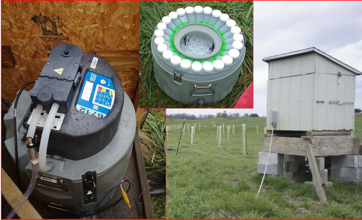
Figure 25. ISCO Automatic Sampler used for sampling storm events. Hut constructed to house the sampler shown on right.
