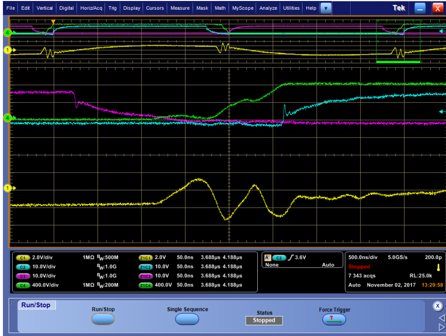
Figure 4.33. Zoomed in CLLC converter waveform under 5 kW load (forward mode) for (1) I_p (10 A/div), (2) V_{GS, s4} , (3) V_{GS, s2} , and (4) V_{ds, s2} .
