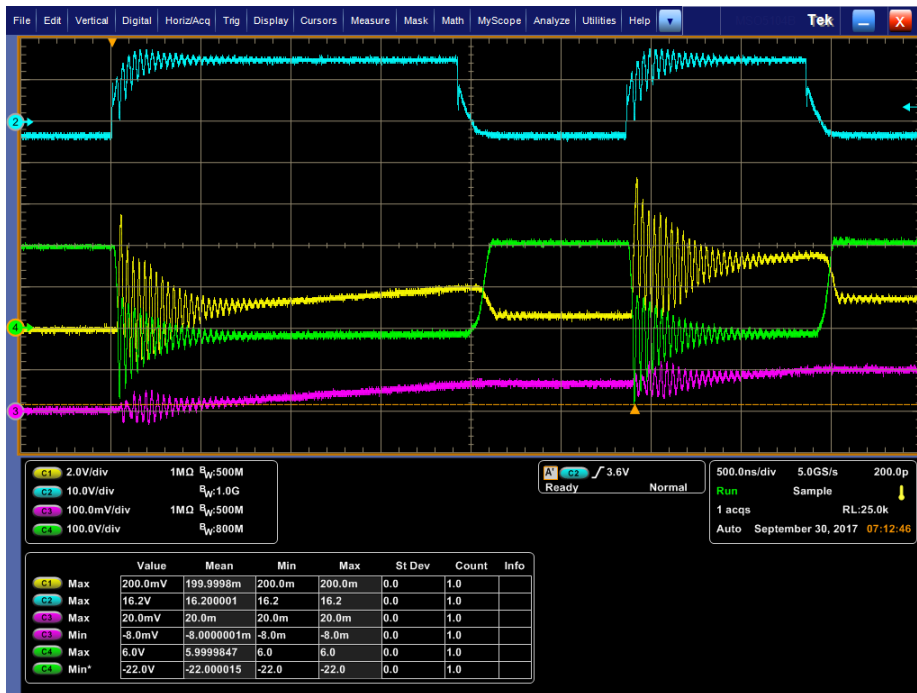
Figure 4.8. DPT waveforms for C3M0010090K with 3\Omega external gate resistance and 200 V DC bus for (1) I_{D, BOT} (10 A/div), (2) V_{GS, BOT} , (3) I_L (10 A/div), and (4) V_{DS, BOT} .
