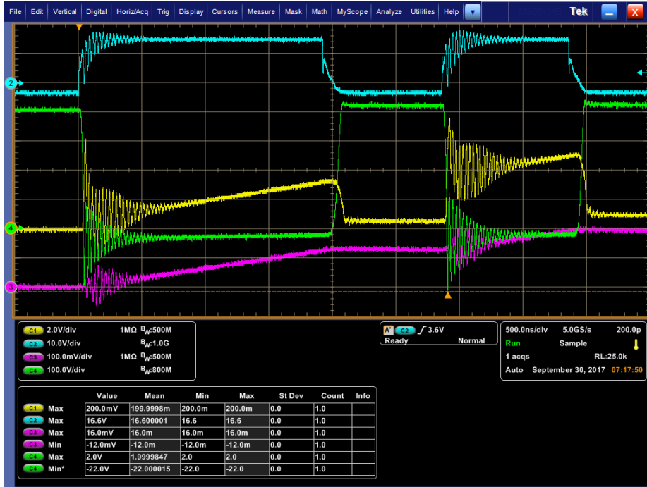
Figure 4.9. DPT waveforms for C3M0010090K with 3\Omega external gate resistance and 400 V DC bus for (1) I_{D, BOT} (10 A/div), (2) V_{GS, BOT} , (3) I_L (10 A/div), and (4) V_{DS, BOT} .
