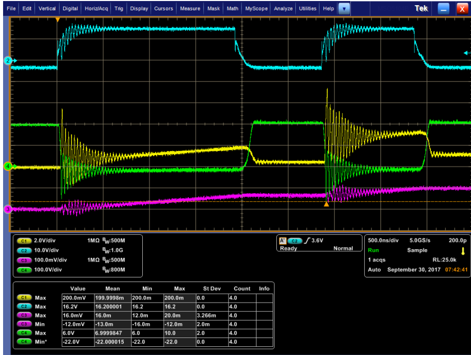
Figure 4.11. DPT waveforms for C3M0010090K with 4\Omega external gate resistance and 200 V DC bus for (1) I_{D, BOT} (10 A/div), (2) V_{GS, BOT} , (3) I_L (10 A/div), and (4) V_{DS, BOT} .
