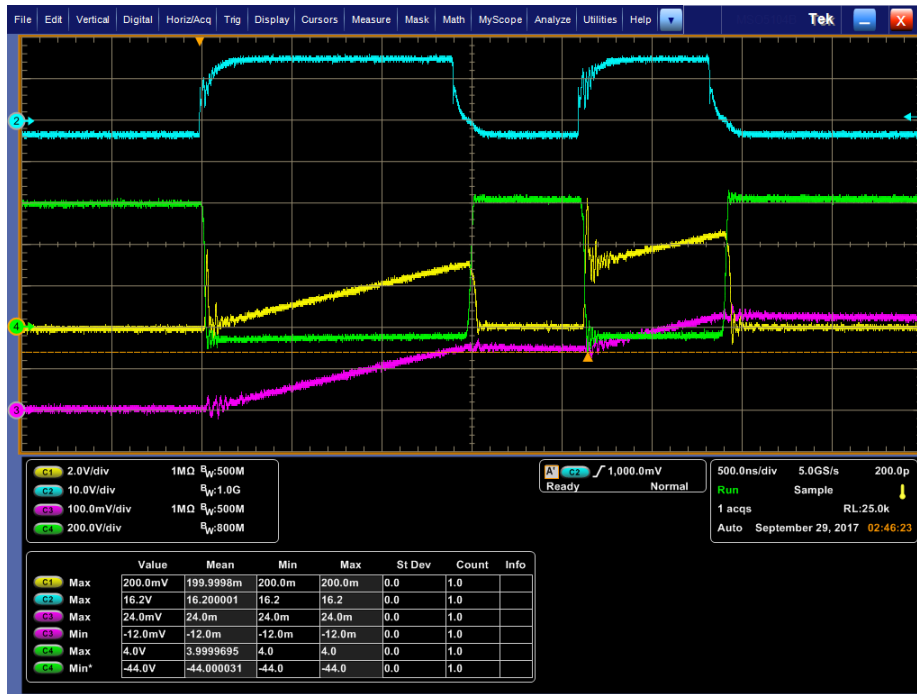
Figure 4.19. DPT waveforms for X3M0016120K with 3\Omega external gate resistance and 600 V DC bus for (1) I_{D, BOT} (10 A/div), (2) V_{GS, BOT} , (3) I_L (10 A/div), and (4) V_{DS, BOT} .
