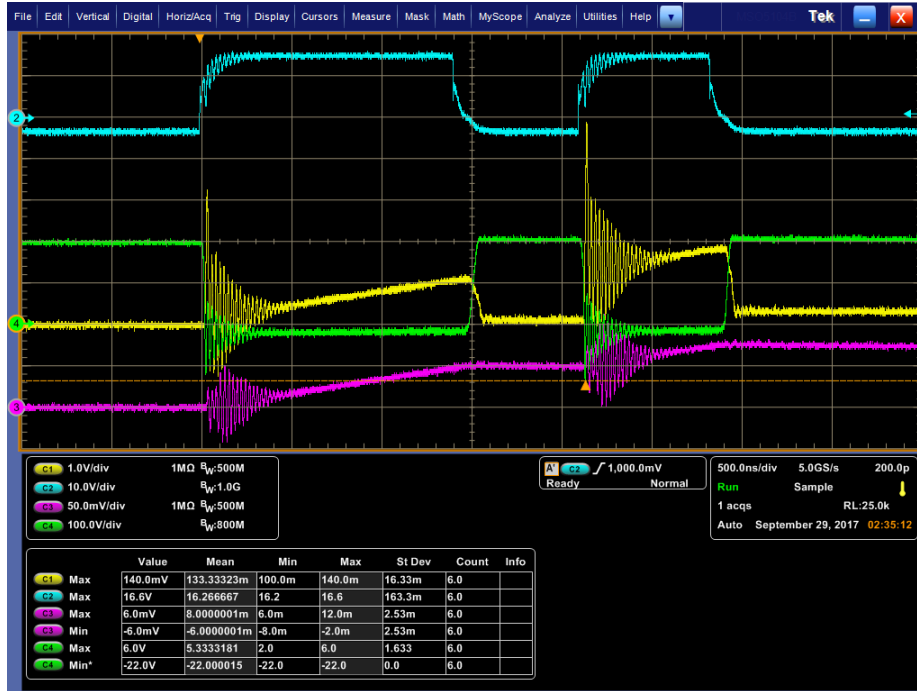
Figure 4.17. DPT waveforms for X3M0016120K with 3\Omega external gate resistance and 200 V DC bus for (1) I_{D, BOT} (5 A/div), (2) V_{GS, BOT} , (3) I_L (5 A/div), and (4) V_{DS, BOT} .
