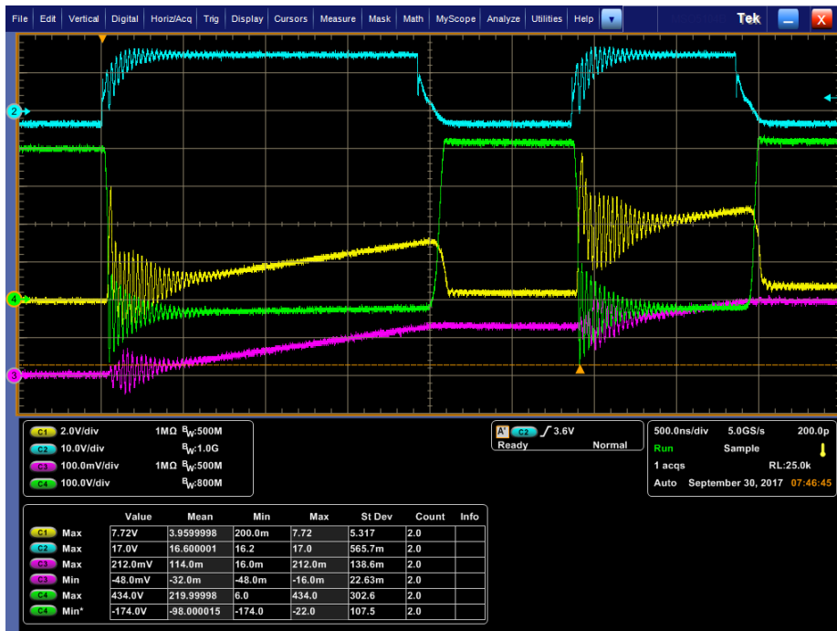
Figure 4.12. DPT waveforms for C3M0010090K with 4\Omega external gate resistance and 400 V DC bus for (1) I_{D, BOT} (10 A/div), (2) V_{GS, BOT} , (3) I_L (10 A/div), and (4) V_{DS, BOT} .
