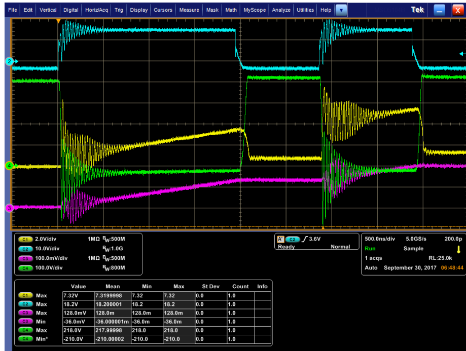
Figure 4.6. DPT waveforms for C3M0010090K with 1.5\Omega external gate resistance and 400 V DC bus for (1) I_{D, BOT} (10 A/div), (2) V_{GS, BOT} , (3) I_L (10 A/div), and (4) V_{DS, BOT} .
