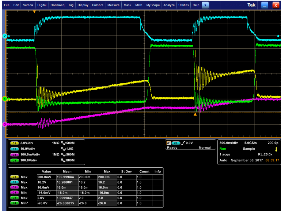
Figure 4.15. DPT waveforms for C3M0010090K with 6\Omega external gate resistance and 400 V DC bus for (1) I_{D, BOT} (10 A/div), (2) V_{GS, BOT} , (3) I_L (10 A/div), and (4) V_{DS, BOT} .
