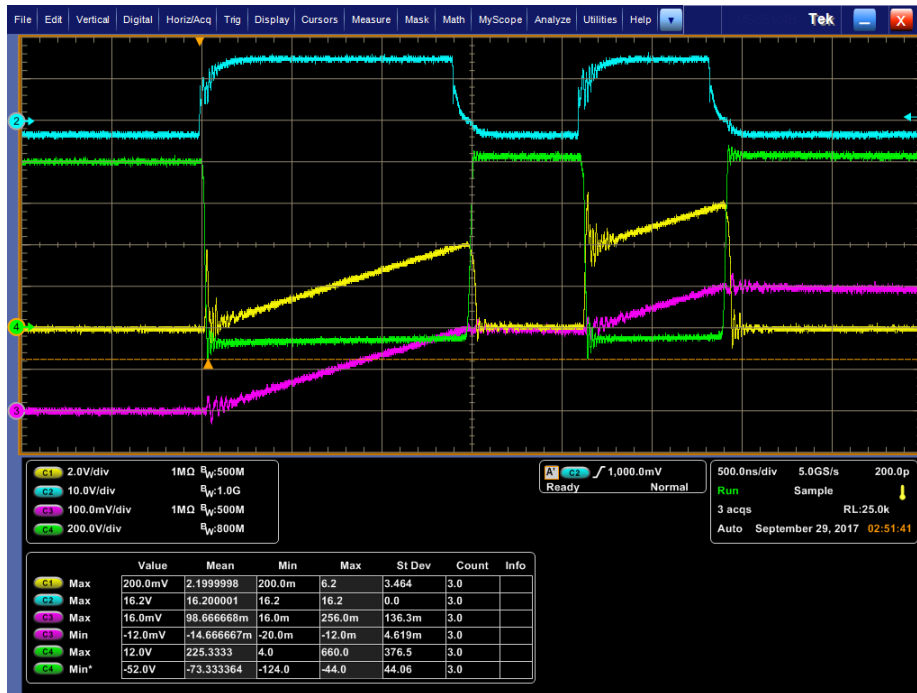
Figure 4.20. DPT waveforms for X3M0016120K with 3\Omega external gate resistance and 800 V DC bus for (1) I_{D, BOT} (10 A/div), (2) V_{GS, BOT} , (3) I_L (10 A/div), and (4) V_{DS, BOT} .
