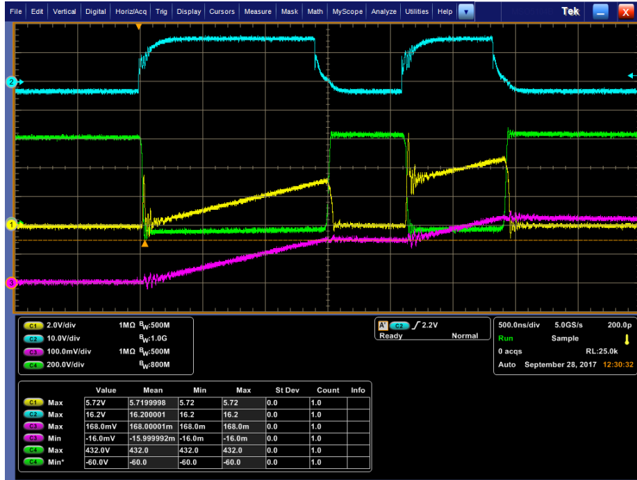
Figure 4.23. DPT waveforms for X3M0016120K with 4\Omega external gate resistance and 600 V DC bus for (1) I_{D, BOT} (10 A/div), (2) V_{GS, BOT} , (3) I_L (10 A/div), and (4) V_{DS, BOT} .
