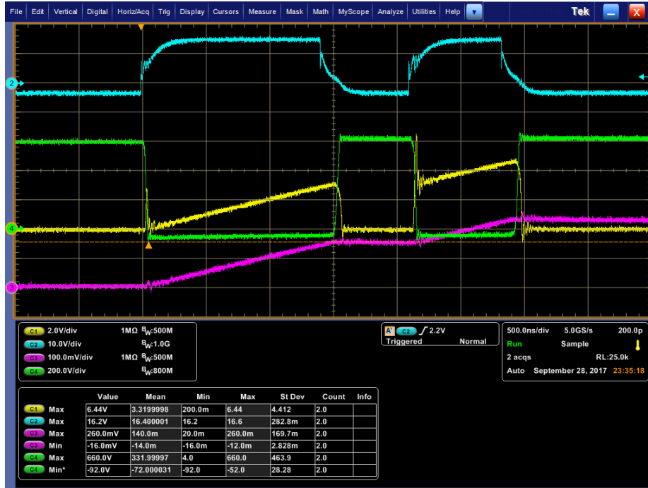
Figure 4.27. DPT waveforms for X3M0016120K with 6\Omega external gate resistance and 600 V DC bus for (1) I_{D, BOT} (10 A/div), (2) V_{GS, BOT} , (3) I_L (10 A/div), and (4) V_{DS, BOT} .
