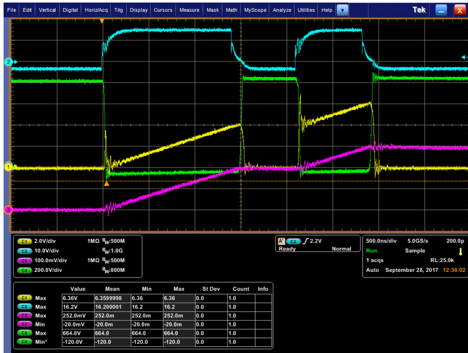
Figure 4.24. DPT waveforms for X3M0016120K with 4\Omega external gate resistance and 800 V DC bus for (1) I_{D, BOT} (10 A/div), (2) V_{GS, BOT} , (3) I_L (10 A/div), and (4) V_{DS, BOT} .
