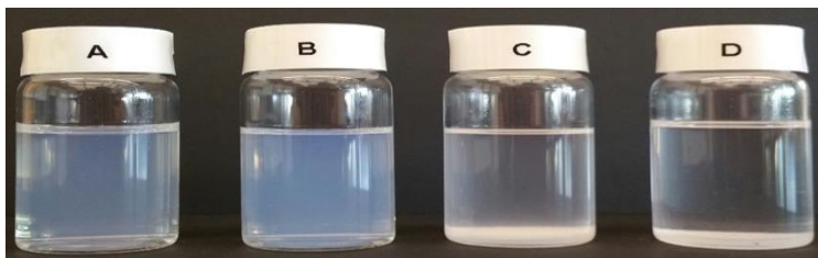
Figure 5a. Dispersion state of 0.1 % (W/V) of \text{TiO}_2 in water suspension (A), \text{TiO}_2 in methanol suspension (B), \text{TiO}_2 in chloroform suspension (C) and \text{TiO}_2 in toluene suspension (D) after one day.
