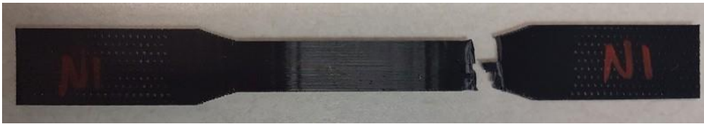
Figure 73. Front View of Coupon with 3 Contours Failure. Delamination occurred due to the lack of raster fill in the gage section.
