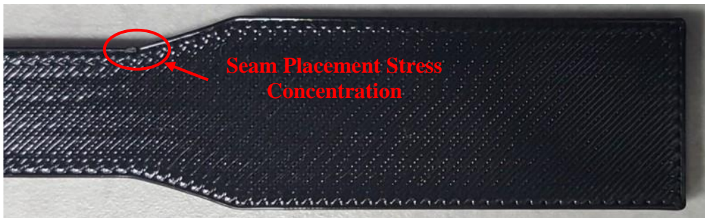
Figure 68. Stress Concentration Due to Seam Place on Test Coupon. The contour seam placement is at the same location between each layer on the test coupon.
