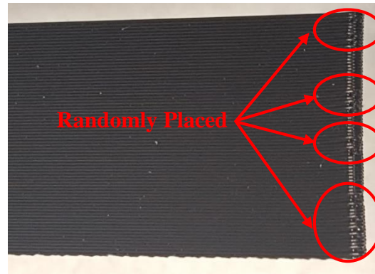
Figure 70. Randomly Placed Seams on Test Coupon. Stratasys Insight Revision software was used to specify random seam placement between each layer.
