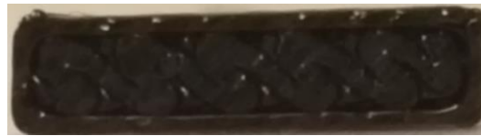
Figure 41. Rectangular Bar Raster Thickness 0.024 in. The interior of the rectangular bar was filled with a raster thickness of 0.024 in.
