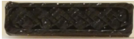
Figure 40. Rectangular Bar Raster Thickness 0.018 in. The interior of the rectangular bar was filled with a raster thickness of 0.018 in.
