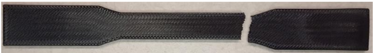
Figure 69. Failure Outside of the Test Region Due to Seam Placement. The crack propagated from the seam into the shoulder of ASTM D638 Type I geometry. The failure did not occur purely in the gage section. Therefore, the data for the coupons with the seam placement at the shoulder is invalid.
