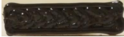
Figure 40. Rectangular Bar Raster Thickness 0.018 in. The interior of the rectangular bar was filled with a raster thickness of 0.018 in.
