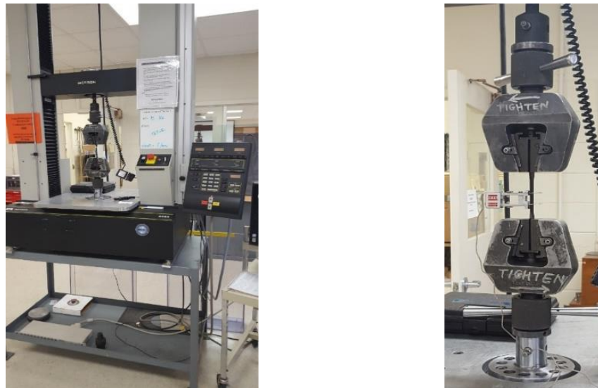
Figure 8. Experimental Setup for Static Testing. A 5 kN Instron 4468 load frame was used to conduct the static tests for ULTEM 9085 coupons. A MTS 634.12E-54 extensometer was used to measure the strain of the gage section as shown in right picture.
