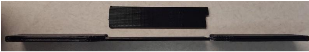
Figure 75. Front View of Coupon with 2 Contours and a Contour Thickness of 0.030 in. Failure. The force shockwave from the sudden failure propagated up the gage section and completely delaminated the contour in the gage section. The gage section has two contour deposited side by side without a raster fill.
