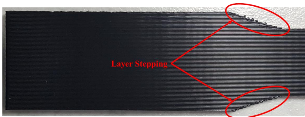
Figure 64. Layer Stepping Due to Discretization of Radius. The layer stepping on the radiuses of the coupon creates a stress concentration.
