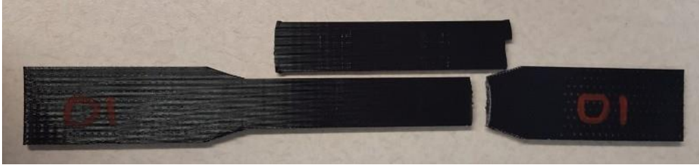
Figure 75. Front View of Coupon with 2 Contours and a Contour Thickness of 0.030 in. Failure. The force shockwave from the sudden failure propagated up the gage section and completely delaminated the contour in the gage section. The gage section has two contour deposited side by side without a raster fill.
