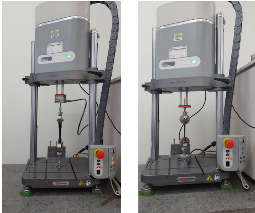
Figure 16. Reconfigured E1000 Fatigue Testing Machine. The picture to the left shows the E1000 in the original configuration with the load cell at the top. The picture to the right shows E1000 with the shortened coupon, shortened grip's mounting rod, and the load cell was moved to the bottom of the machine.
