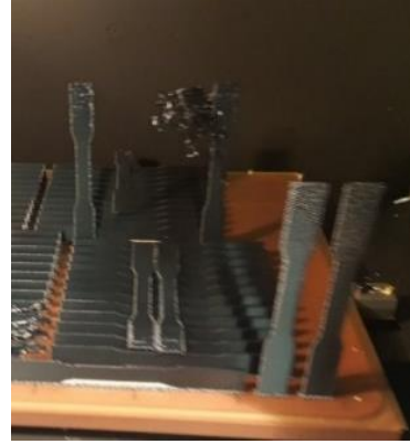
Figure 78. ASTM D638 Type I Build Orientation ZXY Failed Print. The failed printed was caused by the tall aspect ratio of the geometry. The cantilever beam effect caused the specimen to oscillate. The vibration prevented the layers from being deposit correctly.
