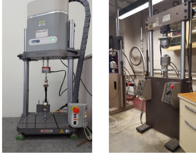
Figure 10. Fatigue Testing Experimental Setup. The ElectroPuls E1000 on the left was used for stress levels less than 50% of ultimate tensile stress. The MTS 810 on the right was used for stress levels greater than 50% of the ultimate tensile stress.
