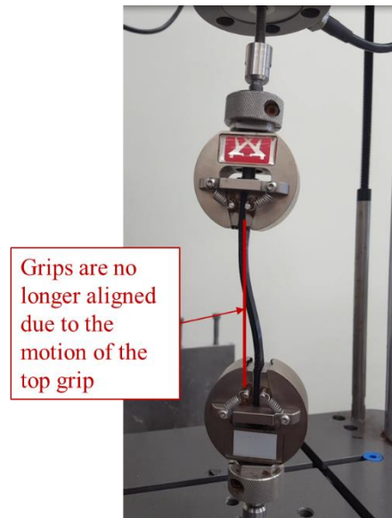
Figure 14. Translating Grip on the E1000. The top grip's mounting shaft does not have enough stiffness to support the compressive load. The bending of the mounting shaft applied a lateral load to the specimen causing it to buckle.
