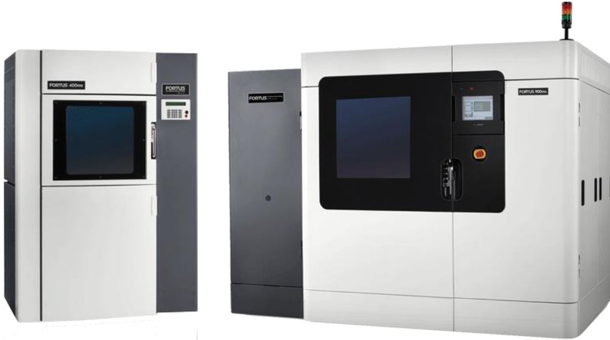
Figure 4. Comparison between Fortus 400MC and Fortus 900MC. Both the Fortus 400MC and the Fortus 900MC are very similar except for the build volumes. The Fortus 400MC has a build envelope of 16 in. x 14 in. x 16 in. and the Fortus 900MC has a build envelope of 36 in. x 24 in. x 36 in. The image above was obtained from Metalworking World Magazine. 3 , 9
