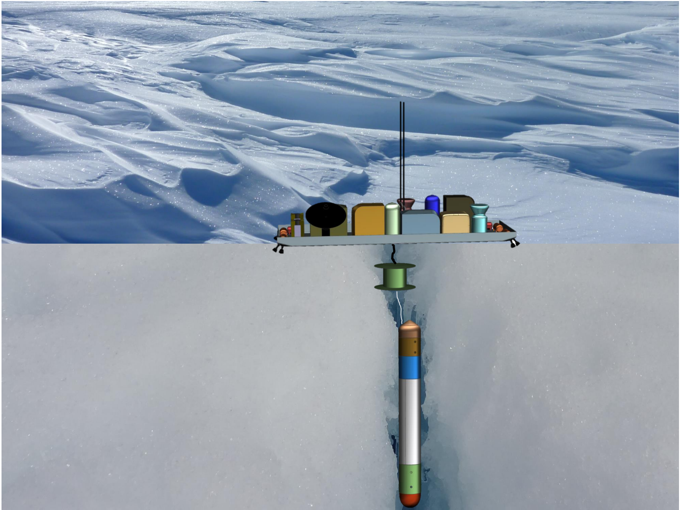
Figure 9.7: Cryobot and surface unit shortly after the descent of the cryobot begins. Background images from http://breconbeacons.files.wordpress.com/2012/01/felicity-in-antarctica.jpg and http://www.polarfield.com/blog/wp-content/uploads/2012/12/DSC00207.jpg .
