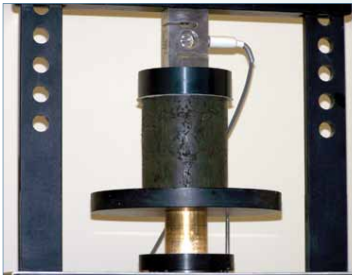
A compression test is administered on an organic soil sample. Results of the tests proved soils with organic content in excess of nine percent are suitable for stability berm fill.
