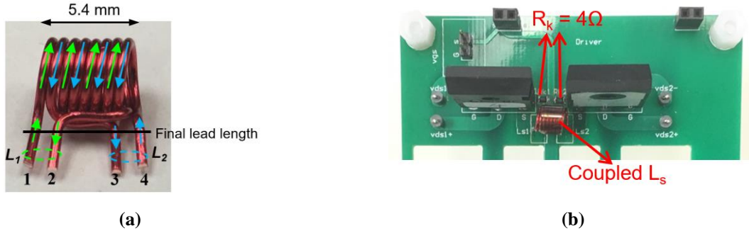
Fig. 3-15. (a) Fabricated coupled inductors, and (b) photo of hardware with designed coupled power-source inductors and resistors inserted.
