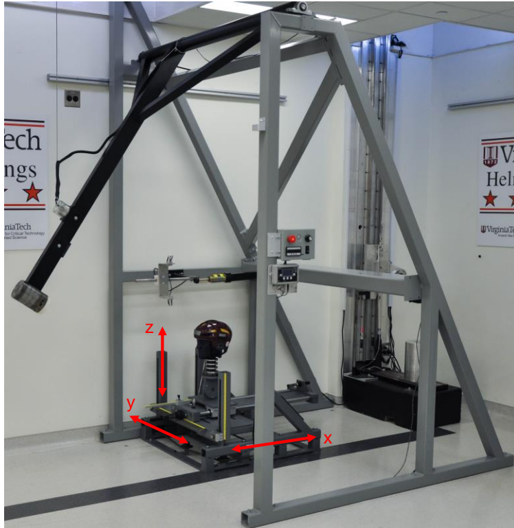
Figure 8: The custom impact pendulum device was used to strike a NOCSAE headform mounted on a Hybrid III 50 th percentile neck. The head and neck were mounted on a sliding mass that simulates the effective mass of the torso during impact. The slide table had 5 degrees of freedom so that any location on the helmet could be impacted: translation along the x axis, translation along the y axis, translation along the z axis, rotation about the y axis, and rotation about the z axis.
