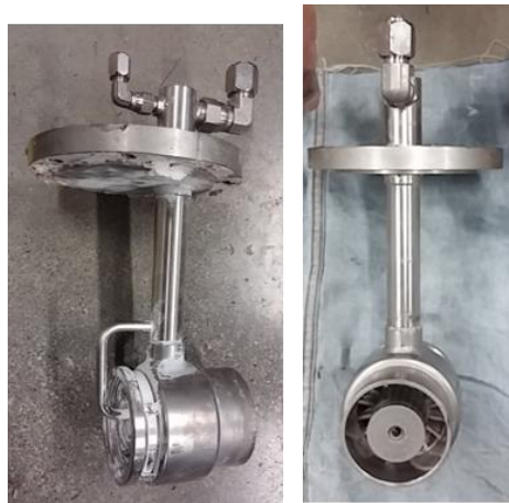
Figure 15. Swirl fuel nozzle (SoLoNOx) designed by Solar Turbines Inc.
