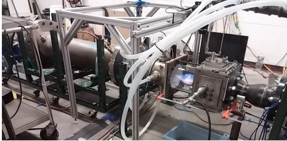
Figure 9. Photograph of the optical combustor rig with a pilot flame inside.
