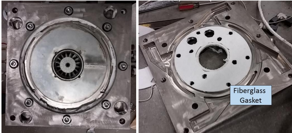
Figure 13. Photograph of dome plate installed on the settling chamber.
