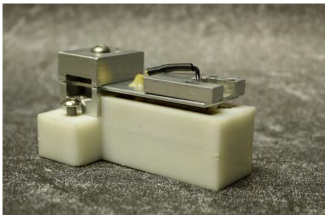
Figure 2: Electromagnetic vibration energy harvester being developed for Pratt & Whitney.
