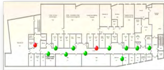
Figure 1: Radio node locations in each floor of the ICTAS building.
