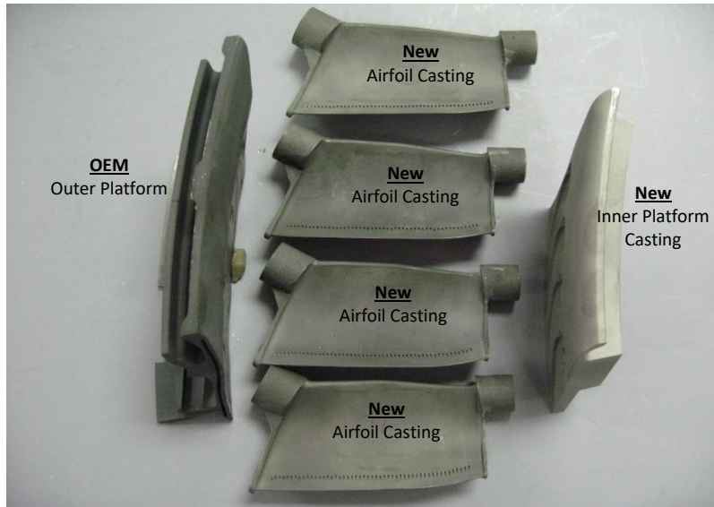
Figure 3: Representative repaired vane
