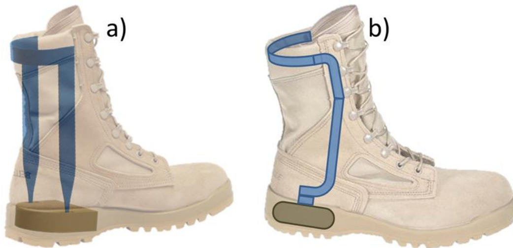
Figure 3.36 – Concept renderings of torque input, with a) simple straight lever, and b) more ergonomic curved lever to avoid tibia and fibula heads.
