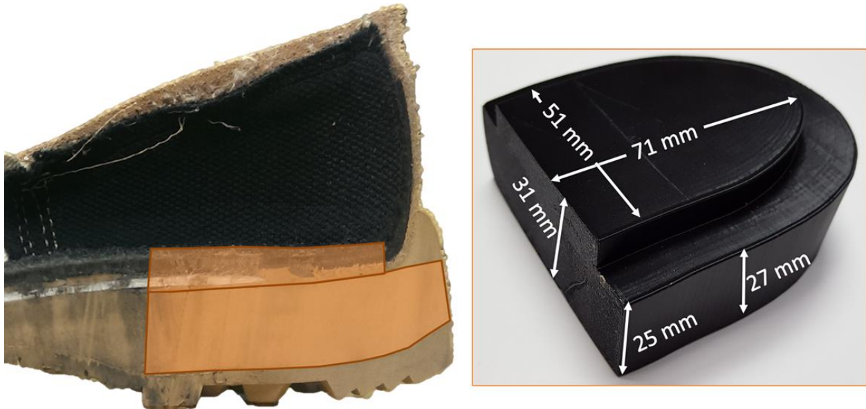
Figure 3.33 – Housing Generation 3: (Left) Cross-section of Belleville 390 hot weather combat boot with overlay of cross-section of device housing size and locations, (Right) picture of 3D printed housing prototype with overlaid dimensions.
