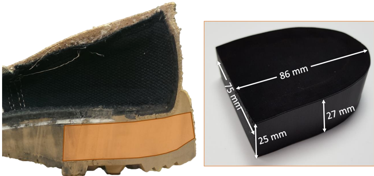
Figure 3.32 – Housing Generation 2: (Left) Cross-section of Belleville 390 hot weather combat boot with overlay of cross-section of device housing size and locations, (Right) picture of 3D printed housing prototype with overlaid dimensions.
