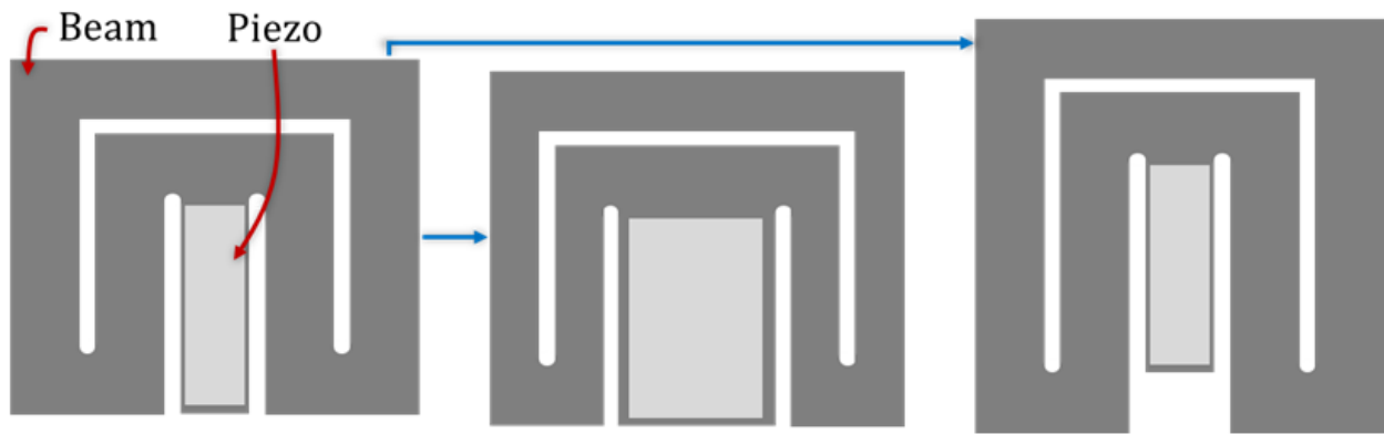
Figure 5.3 – Illustration of possible geometry improvements to the ‘Elephant’ piezoelectric vibration energy harvester.
