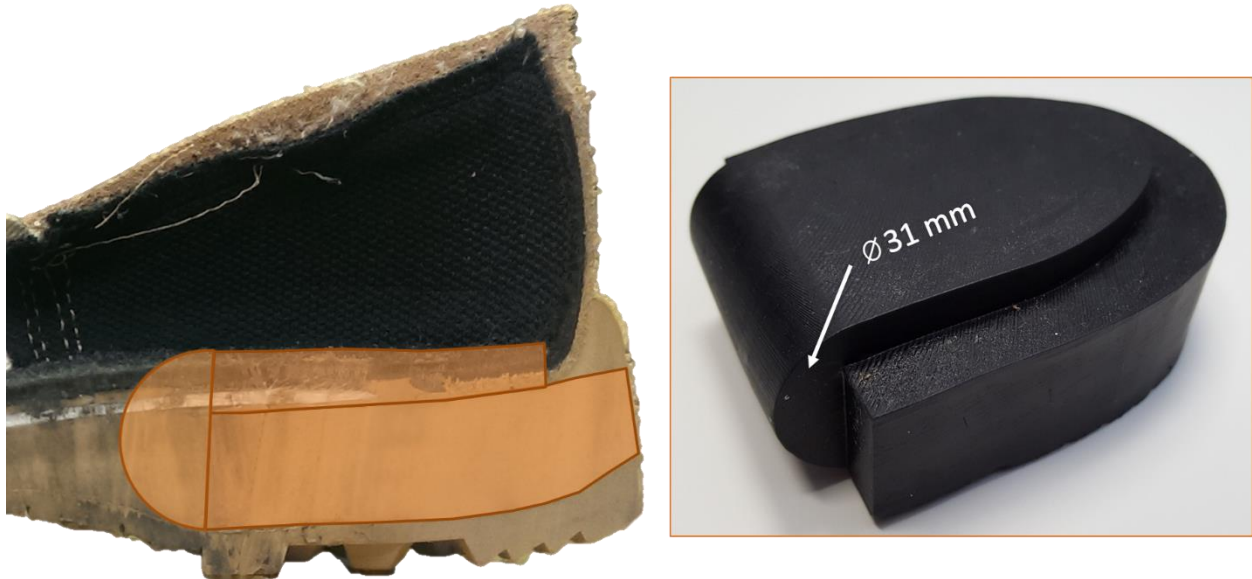
Figure 3.34 – Housing Generation 4: (Left) Cross-section of Belleville 390 hot weather combat boot with overlay of cross-section of device housing size and locations, (Right) picture of 3D printed housing prototype with overlaid dimensions.
