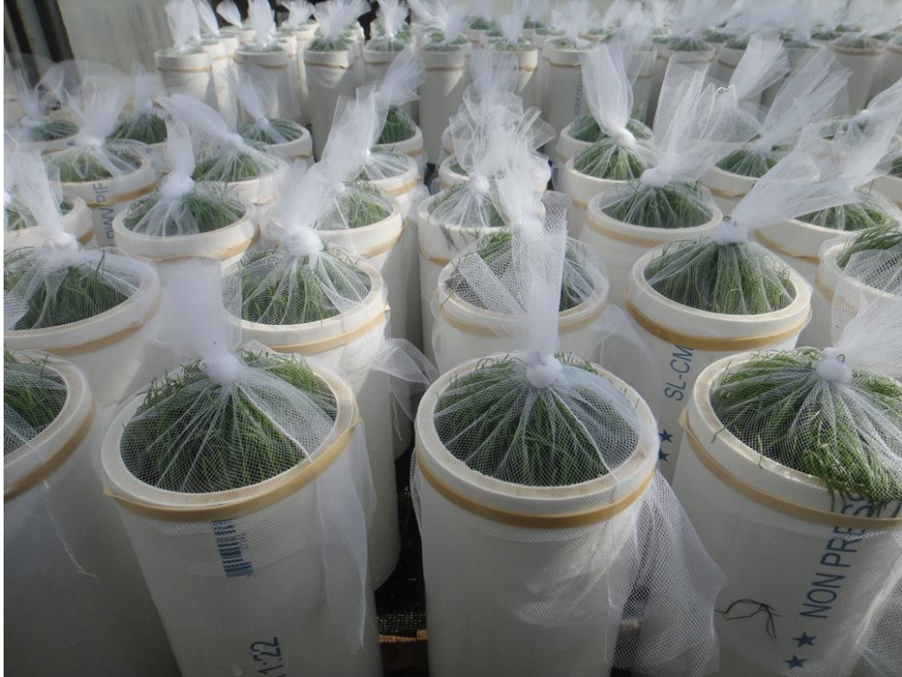
Fig. 3.1. Oviposition arena with treated soil and caged Popillia japonica females.
