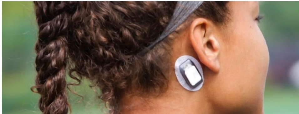
Figure 1. A head impact sensor containing three linear accelerometers and three angular rate sensors placed behind the ear of a player
