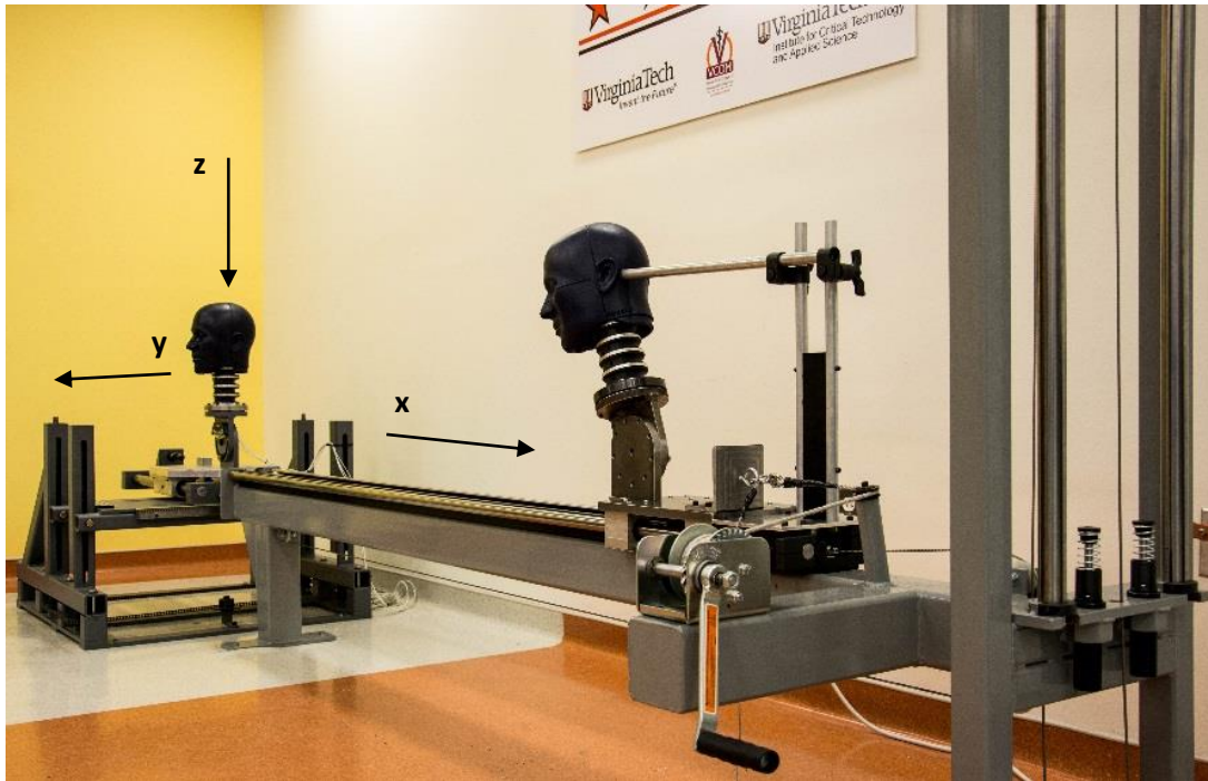
Figure 2. A custom impactor was designed and built to simulate head-to-head impacts in soccer. The system consists of two head and neck assemblies mounted onto sliding masses which are free to translate. One sliding mass is accelerated to a target velocity and impacts another, stationary sliding mass with free travel. The impacted mass is instrumented to measure impact kinematics.
