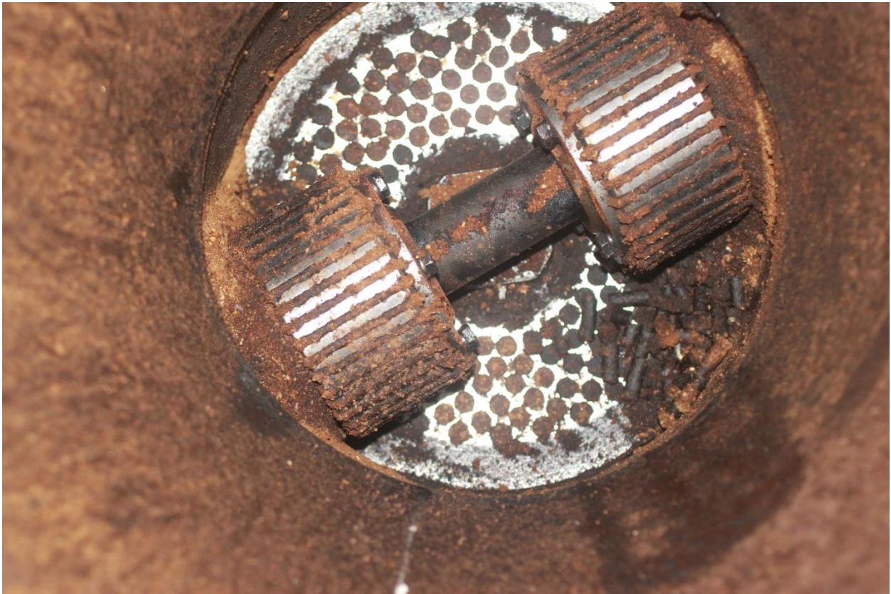
Figure 4.3. The inside of the PTO powered flat die pellet mill. The flat die plate in the bottom rotates against both rollers to create friction and heat. The rollers also force the ground material through the holes in order to create the cylindrical biomass pellets.
