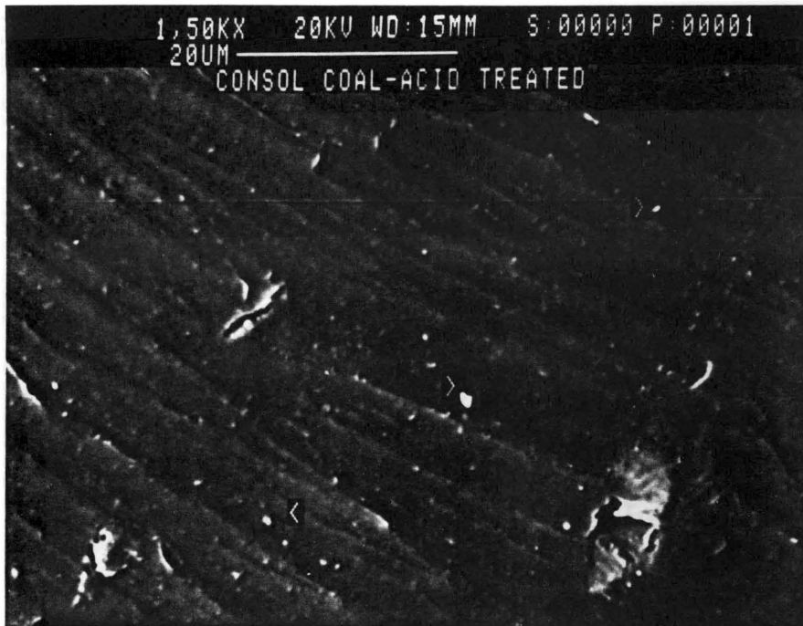
Figure 19. Photomicrographs of Consol Coal: (Top) Feed coal -140 + 270 mesh. (Bottom) Acid treated Consol coal
