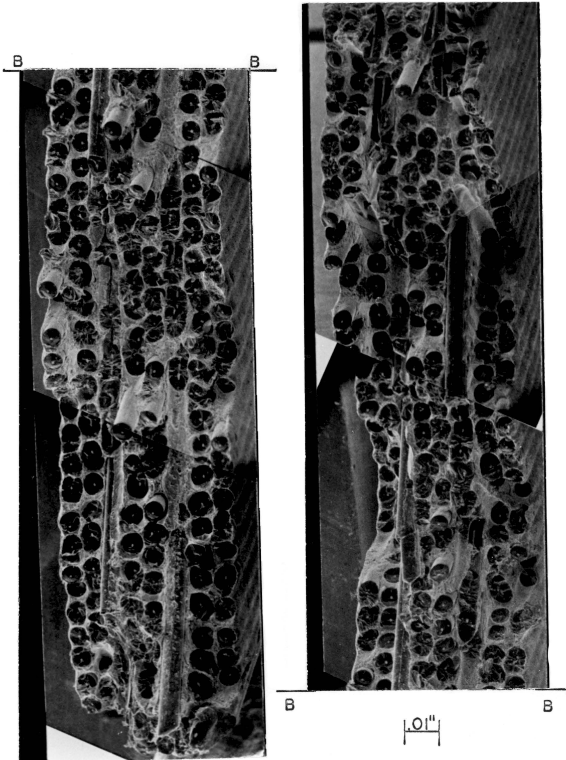
Figure 14. B/A1 Ib static fracture surface.
