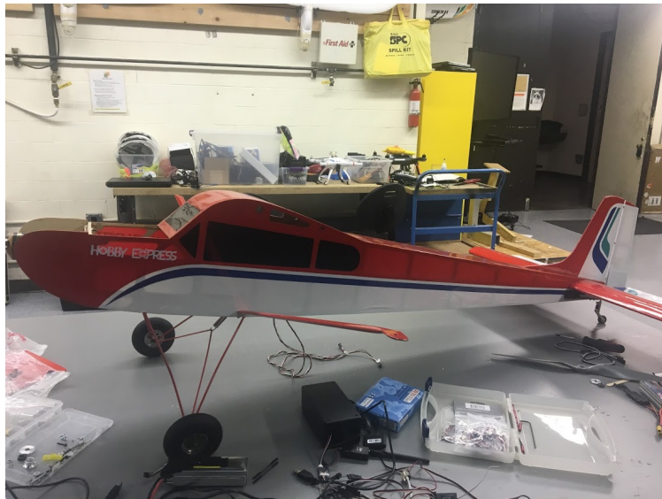
Figure 5.22: Fixed wing aircraft assembled for running flight tests with OcPoC as the flight controller hardware
