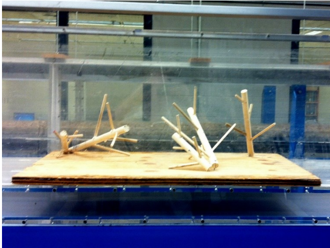
Figure 4.2 – Model woody debris field used to evaluate sensor uncertainty with obstructions in storm sewer channels
