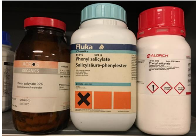
Figure 4-2. Bonding material for sapphire fiber pigtail
